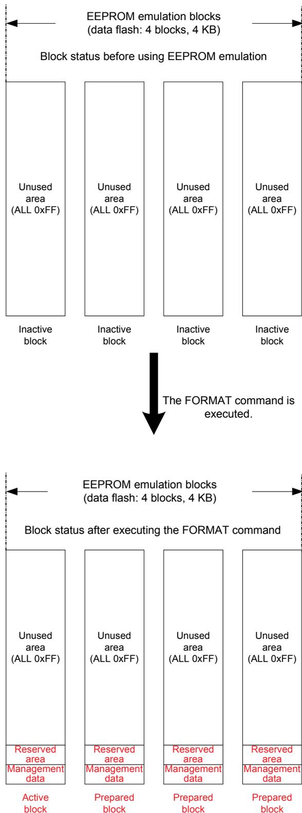
Figure 1-16. Flow when Performing Initialization at Arbitrary Time (when Using Enforced Mode)
