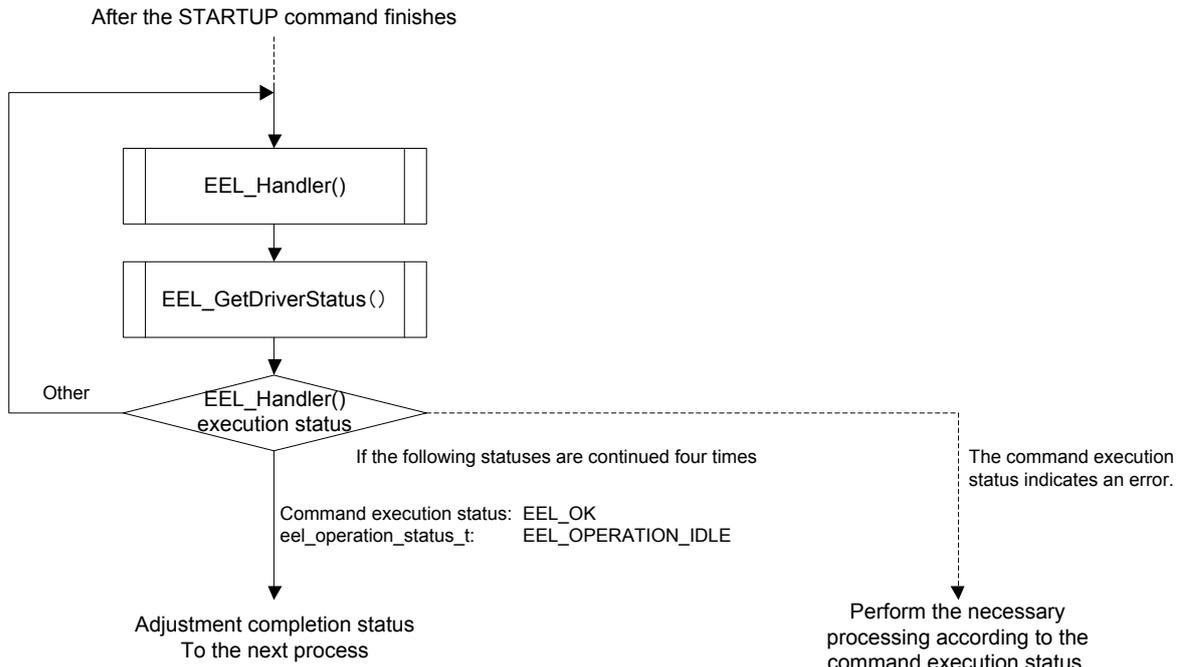
Figure 1-24. Execution Flow when Performing Adjustment after Executing the EEL\_CMD\_WRITE Command (Adjustment Completion Status)
