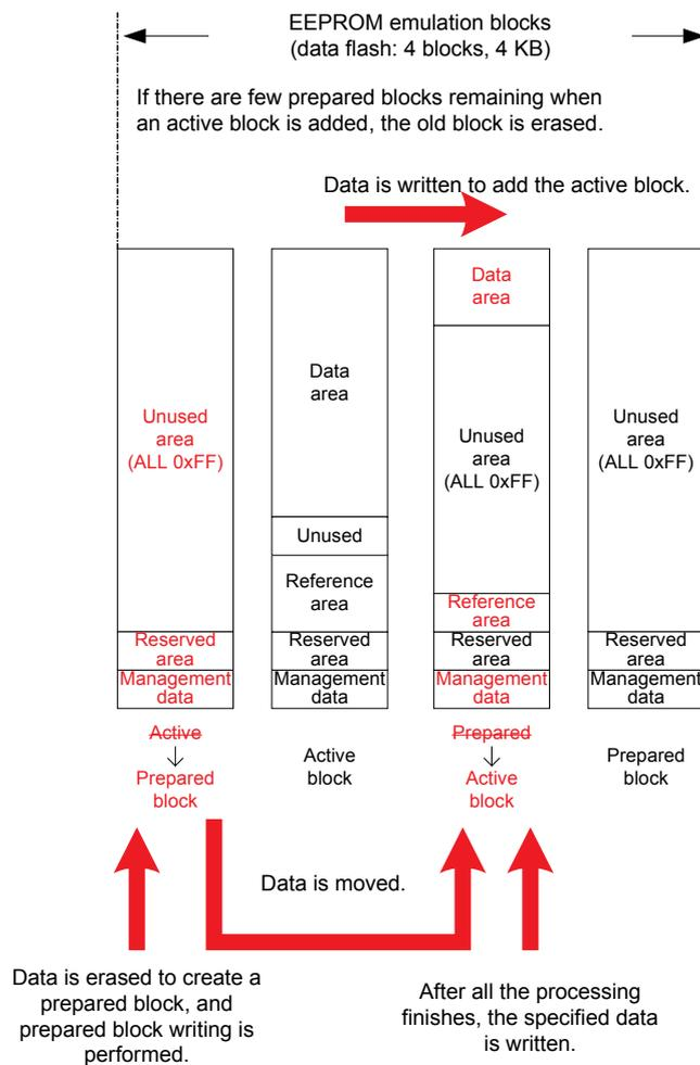
**Figure 1-19. Changes in Processing Time according to Block Status when Writing Data (when Using Enforced Mode)**
