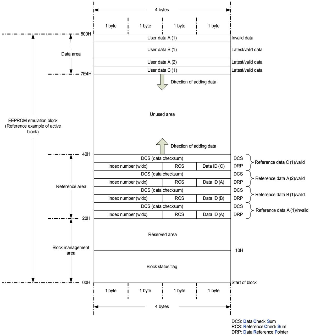
**Figure 1-4. Example of Expanding Active EEPROM Emulation Block**
