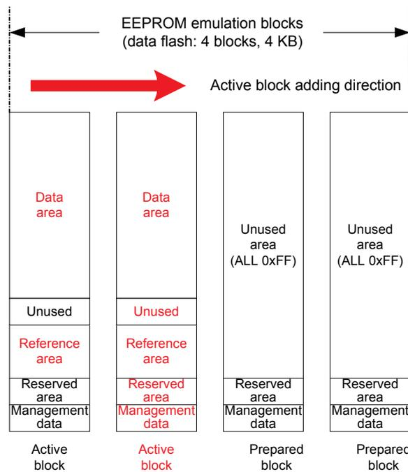
Figure 1-6 (C). EEPROM Emulation Block Transition Example
