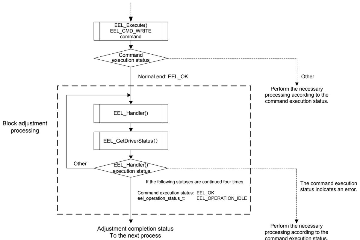
Figure 1-25. Execution Flow when Performing Adjustment upon Starting EEPROM Emulation (Adjustment Completion Status)
