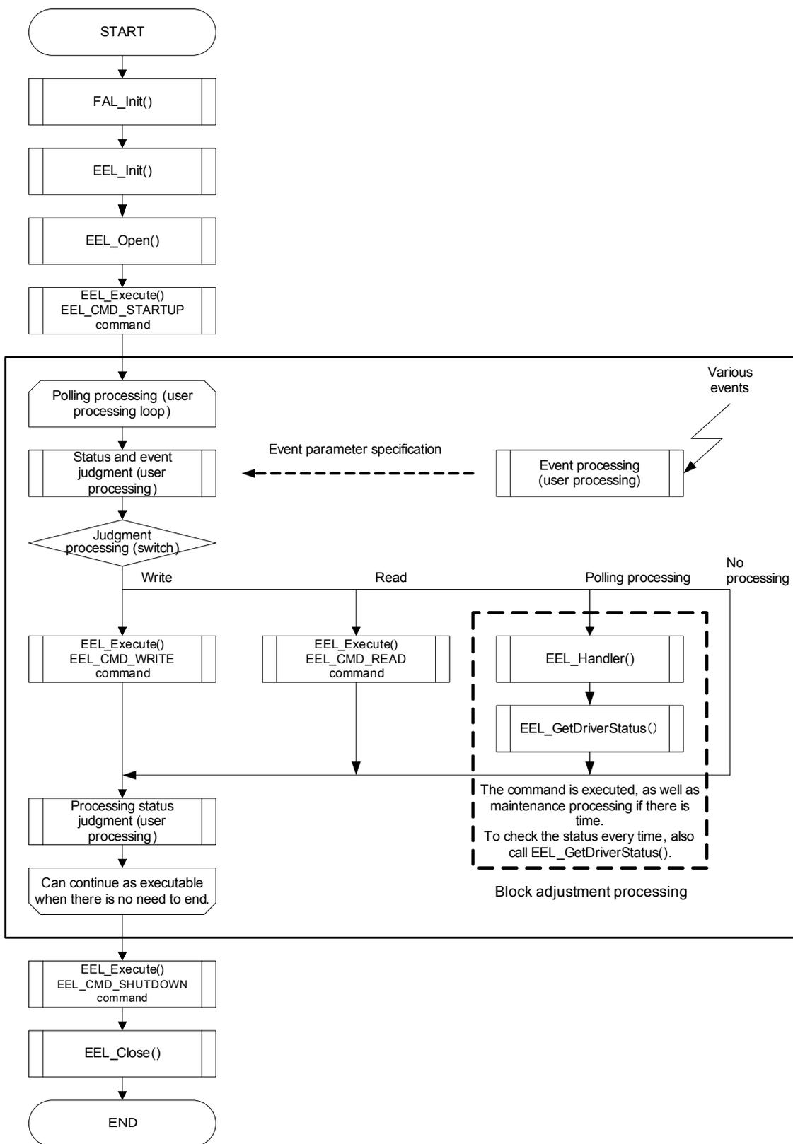
Figure 1-27. Example of Block Adjustment in EEL\_Handler Function Maintenance Mode (Adjustment Completion Status)
