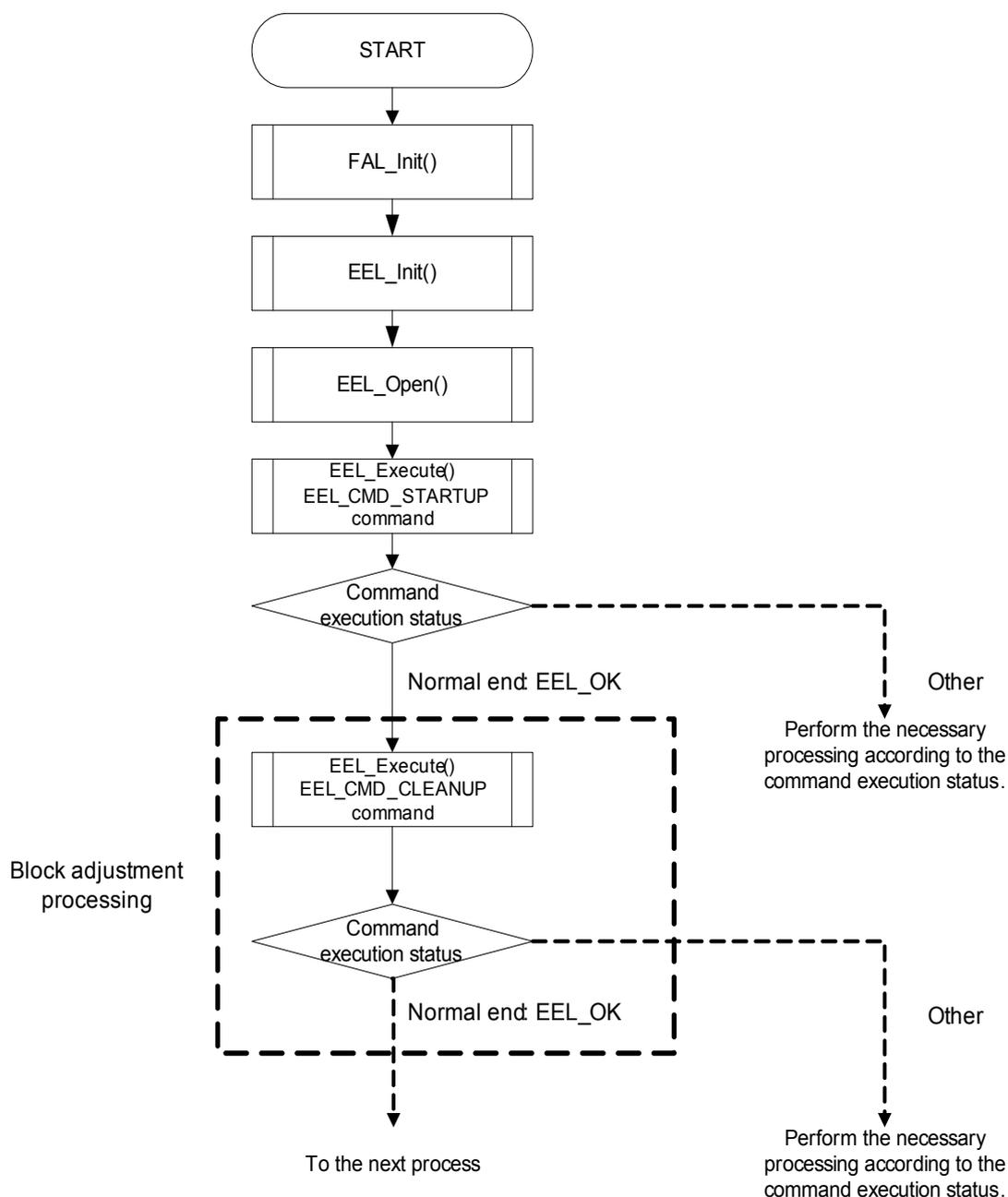
Figure 1-21. Adjusting Blocks by Using the EEL\_CMD\_CLEANUP Command
