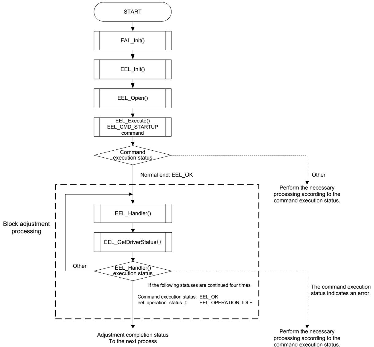
Figure 1-26. Example Flow for Executing Command and Maintenance Mode Processing in Polling Mode
