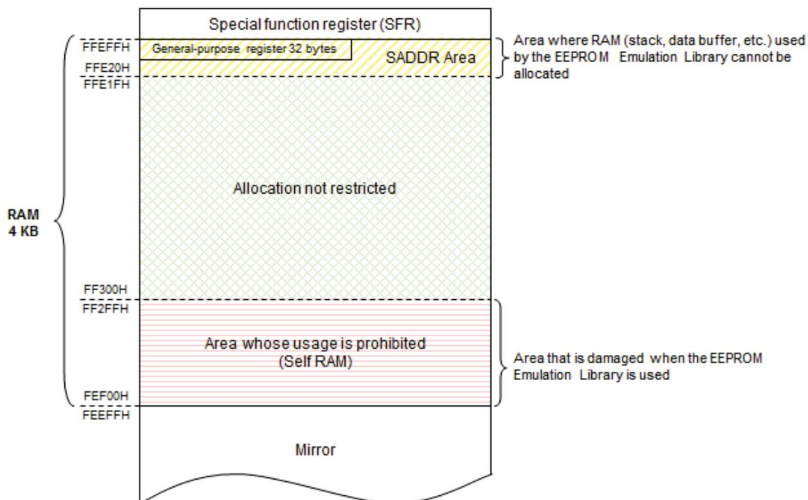
Figure 2-3 Example 2 of RAM Allocation without Self-RAM
