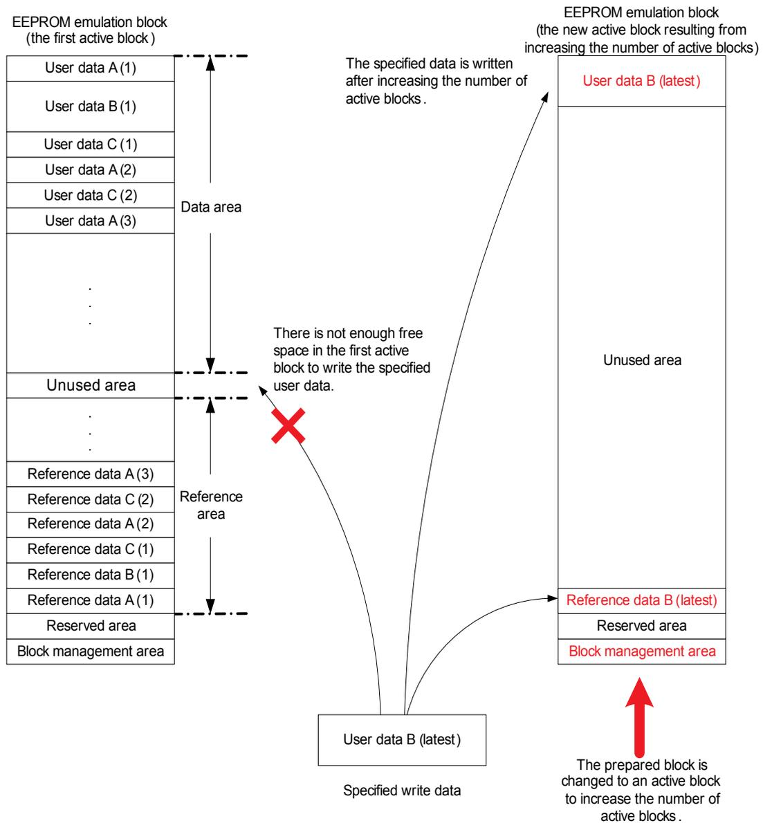
**Figure 1-5. EEPROM Emulation Block Usage Method (Four Blocks)**
