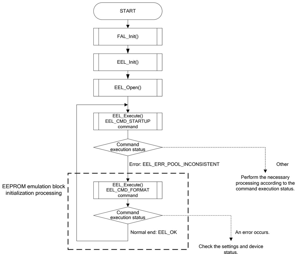
Figure 1-15. Example Block Status Transitions when Initialization is Performed upon Occurrence of EEL\_ERR\_POOL\_INCONSISTENT Error
