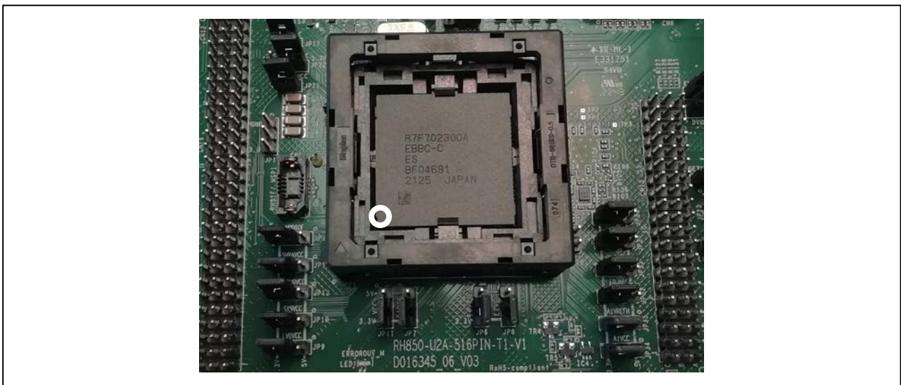
Figure 1.13 Enplas OTP-516(961RS)-0.8-048S-00 socket with mounted device
