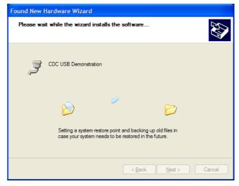
An additional COM port will become available to Window Applications. To be able to see the port that has been allocated you can open the Windows Device Manager window. To do this, go to the start menu and select run. In the dialog displayed type "devmgmt.msc". This will open the device manager. Expand the group of serial ports and the installed ports will be listed. When the Serial Terminal program connects to this COM port", it will receive a repeating message from the RSK saying:
