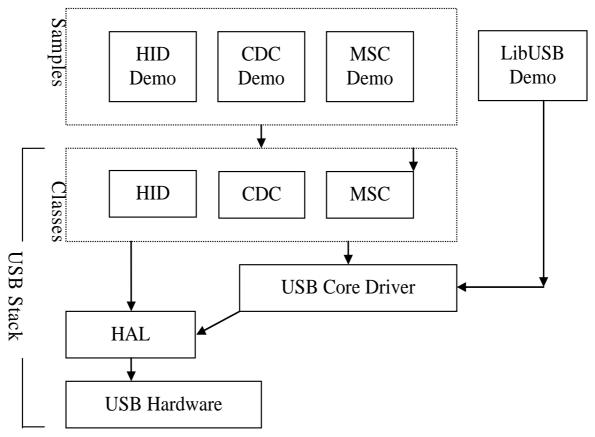
Figure 1 – Embedded SW, including Layers of USB Stack
