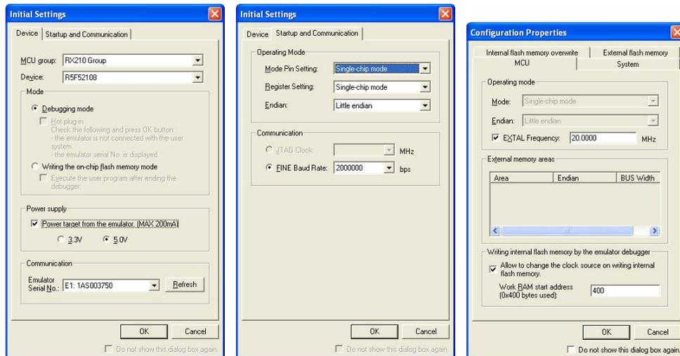
35. The flash memory write program is then downloaded to the microcontroller. The Output window in HEW will state 'Connected'.
