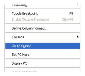
The code will run to the selected line and stop. A temporary breakpoint was automatically inserted in the code and then removed when the program stopped at the breakpoint.
