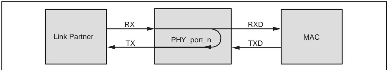
Figure 2.3 Far-End Loopback Diagram
