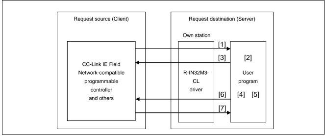
Figure 5.6 Transient2 Request Reception Procedure
