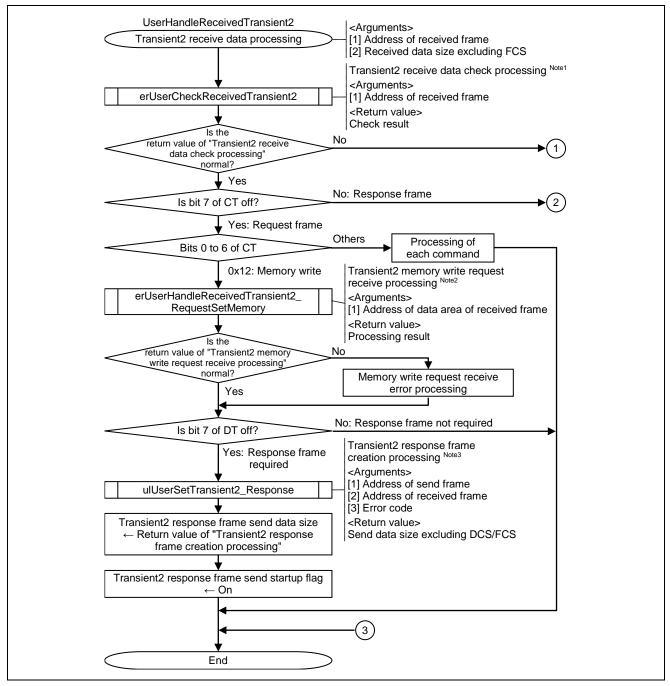
Figure 6.35 Flowchart for Transient2 Receive Data Processing (1/2)
