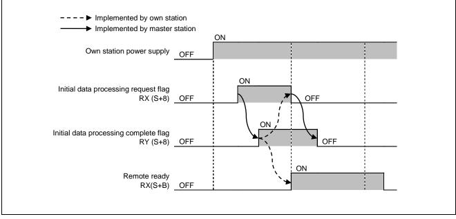
Figure 7.2 Timing Chart: Initial Data Processing Request/Complete Flag
