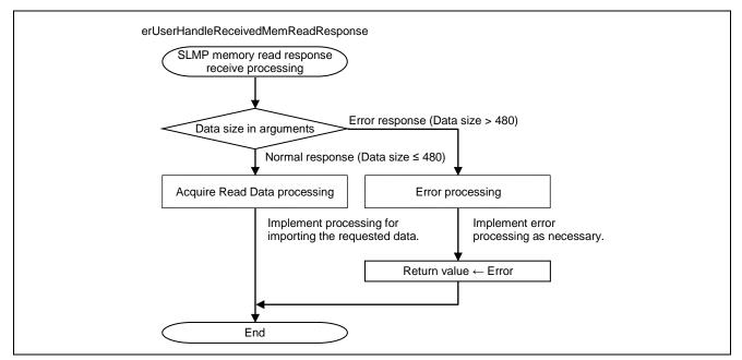
Figure 6.48 Flowchart for SLMP Memory Read Response Receive Processing
