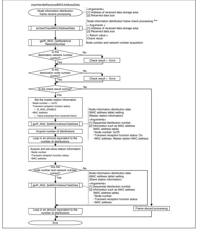
Figure 6.25 Flowchart for Node Information Distribution Frame Receive Processing
