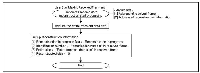
Figure 6.23 Flowchart for Transient1 Receive Data Reconstruction Start Processing
