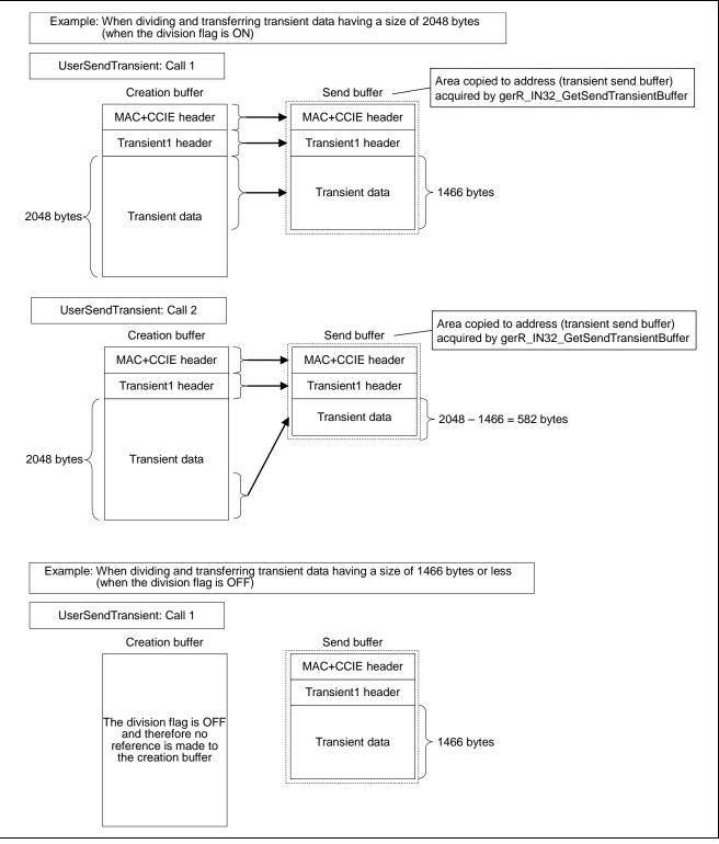
Figure 6.20 Transient Frame Divided Sending Procedure
