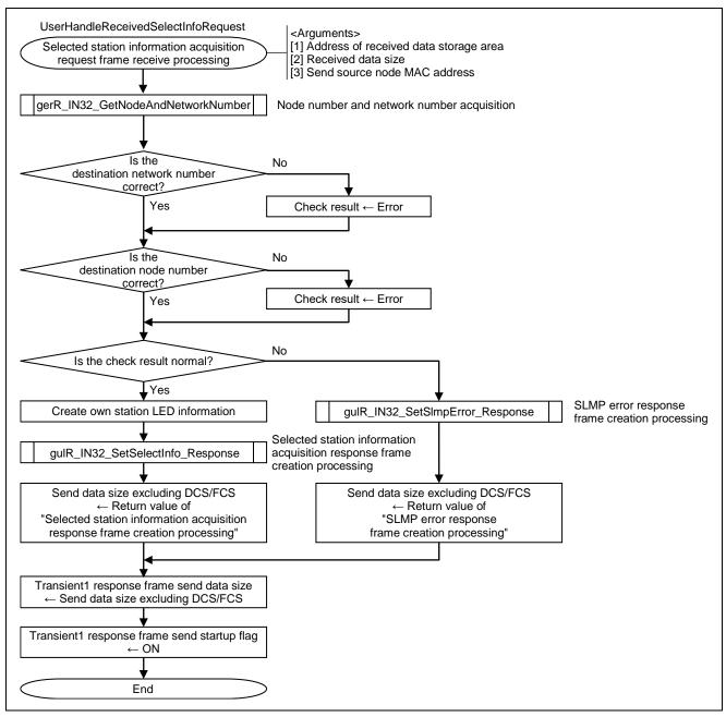
Figure 6.32 Flowchart for Selected Station Information Acquisition Request Frame Receive Processing
