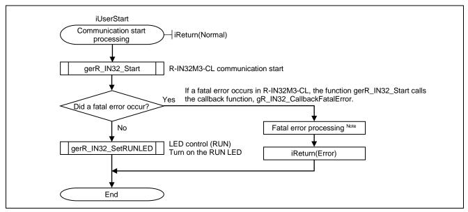
Figure 6.5 Flowchart for Communication Start Processing
