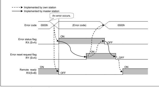
Figure 7.5 Timing Chart: Error Status Flag, Error Reset Request Flag
