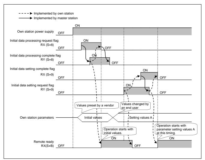
Figure 7.4 Timing Chart: Initial Data Processing and Setting
