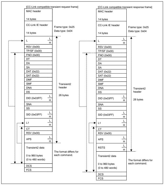
Figure 5.21 Overview of CC-Link Compatible Transient Frame Format
