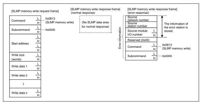
Figure 5.32 SLMP Memory Write Frame
