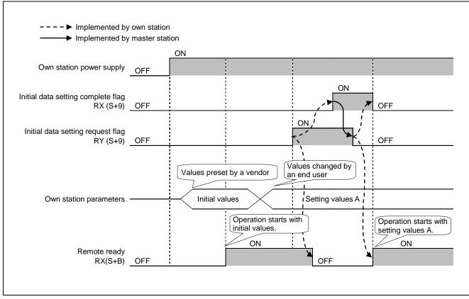
Figure 7.3 Timing Chart: Initial Data Setting Complete/Request Flag
