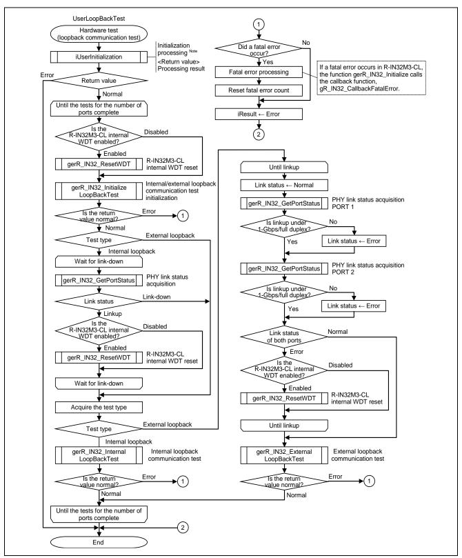
Figure 6.51 Flowchart for Hardware Test (Loopback Communication Test)
