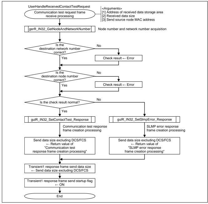
Figure 6.33 Flowchart for Communication Test Request Frame Receive Processing
