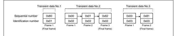
Figure 5.11 Transient1 Header: Relationship Between Sequential Number and Identification Number of Transient Data
