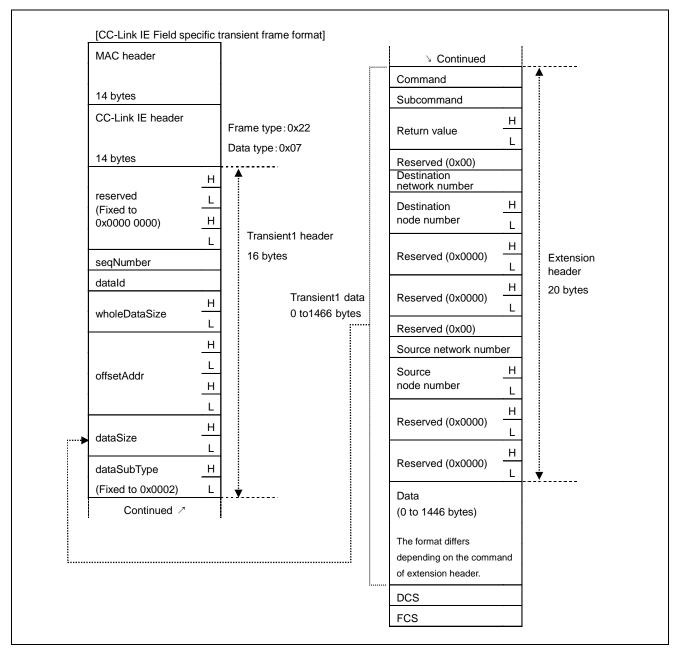
Figure 5.10 Overview of CC-Link IE Field Specific Transient Frame Format
