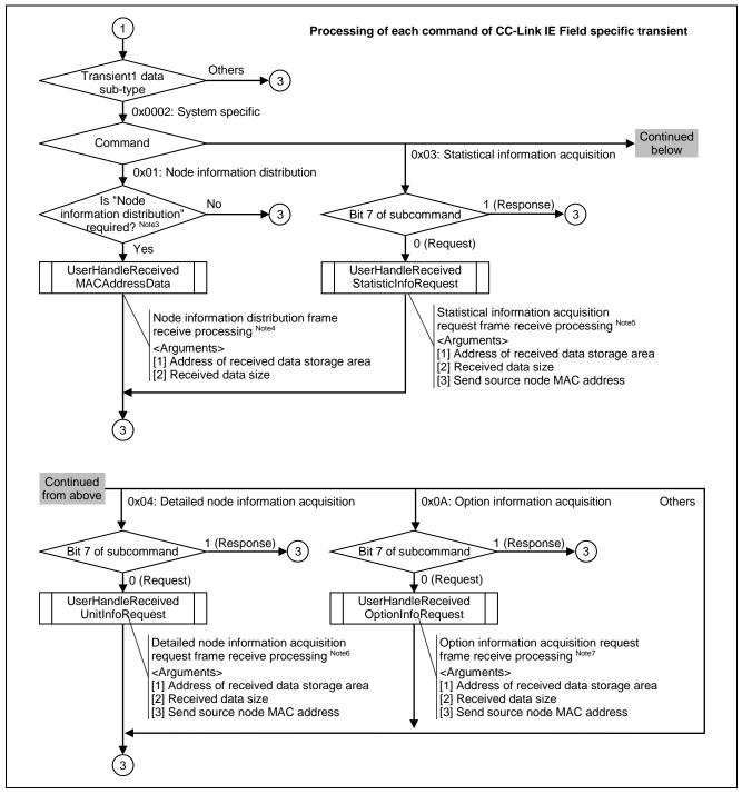
Figure 6.21 Flowchart for Transient1 Receive Data Processing (2/3)
