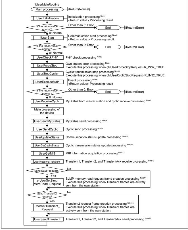
Figure 6.3 Flowchart for Main Processing
