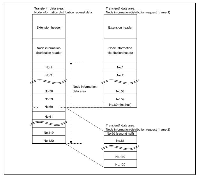
Figure 5.12 Transient1 Data Area: Divided Frames at Node Information Distribution Request
