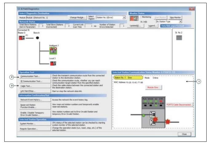
Figure 2.1 Diagnostic Window/Operation Locations (GX Works2)
