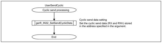
Figure 6.13 Flowchart for Cyclic Send Processing
