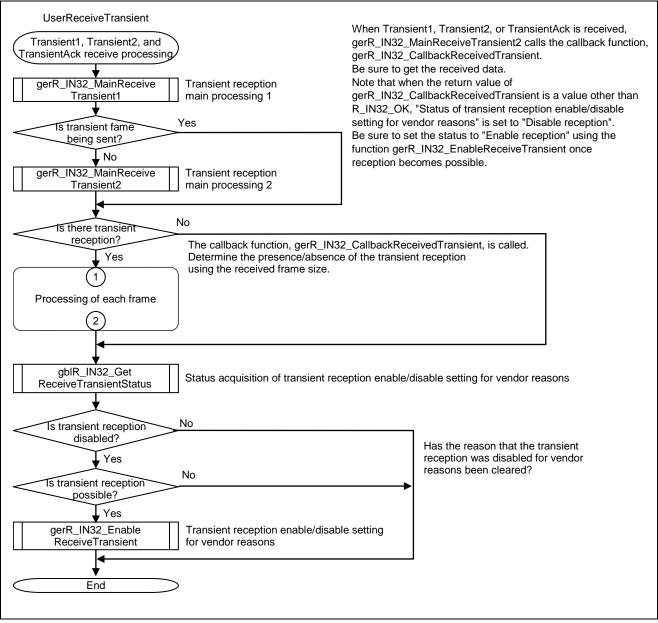
Figure 6.17 Flowchart for Transient1, Transient2, and TransientAck Receive Processing (1/2)
