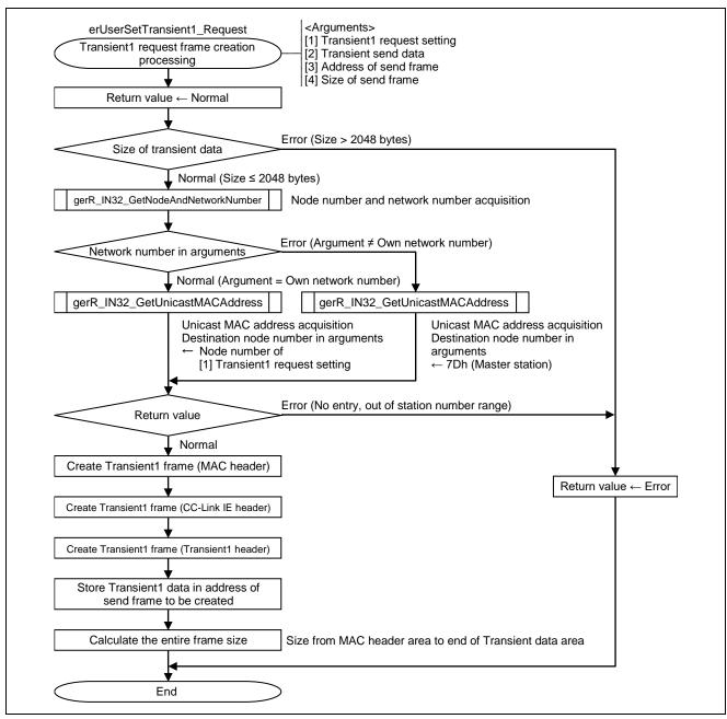
Figure 6.47 Flowchart for Transient1 Request Frame Creation Processing
