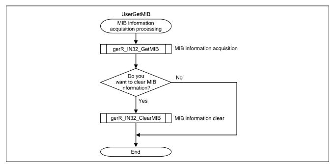
Figure 6.16 Flowchart for MIB Information Acquisition Processing
