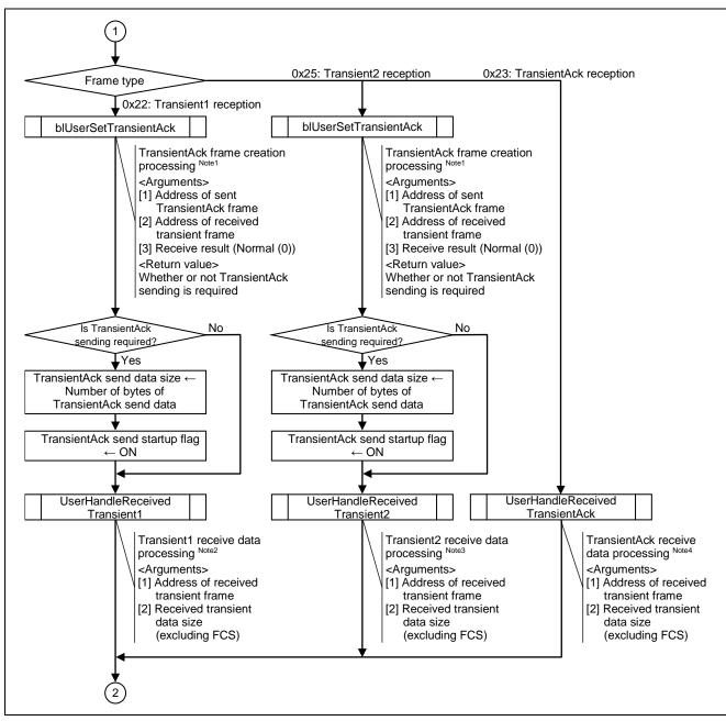
Figure 6.17 Flowchart for Transient1, Transient2, and TransientAck Receive Processing (2/2)
