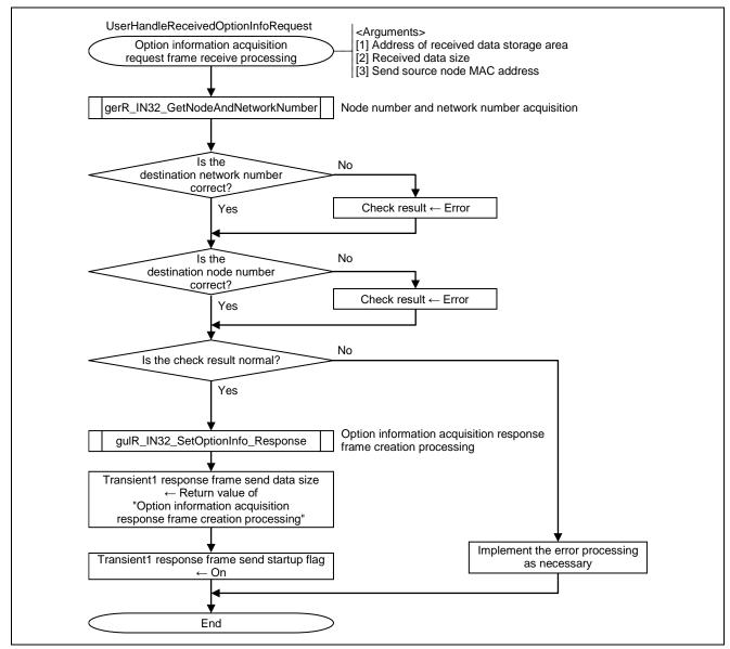
Figure 6.31 Flowchart for Option Information Acquisition Request Frame Receive Processing
