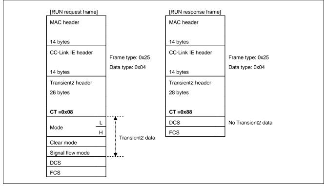
Figure 5.24 Overview of RUN Frame Format
