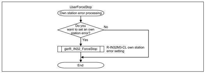
Figure 6.8 Flowchart for Own Station Error Processing
