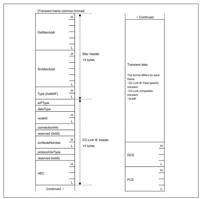
Figure 5.8 Transient Frame Common Format
