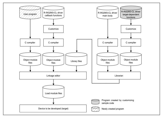
Figure 6.2 Firmware Development Procedure
