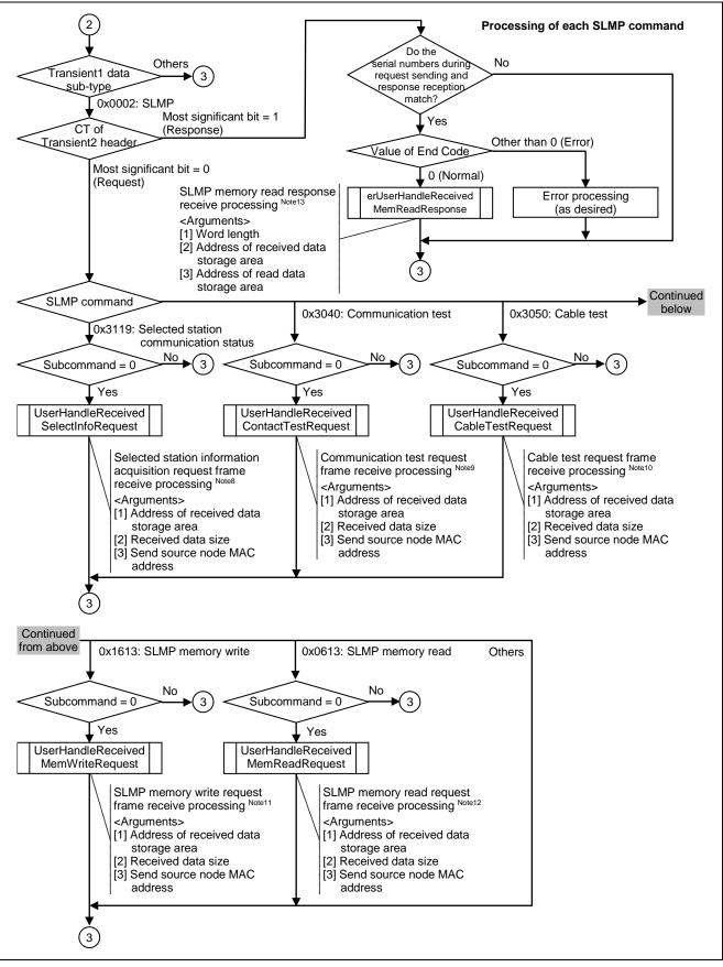
Figure 6.21 Flowchart for Transient1 Receive Data Processing (3/3)
