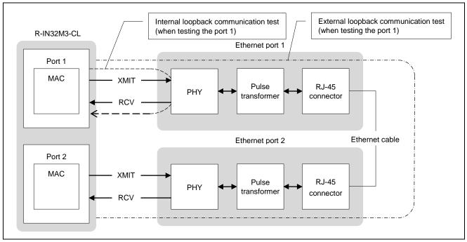
Figure 6.50 Port Schematic Diagram
