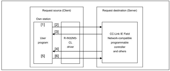
Figure 5.7 Transient2 Request Sending Procedure
