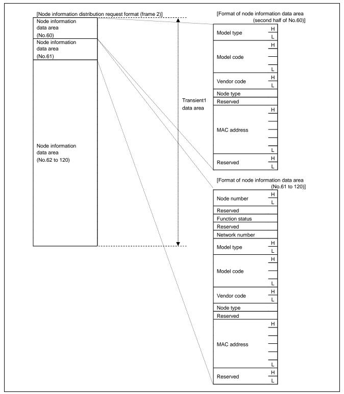
Figure 5.15 Transient1 Data Area: Node Information Distribution Request (Frame 2)
