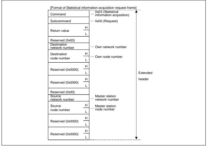
Figure 5.16 Transient1 Data Area: Statistical Information Acquisition Request
