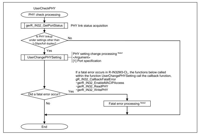
Figure 6.6 Flowchart for PHY Check Processing
