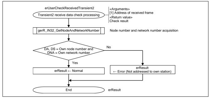
Figure 6.36 Flowchart for Transient2 Receive Data Check Processing
