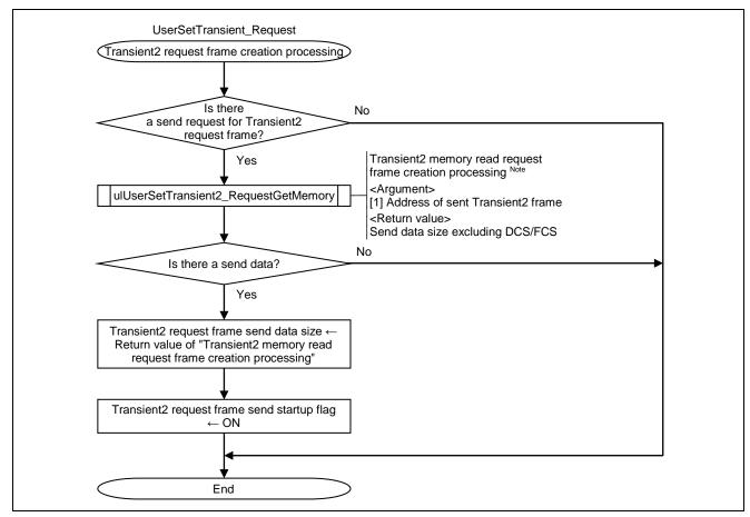
Figure 6.18 Flowchart for Transient2 Request Frame Creation Processing
