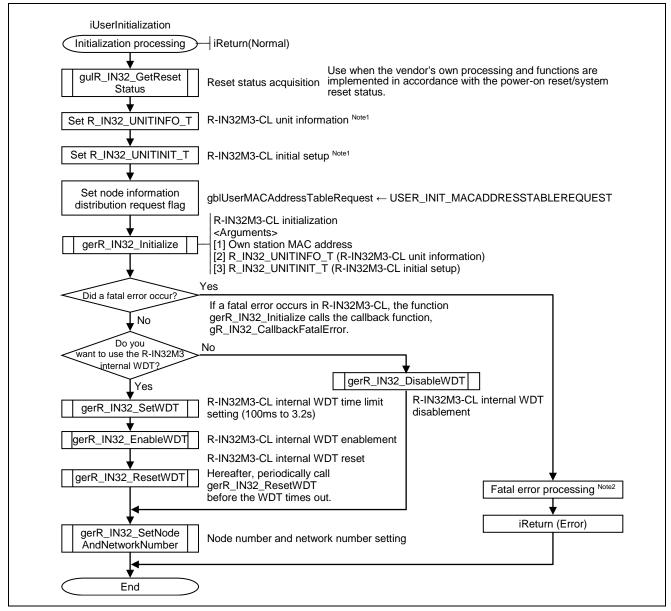
Figure 6.4 Flowchart for Initialization Processing
