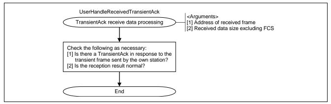
Figure 6.37 Flowchart for TransientAck Receive Data Processing
