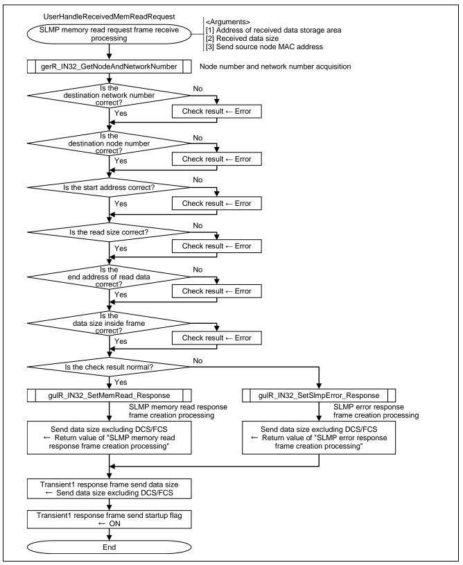
Figure 6.43 Flowchart for SLMP Memory Read Request Frame Receive Processing
