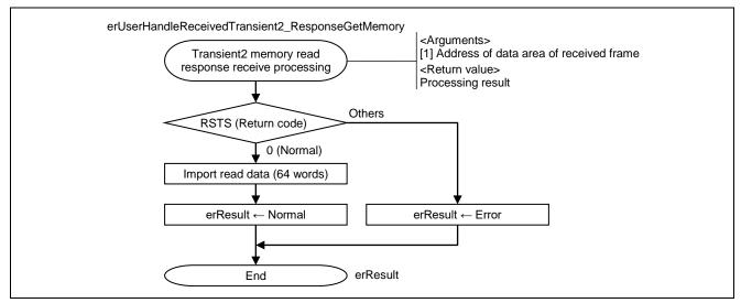
Figure 6.42 Flowchart for Transient2 Memory Read Response Receive Processing
