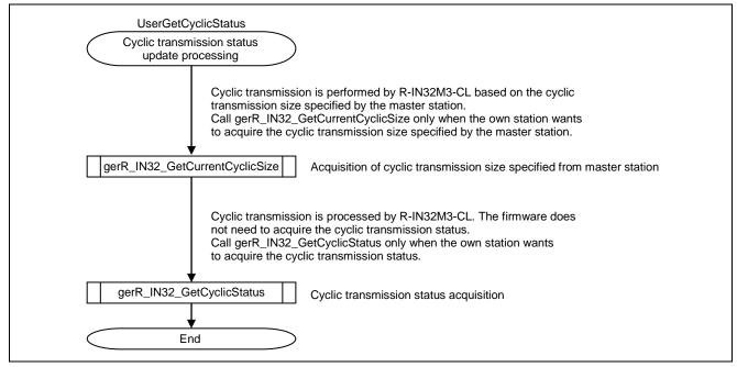
Figure 6.15 Flowchart for Cyclic Transmission Status Update Processing
