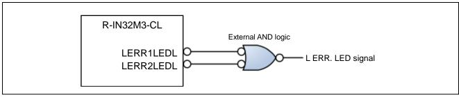
Figure 4.1 External AND Logic for Turning L ERR. On
