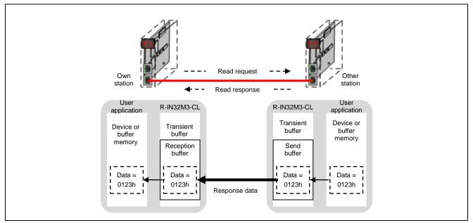
Figure 5.2 Flow of Transient Data
