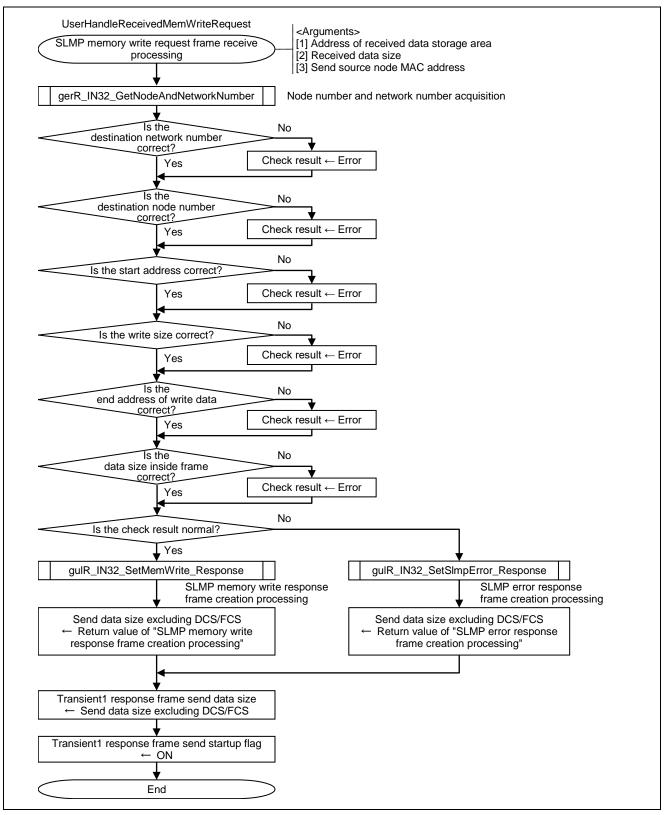
Figure 6.44 Flowchart for SLMP Memory Write Request Frame Receive Processing
