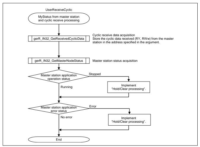
Figure 6.11 Flowchart for MyStatus from Master Station and Cyclic Receive Processing
