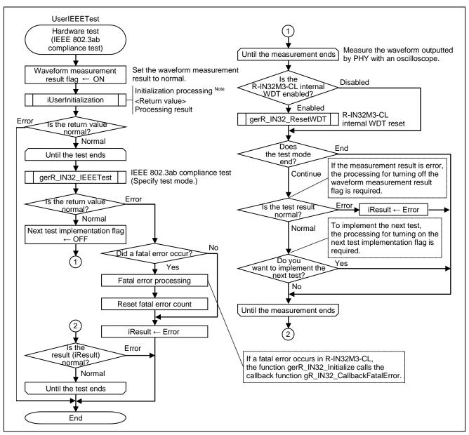
Figure 6.49 Flowchart for Hardware Test (IEEE 802.3ab Compliance Test)
