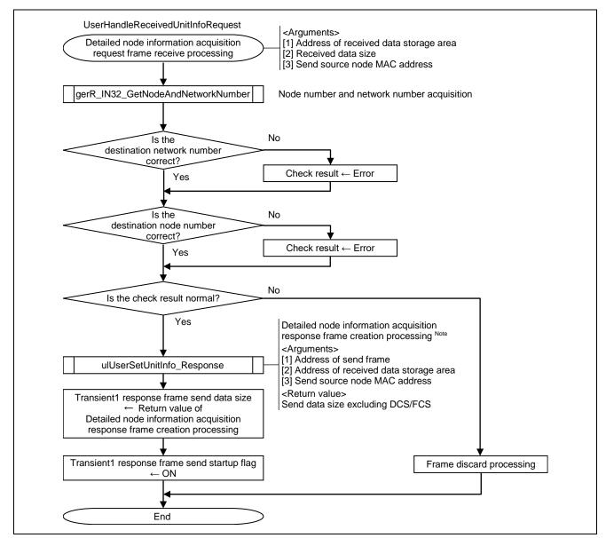
Figure 6.29 Flowchart for Detailed Node Information Acquisition Request Frame Receive Processing
