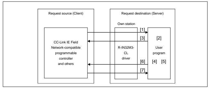
Figure 5.4 Transient1 Request Reception Procedure
