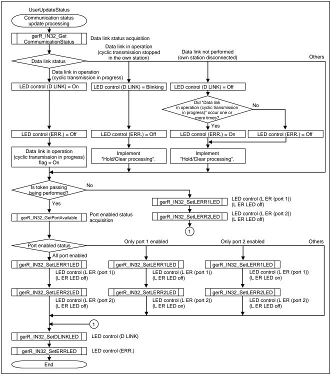
Figure 6.14 Flowchart for Communication Status Update Processing
