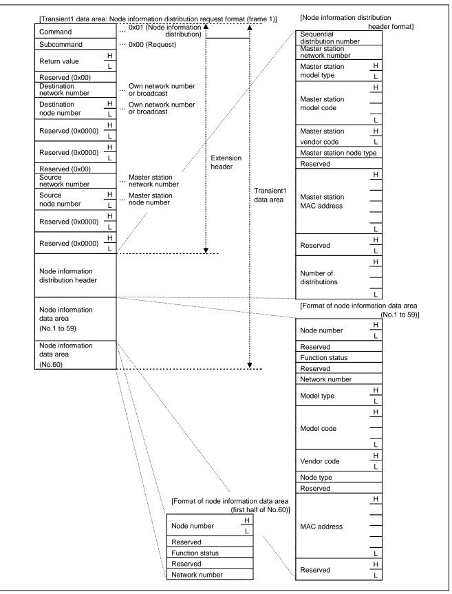
Figure 5.14 Transient1 Data Area: Node Information Distribution Request (Frame 1)
