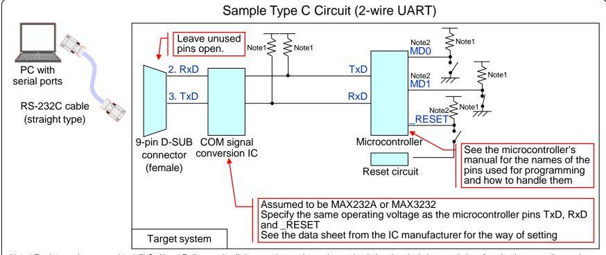
Note1 Resistance is assumed to 4.7kΩ. About Pull-up and pull-down resistor values, please check the electrical characteristics of each microcontroller, and use the appropriate resistor values.
