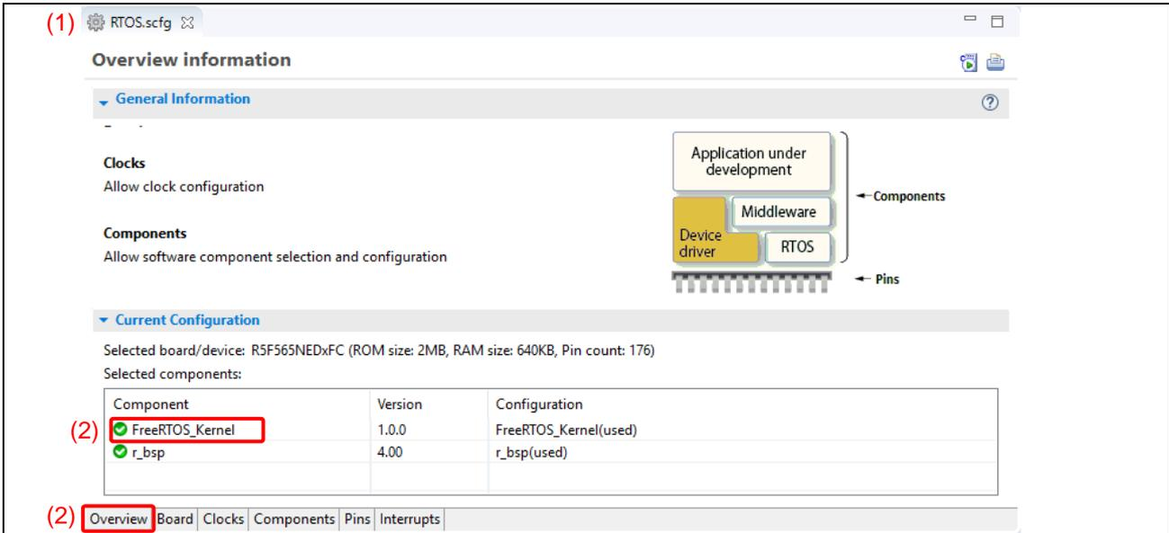
Figure 2-1 Smart Configurator perspective with FreeRTOS™
