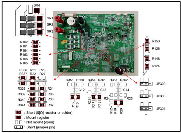
Figure 3-1 Factory Default Settings (Sensorless Vector Control)
