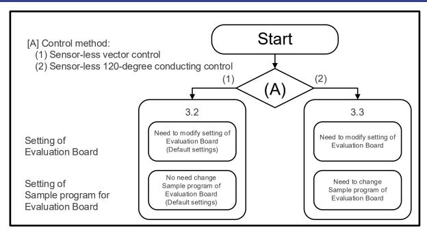
Figure 3-2 Setting of RAJ306101 RSSK for Motor Evaluation
