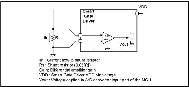
Figure 4-7 Current Sense Circuits (Internal)
