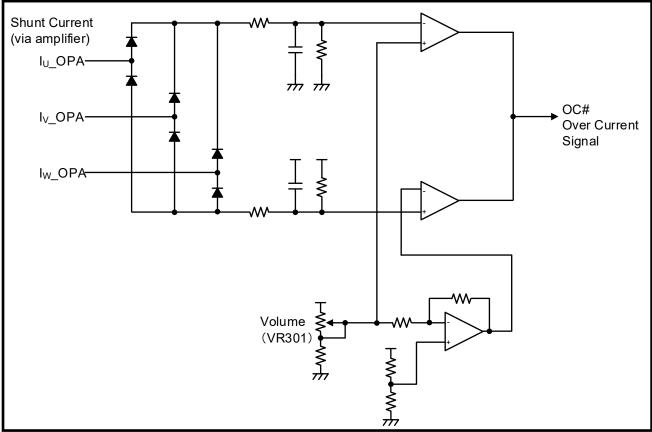
**Figure 4-6 Overcurrent Detection Circuit**
