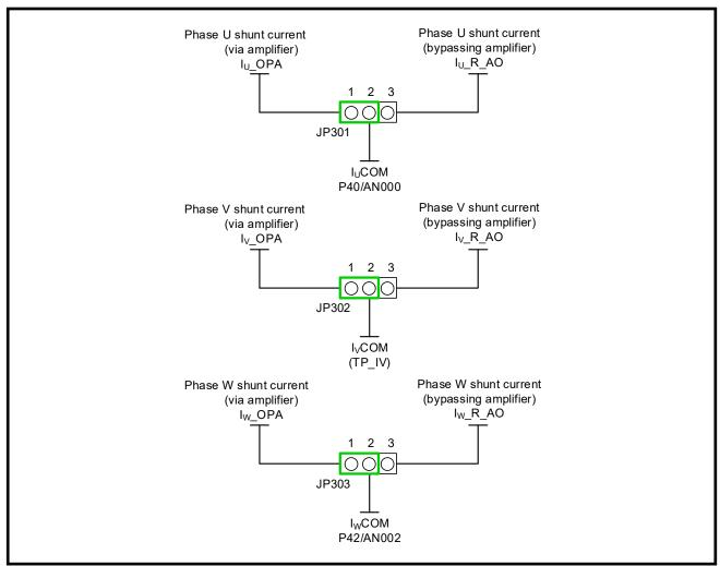
Figure 4-9 Current Sense Circuits (External) Function Selection Jumper
