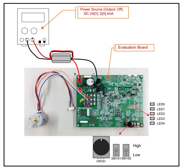
Figure 3-5 Initial Settings for Evaluation Board
