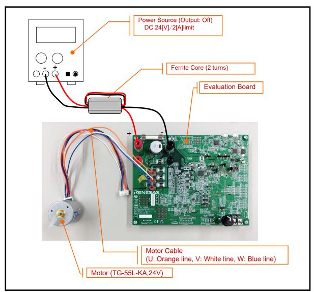
**Figure 3-11 Connections for Evaluation Environment**
