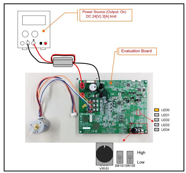
Figure 3-13 Power Supply for Evaluation Board
