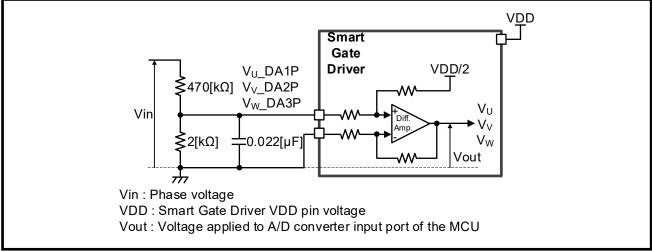
Figure 4-11 Phase Voltage Detection Circuit
