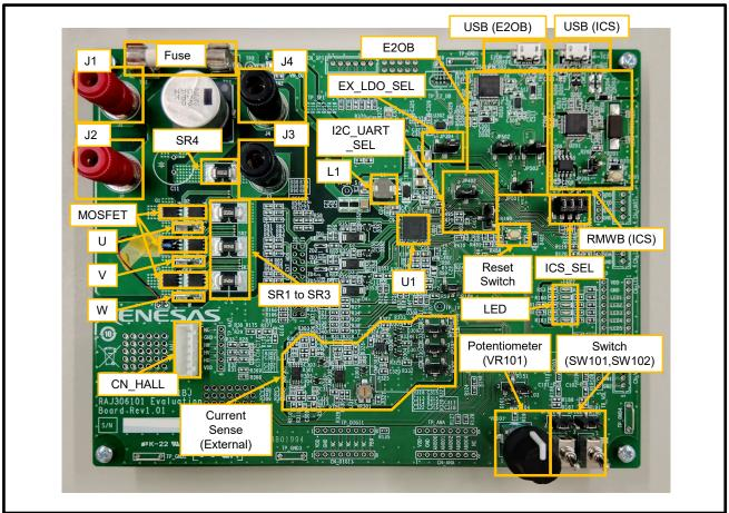
Figure 2-3 Main Parts, Terminals, and Connectors
