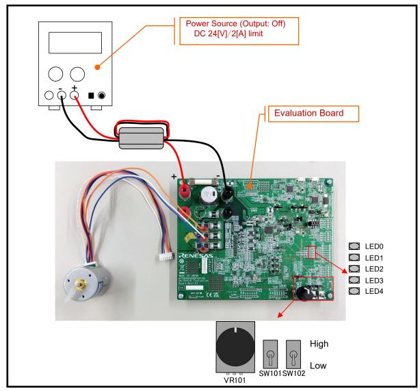
Figure 3-9 Stop Power Supply.
