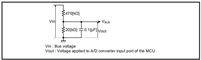
Figure 4-10 Bus Voltage Detection Circuit
