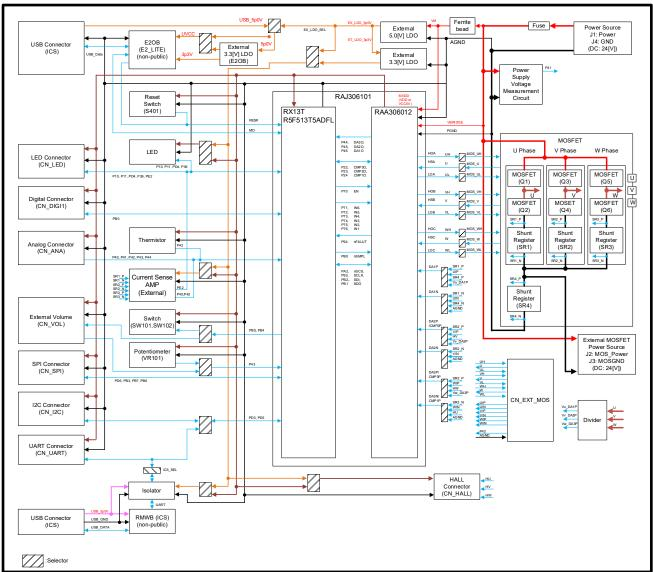
Figure 2-2 Block Diagram
