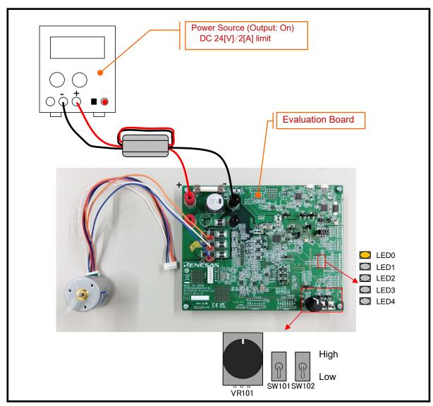
Figure 3-6 Power Supply for Evaluation Board
