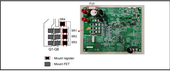
Figure 4-13 Components Change Location (Using Other Motor)
