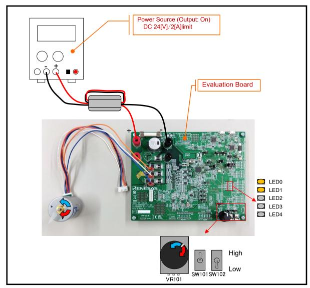
**Figure 3-14 Motor Operation**
