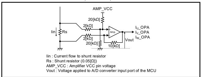
Figure 4-8 Current Sense Circuits (External)
