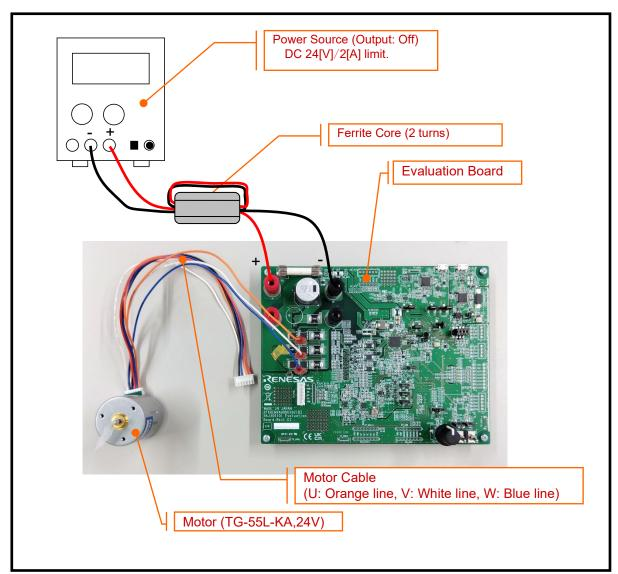
Figure 3-4 Connections for Evaluation Environment
