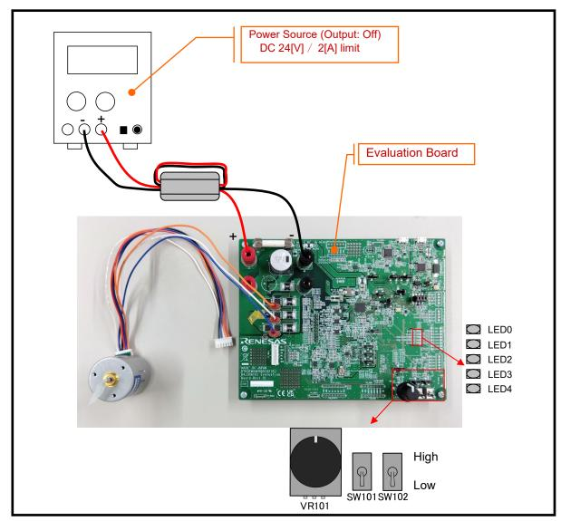
Figure 3-12 Initial Settings for Evaluation Board
