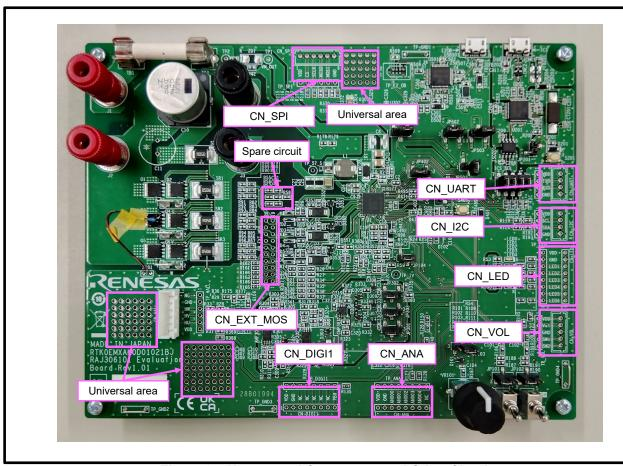
Figure 2-4 Unmounted Connectors and Other Circuits **Table 2-5 Unmounted Connectors and Other Circuits List**
