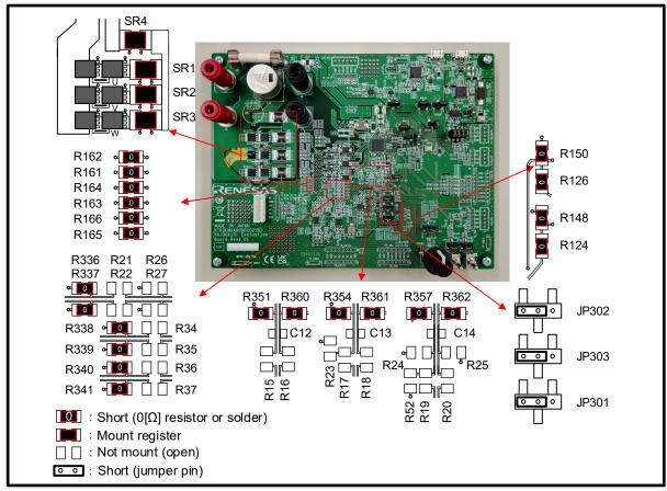
Figure 3-10 Board Connection Settings (Sensorless 120-degree Conducting Control)
