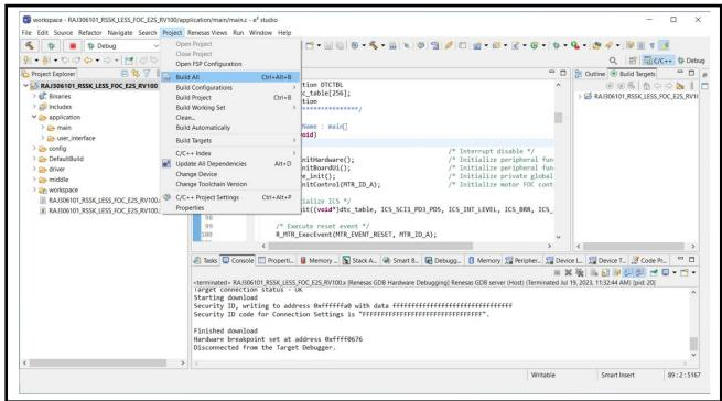
Figure 5-2 Firmware Build
