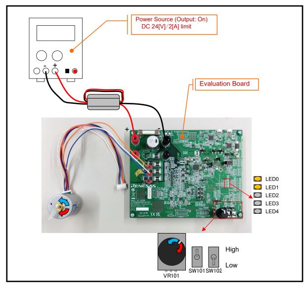
**Figure 3-7 Motor Operation**
