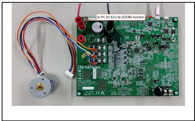
Figure 5-1 Connect with PC (E2 Lite Function)
