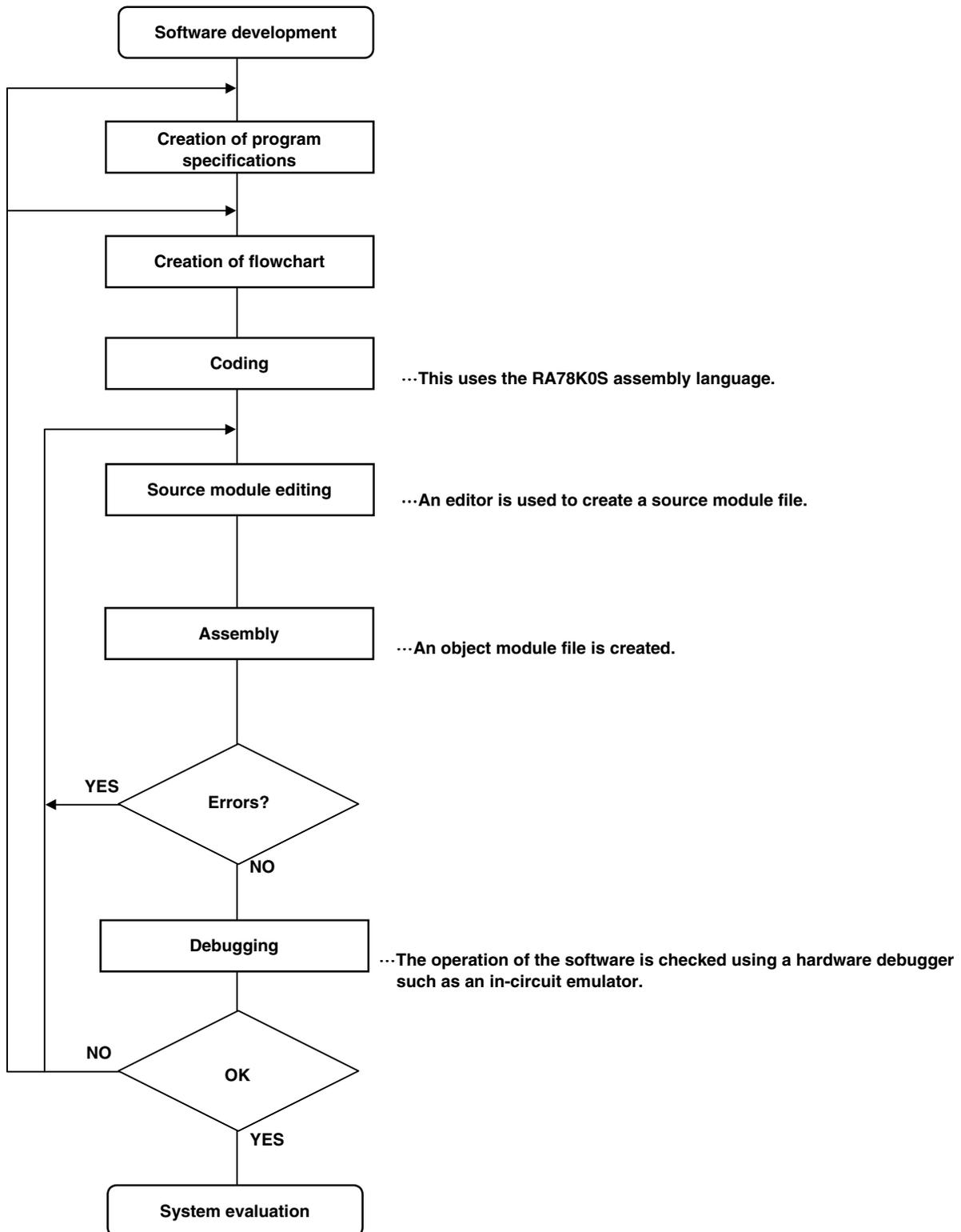
The RA78K0S is then applied to the assembly process.
