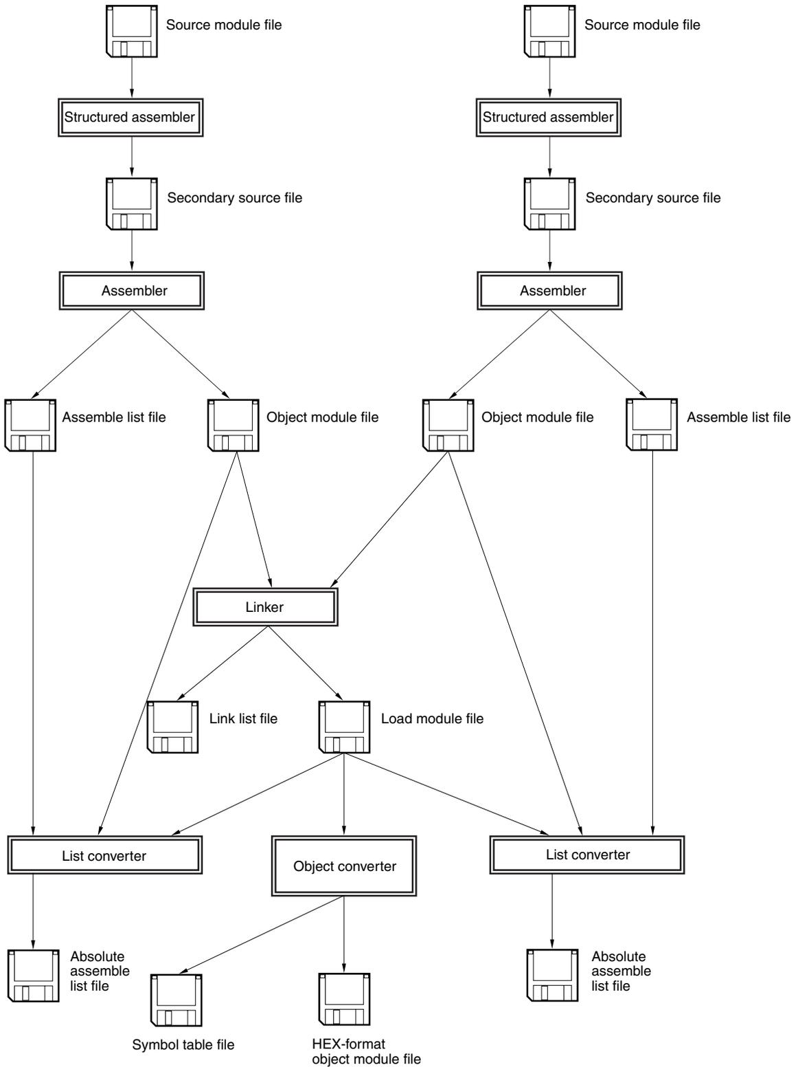
Figure 3-3. RA78K0S Execution Procedure 2
