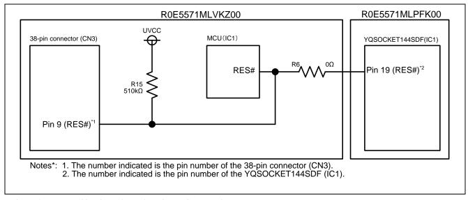
Figure 2 Reset Circuit on the Debugging MCU Board
