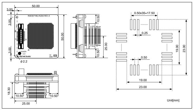
Figure 4 Reference Foot Pattern and Dimensions of This Product (R0E5571MLDMB01)
