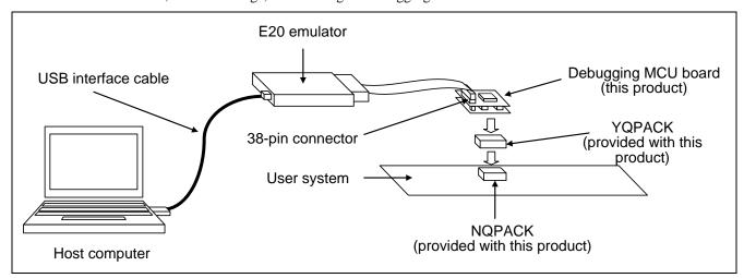
Figure 1 System Configuration
