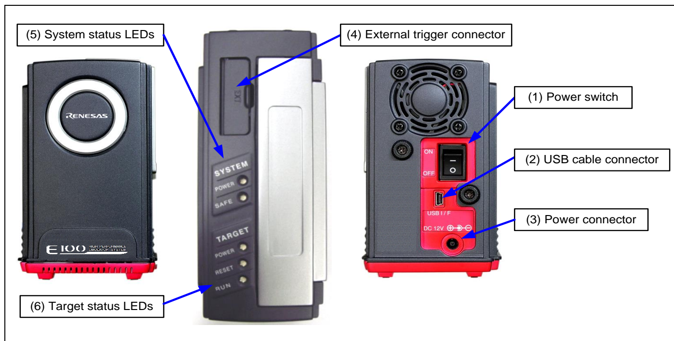
Figure 1.2 Names of each part of the emulator
