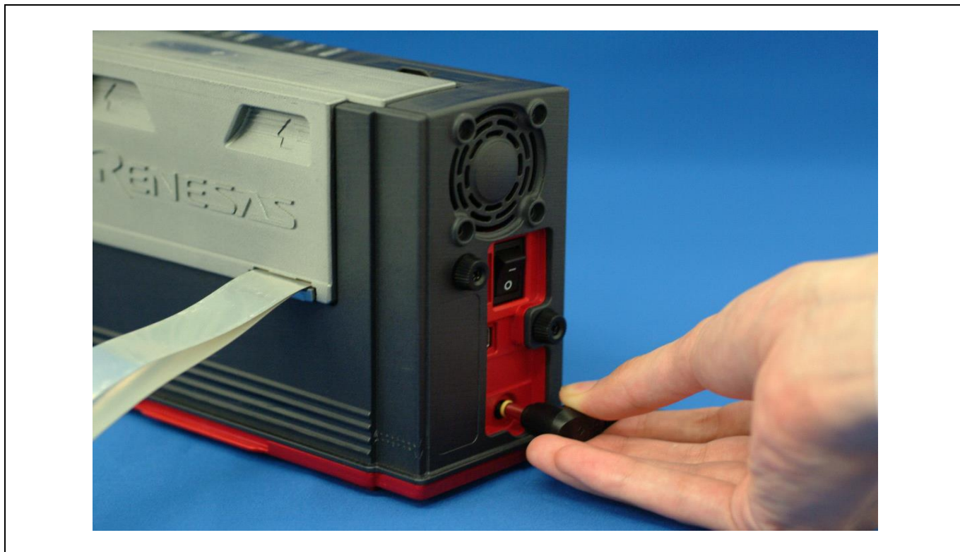
Figure 2.5 Connecting the emulator power supply
