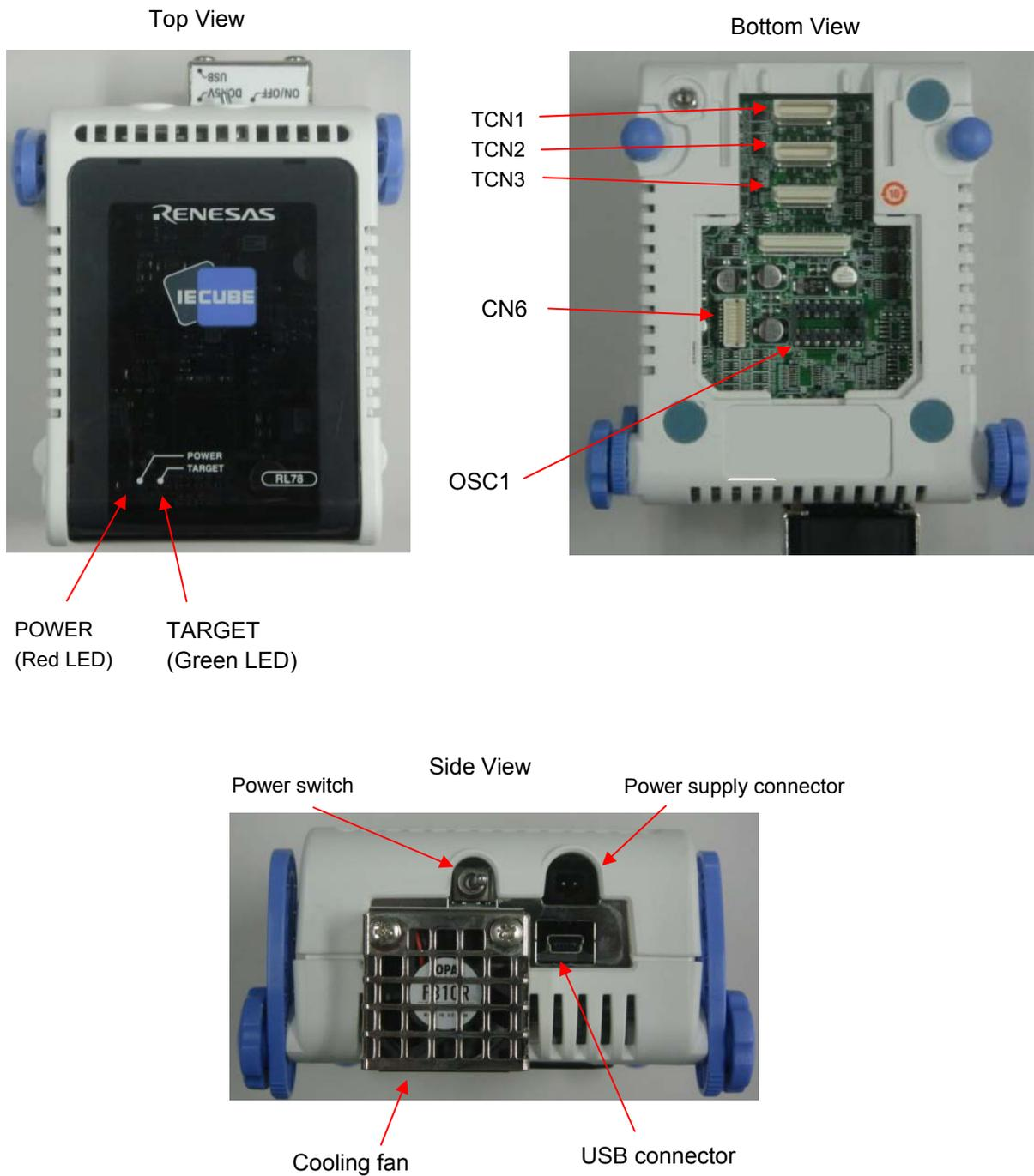
Figure 1-1. Names of Parts of QB-RL78L12
