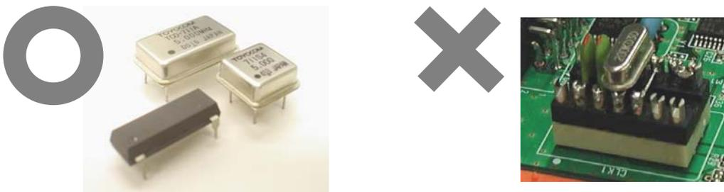
Figure 2-2. Oscillator Shape
