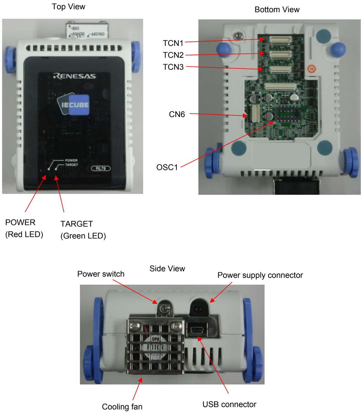
Figure 1-1. Names of Parts of QB-RL78G1C
