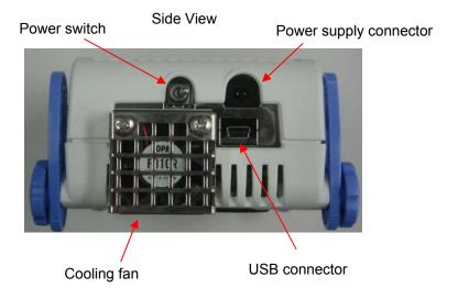
Figure 1-1. Names of Parts of QB-RL78F14
