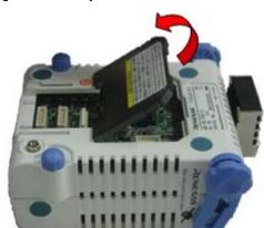
Figure 2-1. Acrylic Board Removal Method
