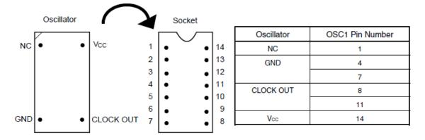
**Remark** Insert the oscillator into the socket, take care for the pin 1 position.
