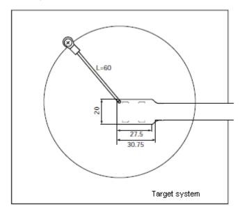
Figure 2-6 Where GND Wire Can Be Connected
