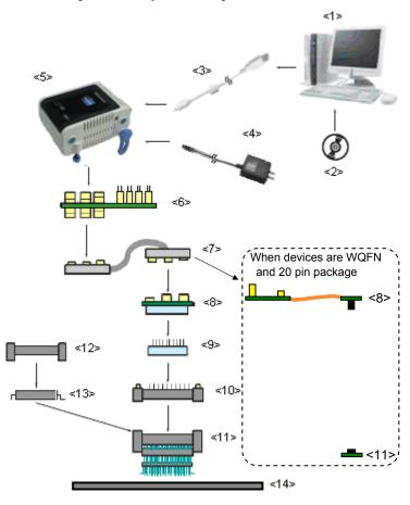
Figure 1-2. System Configuration
