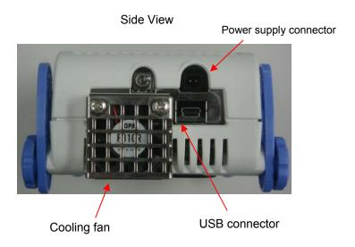
Figure 1-1. Names of Parts of QB-RL78F12
