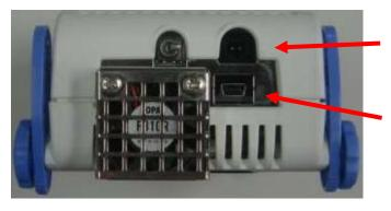
Power supply connector (Connect AC adapter)
