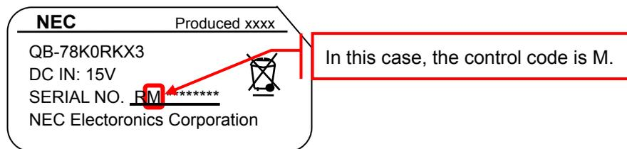
**Figure 2. Checking Control Code (ID78K0R-QB)**
