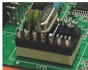
Figure 2-3. Oscillator Shape
