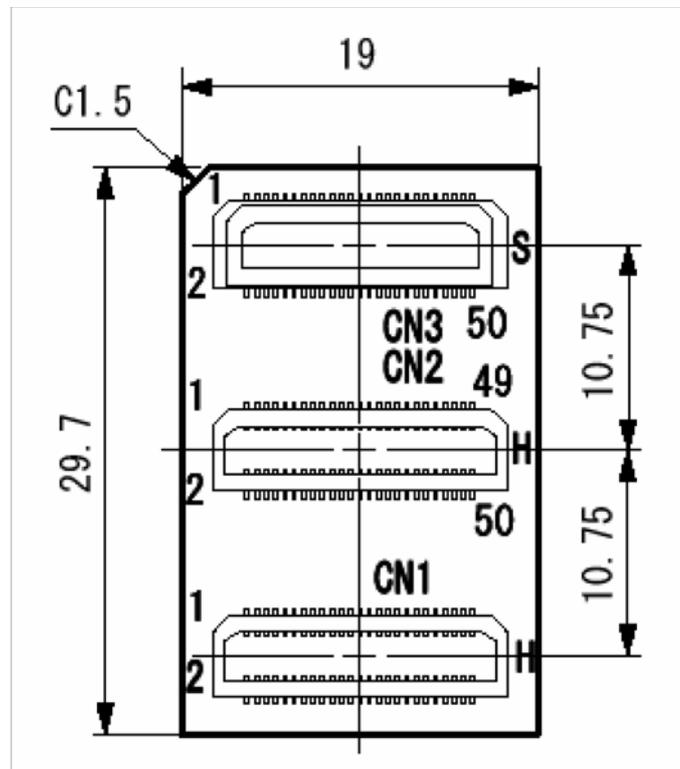
Figure 5-4: Exchange Adapter for 100-pin bottom view
