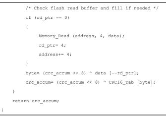
Figure B.3 16-bit CRC Calculation Specifications
