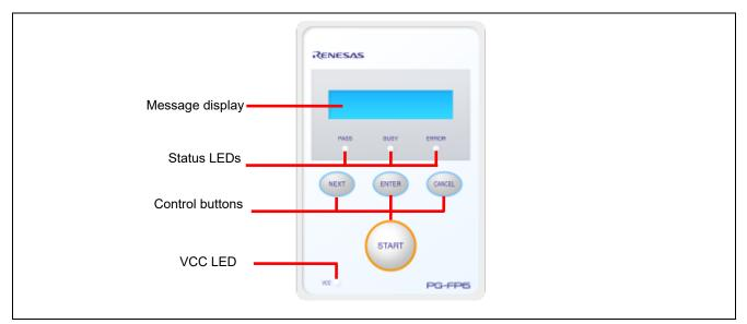
Figure 2.1 FP6 Top View <Control Panel>
