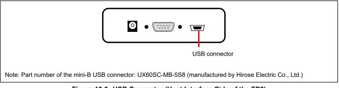
Figure 10.6 USB Connector (Host Interface Side of the FP6)
