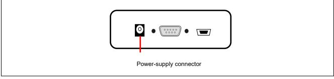
Figure 10.1 Power-Supply Connector
