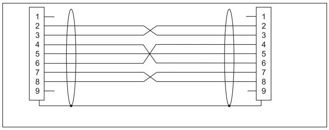
Figure 10.5 Connection of the Serial Cable
