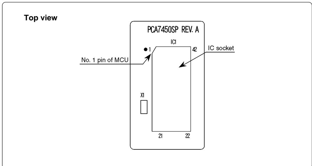
Figure 4.4 Mounting an MCU (PCA7450SP)
