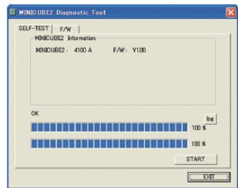
If the firmware version is not the latest, refer to the MINICUBE2 diagnostic tool user's manual and update the firmware. After self-testing and firmware version checking are completed, disconnect MINICUBE2 and the host machine once.
