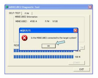
When self-testing for the second or later time, "NG" is displayed for items with which NG is detected, in the result dialog box of (6) in **3.3 Execution of Self-Testing**. Click the [OK] button.
