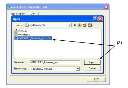
(4) Confirm that the path to the folder where MINICUBE2 firmware is stored is displayed in the path indication area, and the specified MINICUBE2 firmware is displayed in [File Name] .
