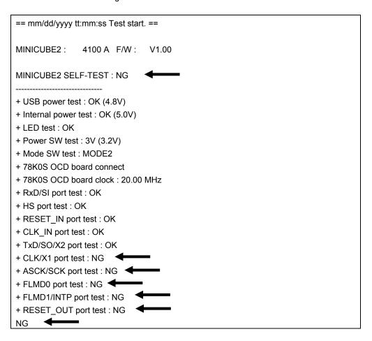
If the test result includes "NG" as shown above, the cause may be a defect in MINICUBE2. Refer to **3.2 Cautions** on **Self-Testing** and **3.5.2 Action for error**, and retry self-testing. If the same items resulted in "NG" even after the relevant action is implemented, the cause may be a defect in MINICUBE2. In such a case, consult an NEC Electronics sales representative or distributor.
