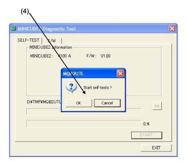
(5) The upper progress bar indicates the progress status of the test currently being performed. The lower progress bar indicates the status of progress for overall self-testing.
