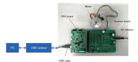
Figure 4-7 Board connection (using VCOM port)
