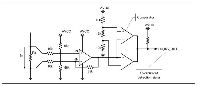
Figure 5-3 Overcurrent detection circuit
