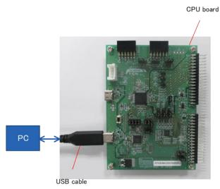
Figure 4-9 Board connection (CPU board only)
