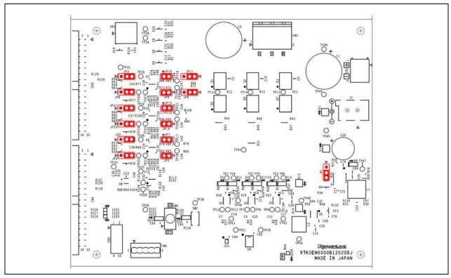
Figure 4-5 Default jumper pin setting
