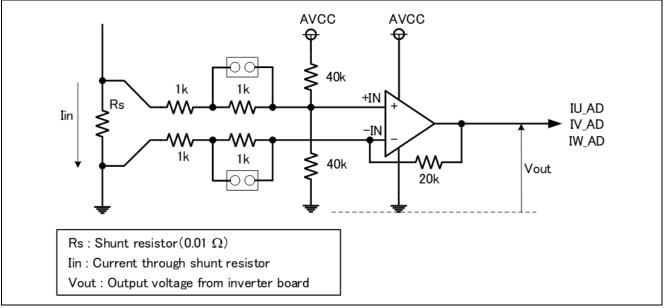
Figure 5-2 Current detection circuit
