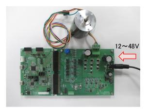
Figure 4-10 Power supply from DC jack
