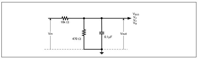
Figure 5-4 Output voltage detection circuit
