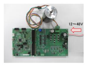
Figure 4-11 Power supply from terminal block
