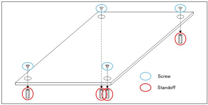
Figure 4-4 Standoffs and Screws assembly
