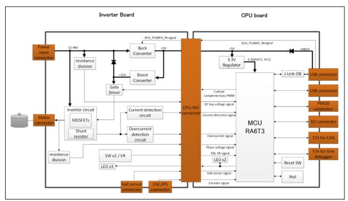
Figure 4-1 MCK-RA6T3 block diagram
