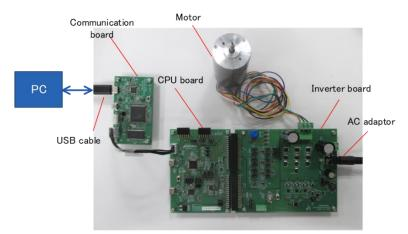
Figure 4-8 Board connection (using communication board)
