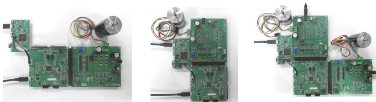
(1)CPU board + INV board (connected with CN1,CN2)
