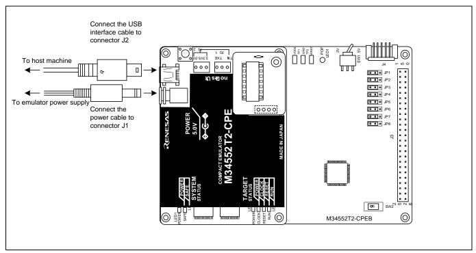
Figure 2.4 Connecting the emulator system
