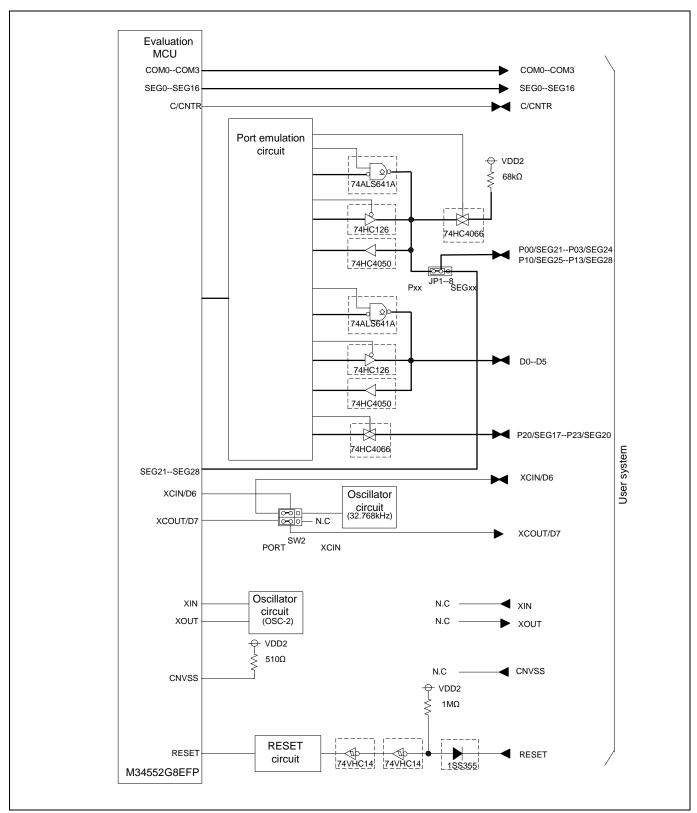
Figure 4.2 Connection diagram
