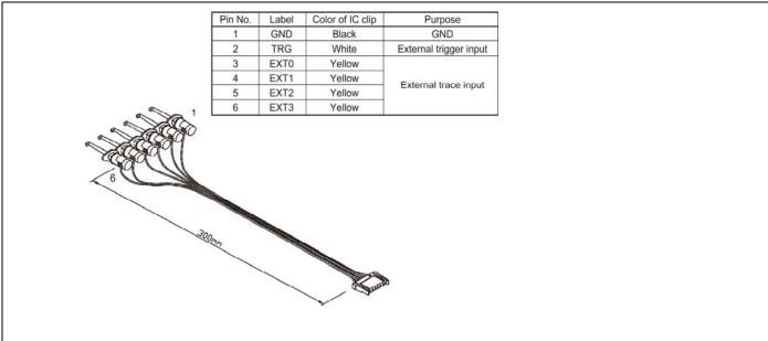
Figure 2.19 Pin assignment of the external trace cable
