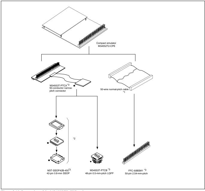
Figure 2.10 Connection of the M34552T2-CPE and user system
