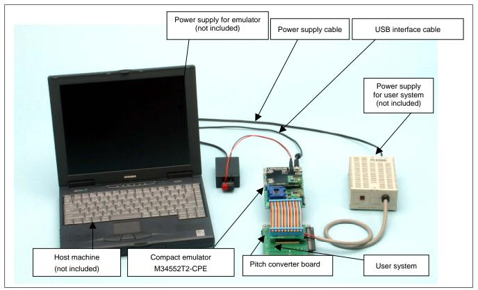
Figure 1.1 System configuration
