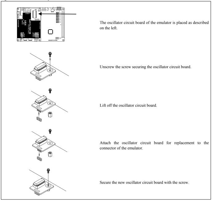
Figure 2.15 Replacing oscillator circuit boards
