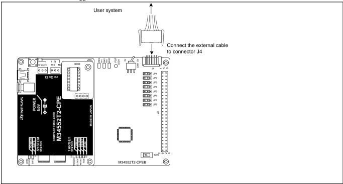
Figure 2.18 Connecting the external trace/trigger cable
