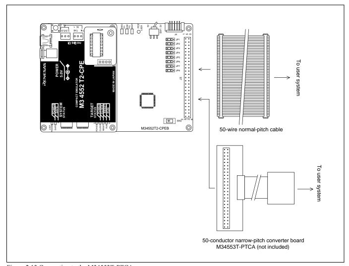
Figure 2.13 Connecting to the M34553T-PTCA
