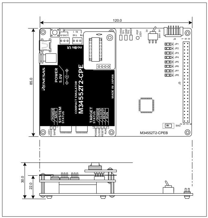
Figure 4.3 External dimensions of the compact emulator
