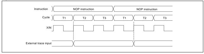
Figure 2.20 Latch timing of external trace input
