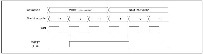
Figure 2.23 Output waveform of the check pin WRST
