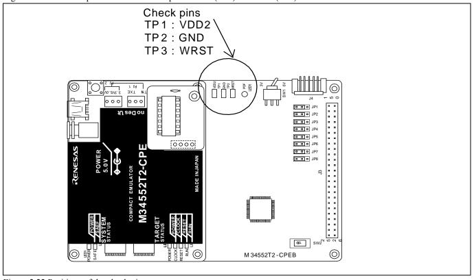
Figure 2.22 Positions of the check pins
