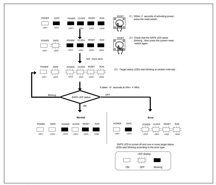
Figure 2.9 Self-check procedure
