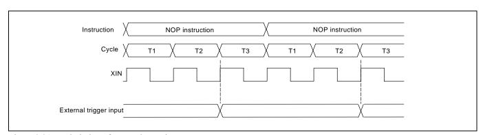
Figure 2.21 Latch timing of external trace input
