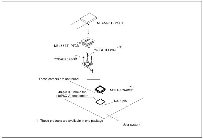
Figure 2.14 Connecting to the 48-pin 0.5-mm-pitch LQFP package foot pattern
