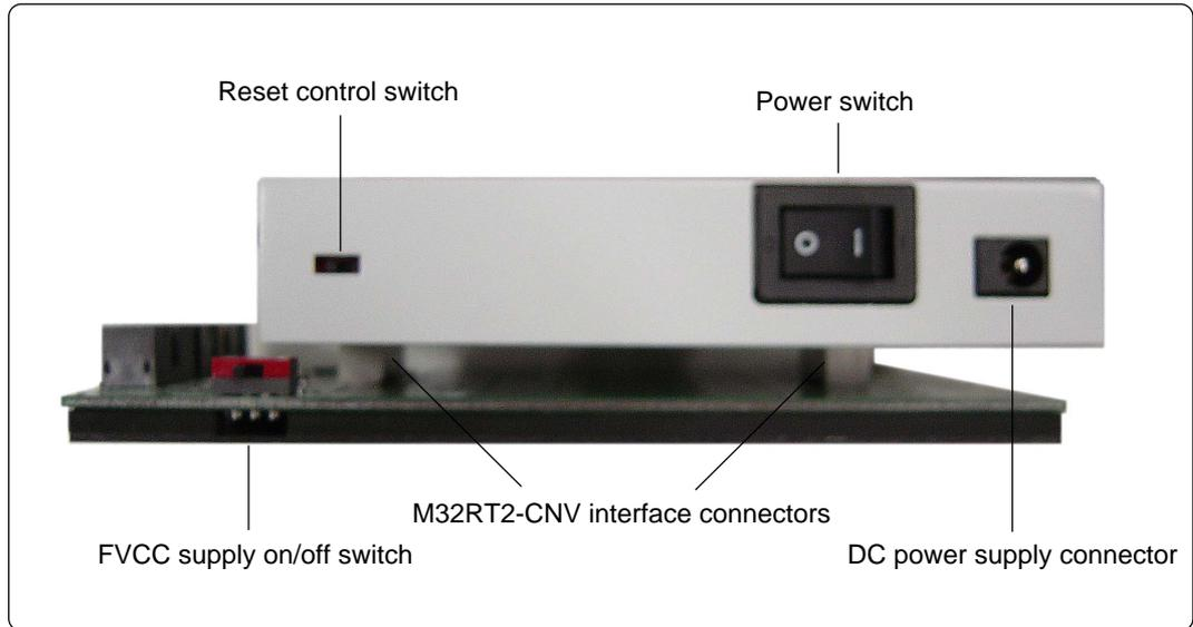
Figure 2.4 Name of each part on the side panel
