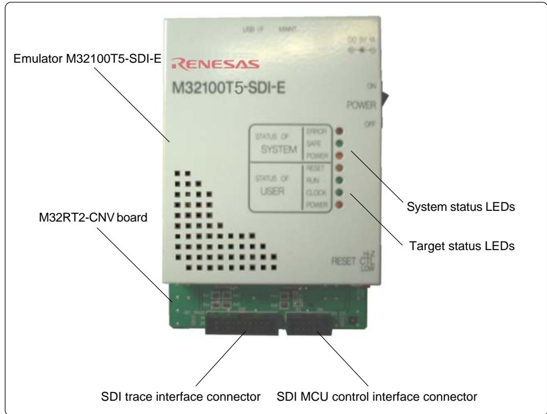
Figure 2.3 Name of each part on the upper panel
