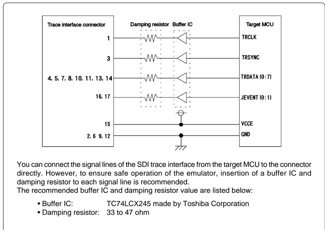
Figure 3.6 Sample circuit of the SDI trace interface
