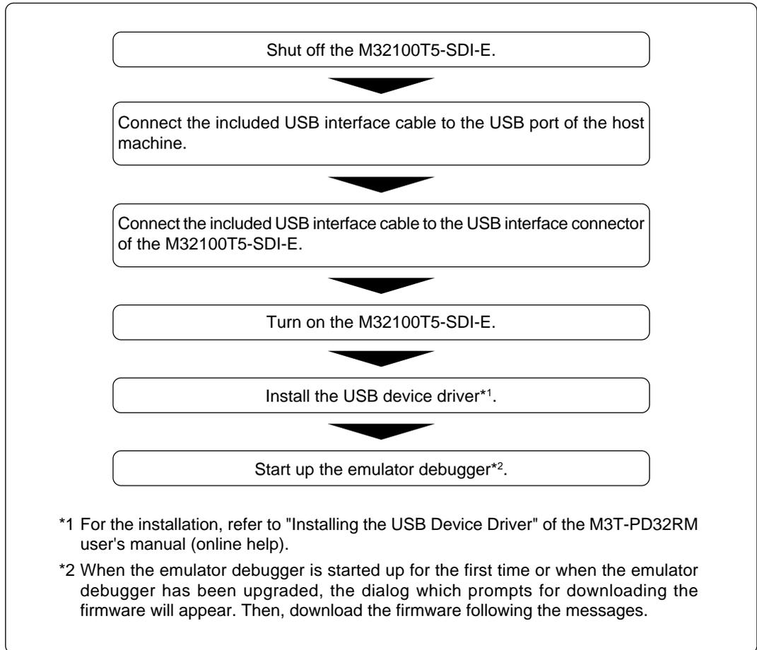
Figure 3.3 USB interface connection procedure
