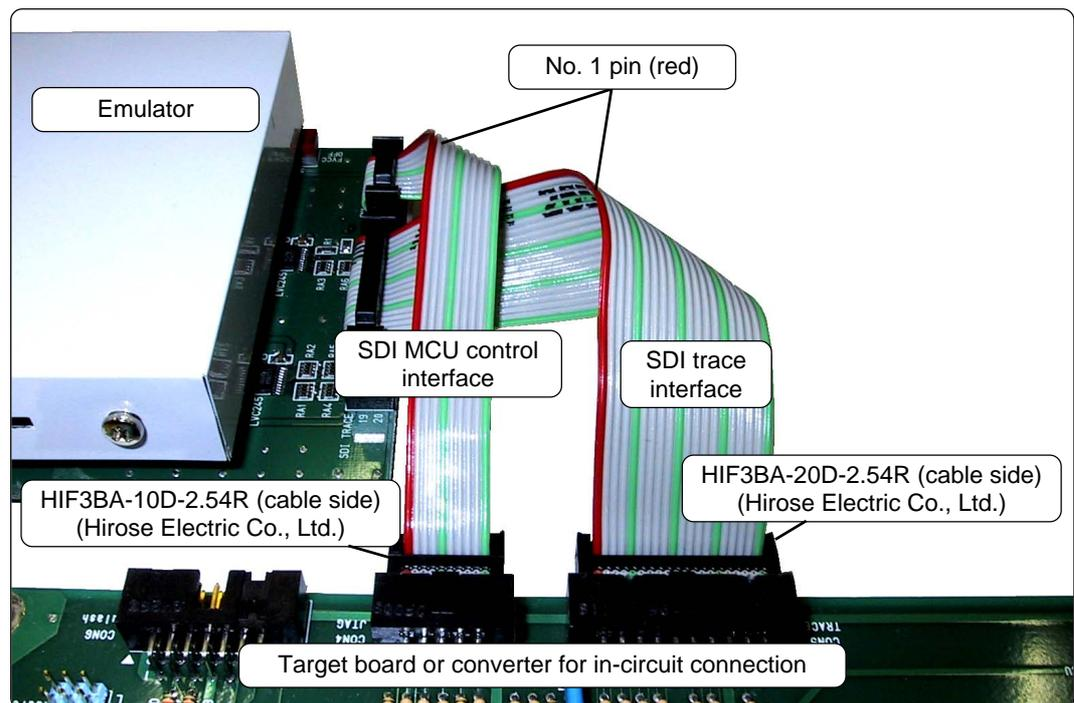
Figure 3.4 Connecting the SDI interface cables
