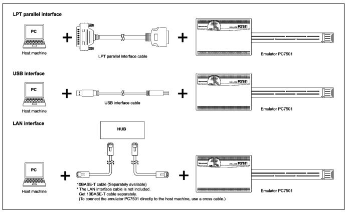
Figure 2.2 Outline for interface cable connections
