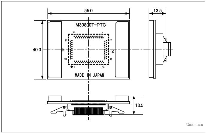
Figure 4.4 External dimensions of the M30800T-PTC
