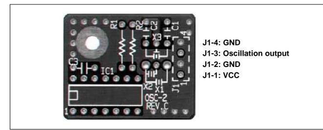
Figure 2.19 External view of the oscillator board OSC-2 (bare board) and connector pin assignments
