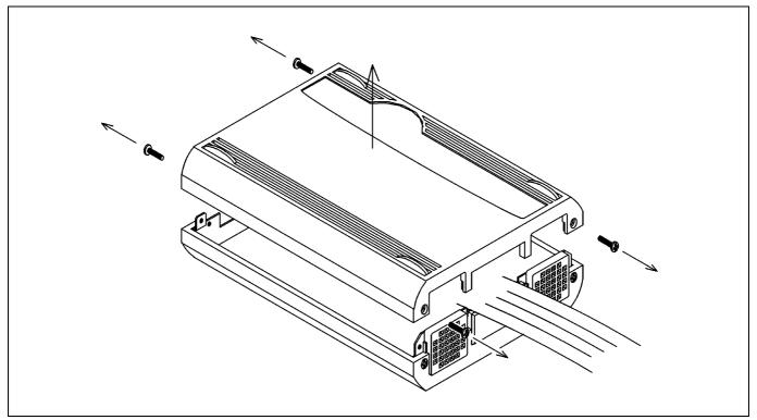
Figure 2.17 Removing the upper cover
