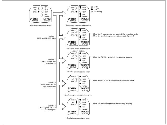
Figure 2.6 Self-check procedure
