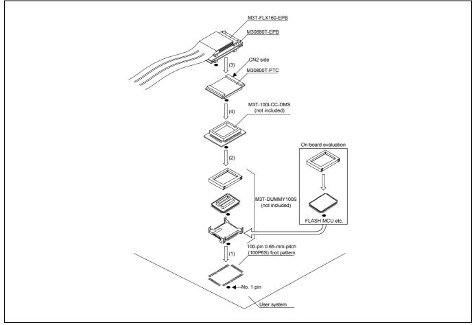
Figure 2.9 Connecting to a 100-pin 0.65-mm-pitch foot pattern (1/3)
