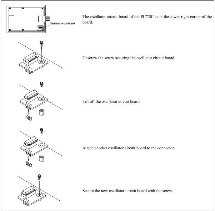
Figure 2.18 Replacing oscillator circuit boards
