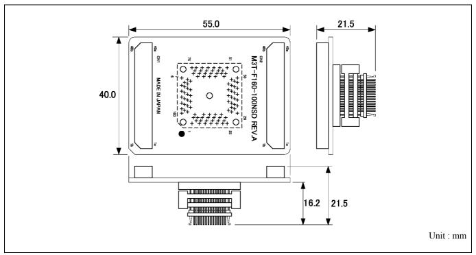
Figure 4.5 External dimensions of the M3T-F160-100NSD
