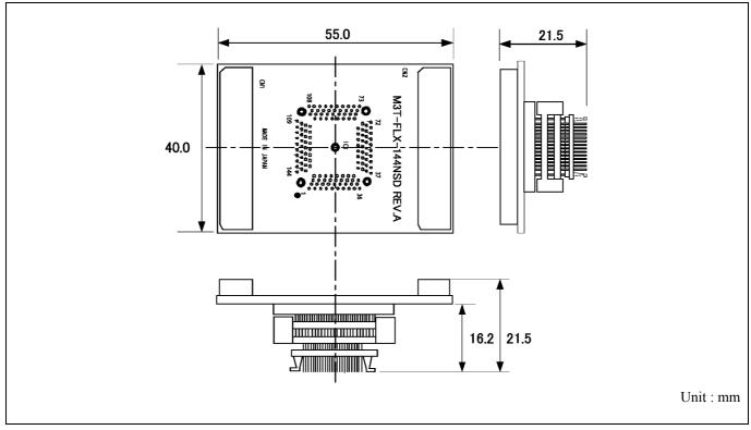
Figure 4.6 External dimensions of the M3T-FLX-144NSD
