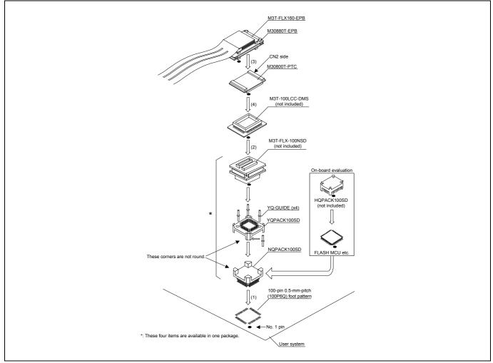
Figure 2.13 Connecting to a 100-pin 0.5-mm-pitch foot pattern (2/3)
