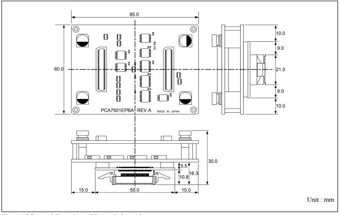
Figure 4.3 External dimensions of the emulation probe
