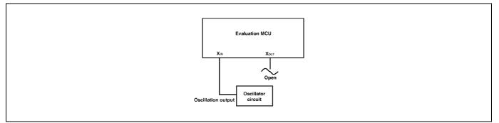
Figure 2.21 External oscillator circuit
