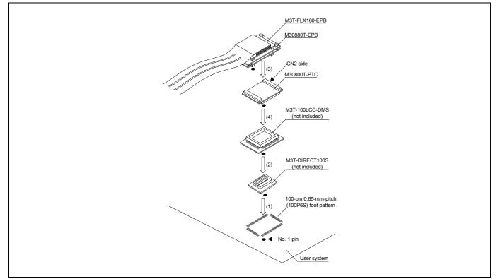
Figure 2.10 Connecting to a 100-pin 0.65-mm-pitch foot pattern (2/3)
