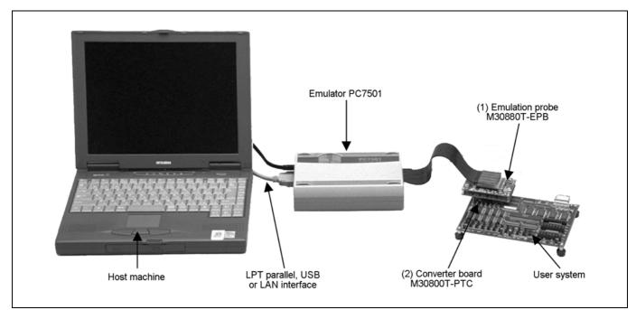
Figure 1.1 System configuration
