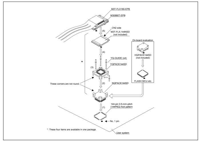
Figure 2.15 Connecting to a 144-pin 0.5-mm-pitch foot pattern
