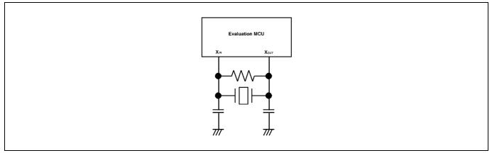
Figure 2.22 Circuit in which oscillation does not occur
