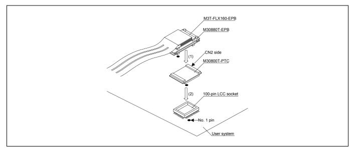
Figure 2.8 Connecting to a 100-pin LCC socket
