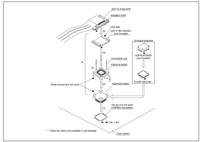
Figure 2.14 Connecting to a 100-pin 0.5-mm-pitch foot pattern (3/3)
