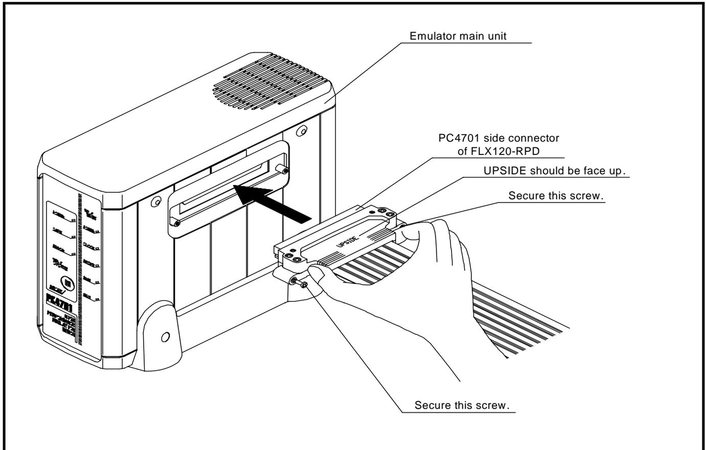
Figure 2.2 Connecting the cable to the PC4701
