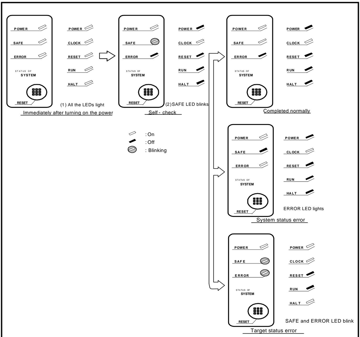
Figure 2.6 LED display in the self-check procedure
