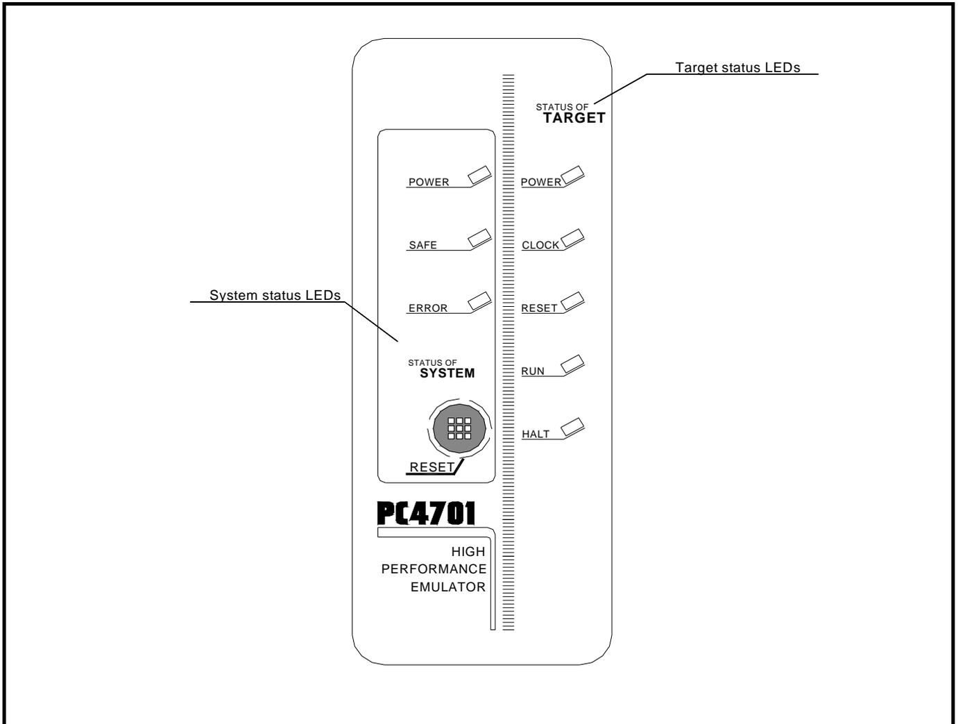
Figure 1.2 Names of the LEDs on the front panel of the PC4701
