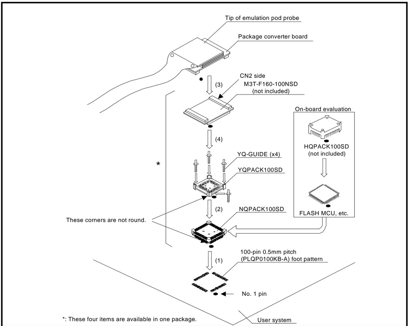
Figure 2.14 Connecting to a 100-pin 0.5mm pitch foot pattern (1/2)
