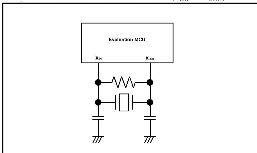
Figure 2.23 Circuit in which oscillation does not occur
