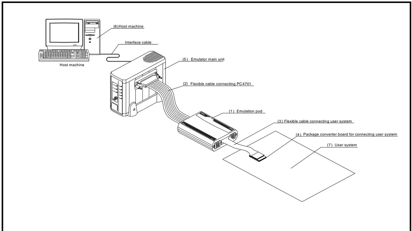
Figure 1.1 System configuration
