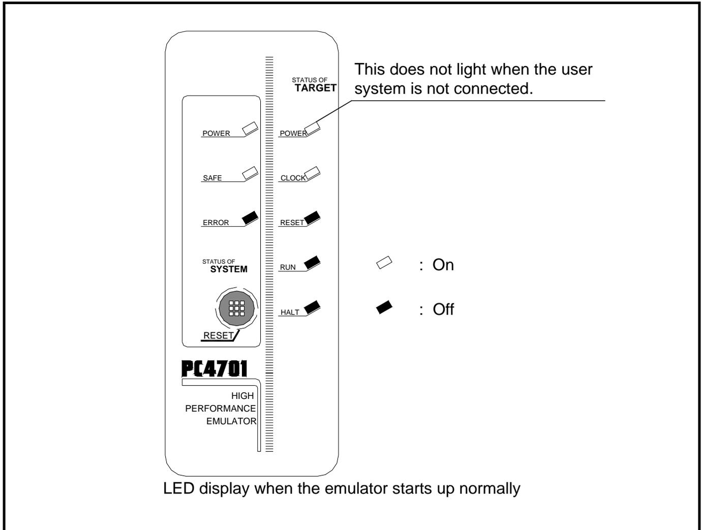
Figure 2.4 LED display when the power turned on
