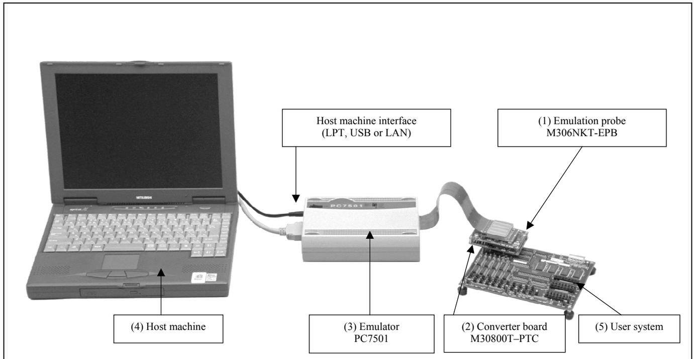
Figure 1.1 System configuration
