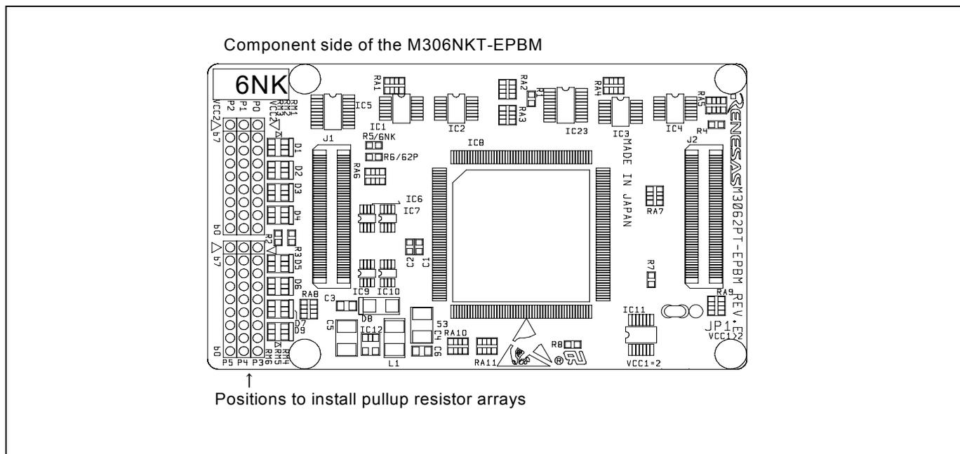
Figure 2.17 Positions of the pullup resistors
