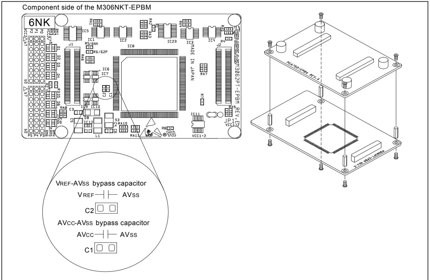
Figure 2.16 Foot pattern for A/D conversion bypass capacitors and the configuration of this product
