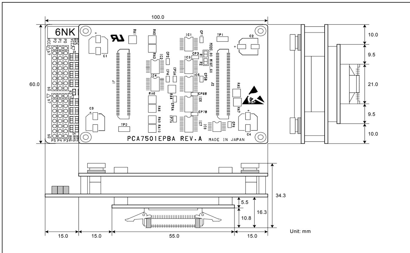
Figure 4.8 External dimensions of the emulation probe
