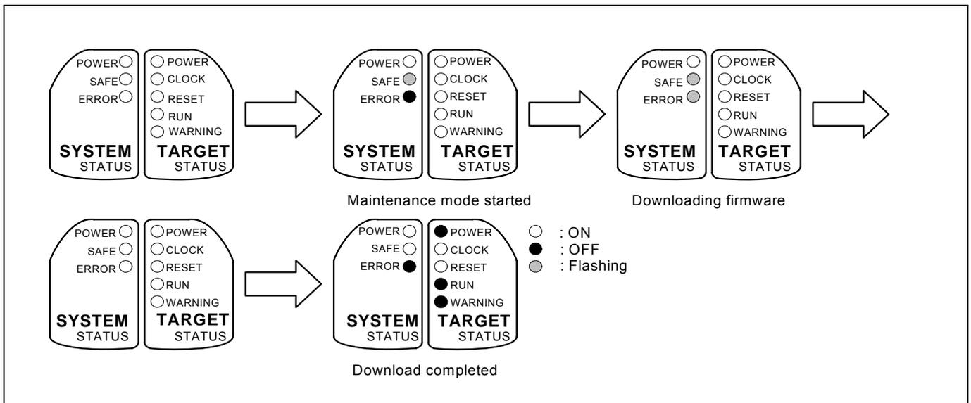
Figure 2.5 LEDs during firmware download in maintenance mode
