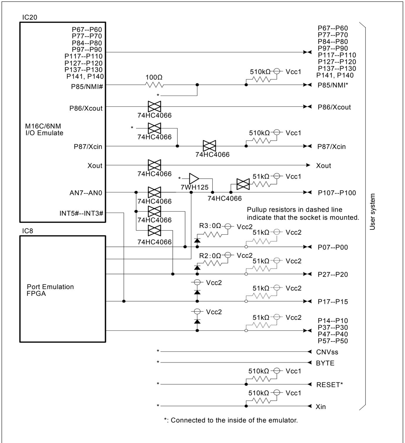
Figure 4.7 Connection diagram
