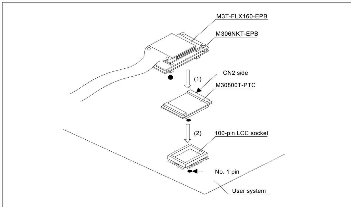
Figure 2.9 Connecting to a 100-pin LCC socket
