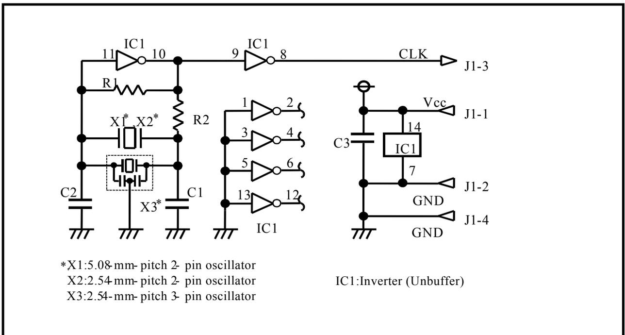
Figure 2.4 Circuits of the OSC-2 oscillator circuit bare board
