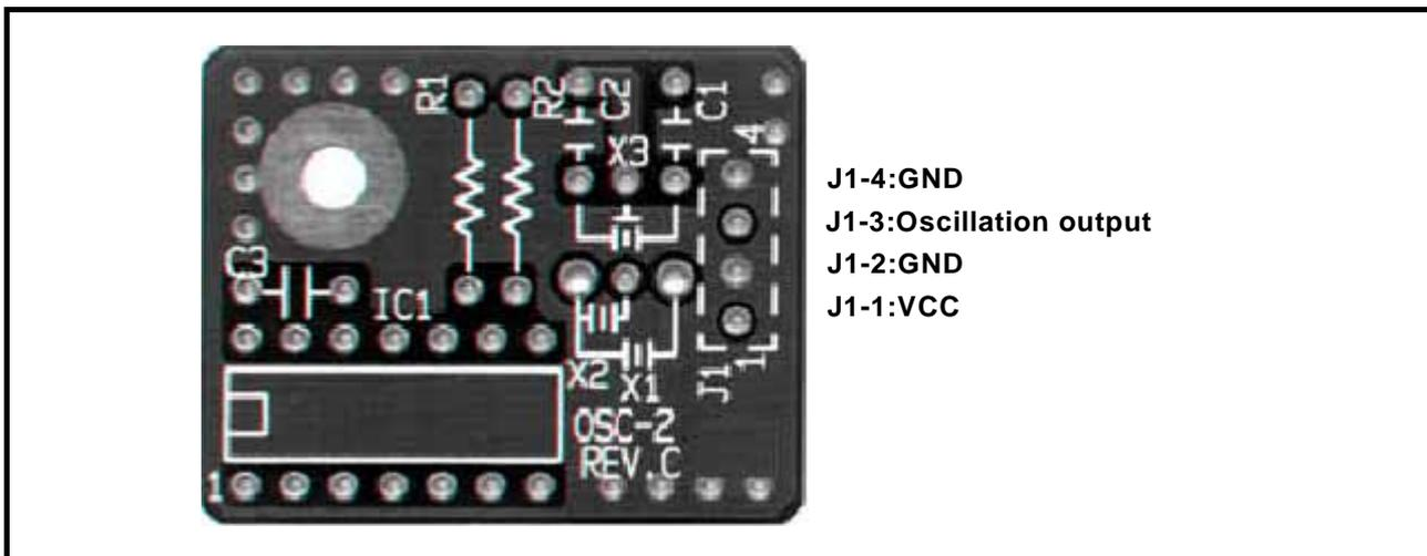
Figure 2.3 External view of the OSC-2 oscillator circuit board and its connector pin positions
