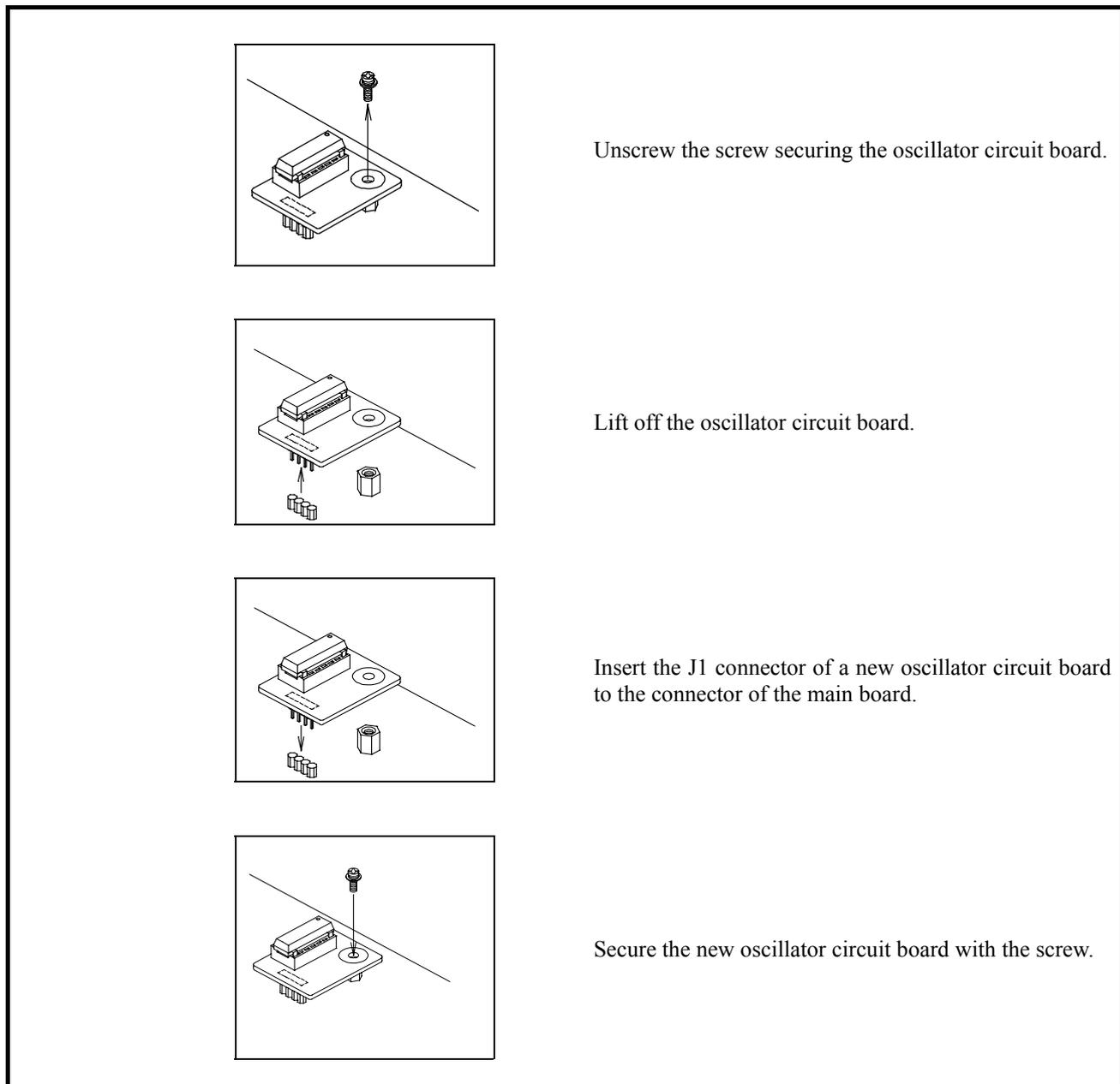
**Figure 2.5 Replacing oscillator circuit boards**
