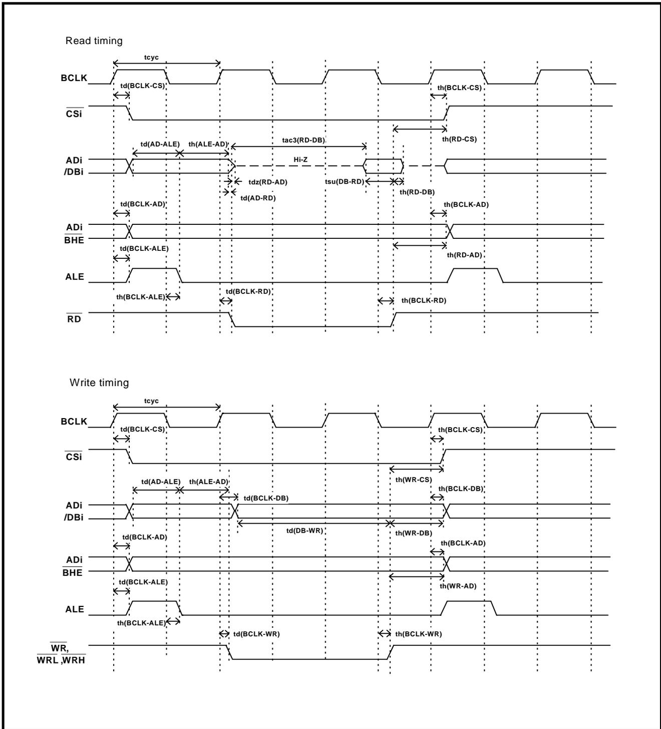
Figure 4.2 Memory expansion and microprocessor modes (2-wait, accessing external area, using multiplex bus)
