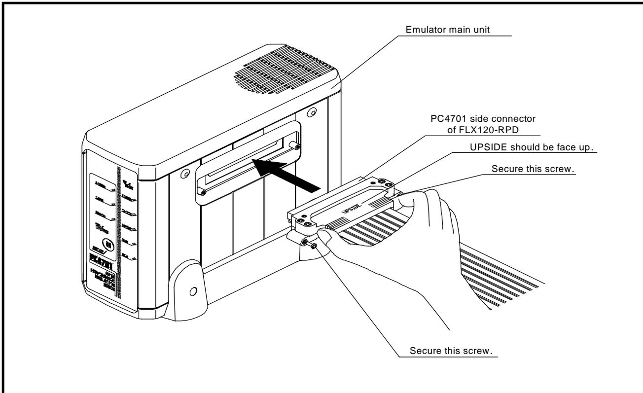
Figure 2.12 Connecting the cable to the PC4701
