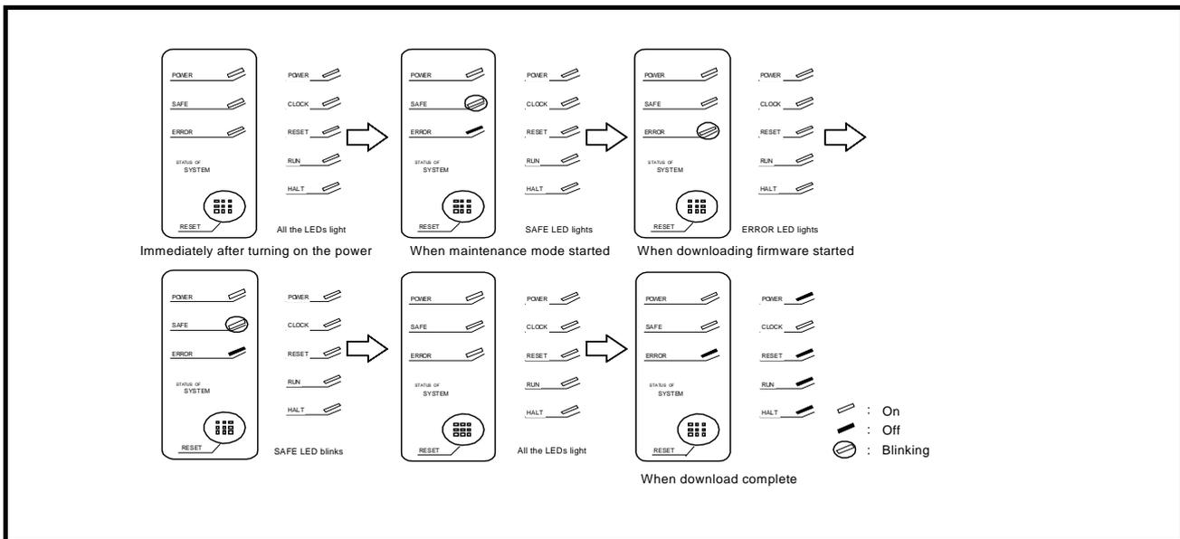
Figure 3.2 Downloading firmware in maintenance mode
