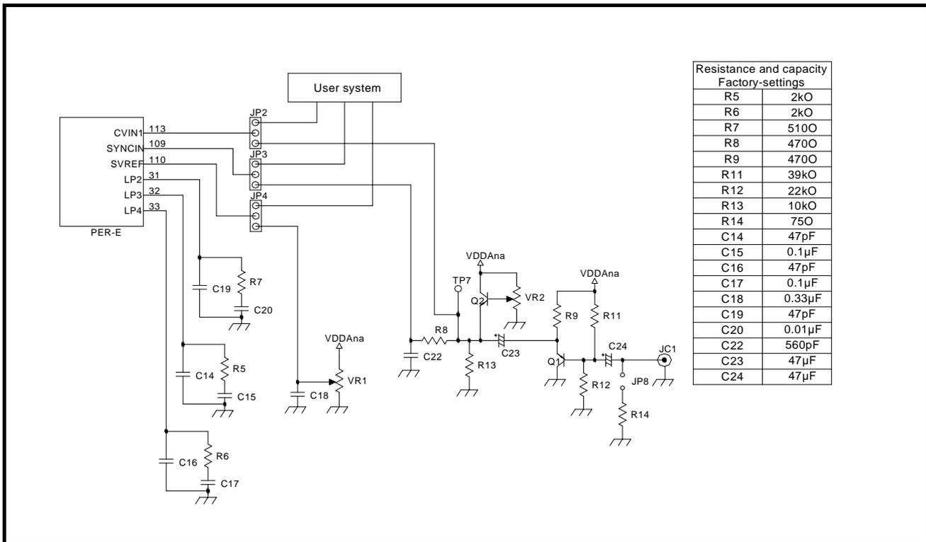
Figure 2.10 Connection diagram of circuits connected to the data slicer
