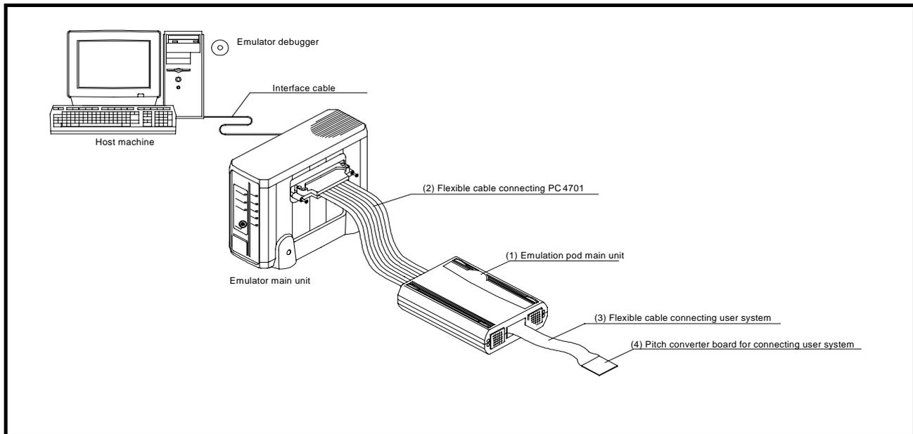
**Figure 1.1 System configuration**
