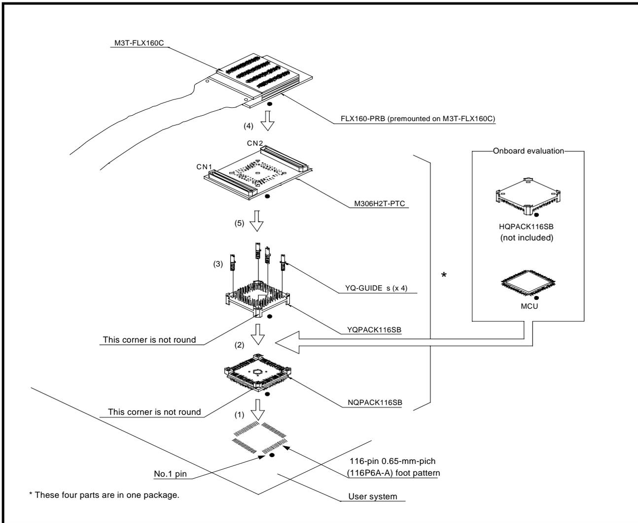
Figure 2.14 Connecting the user system
