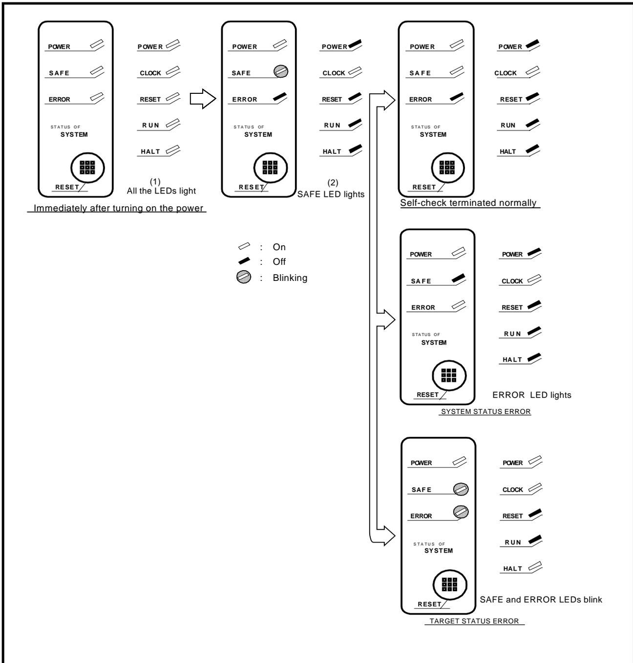
Figure 3.4 Self-check procedure
