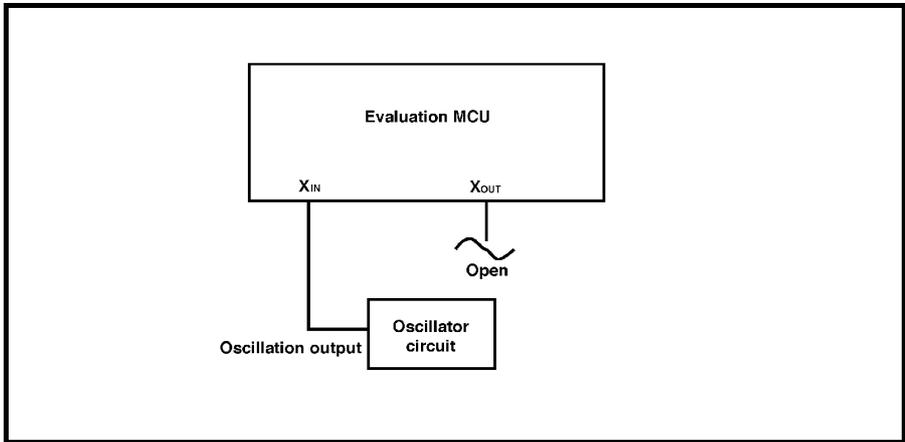
Figure 2.6 External oscillator circuit
