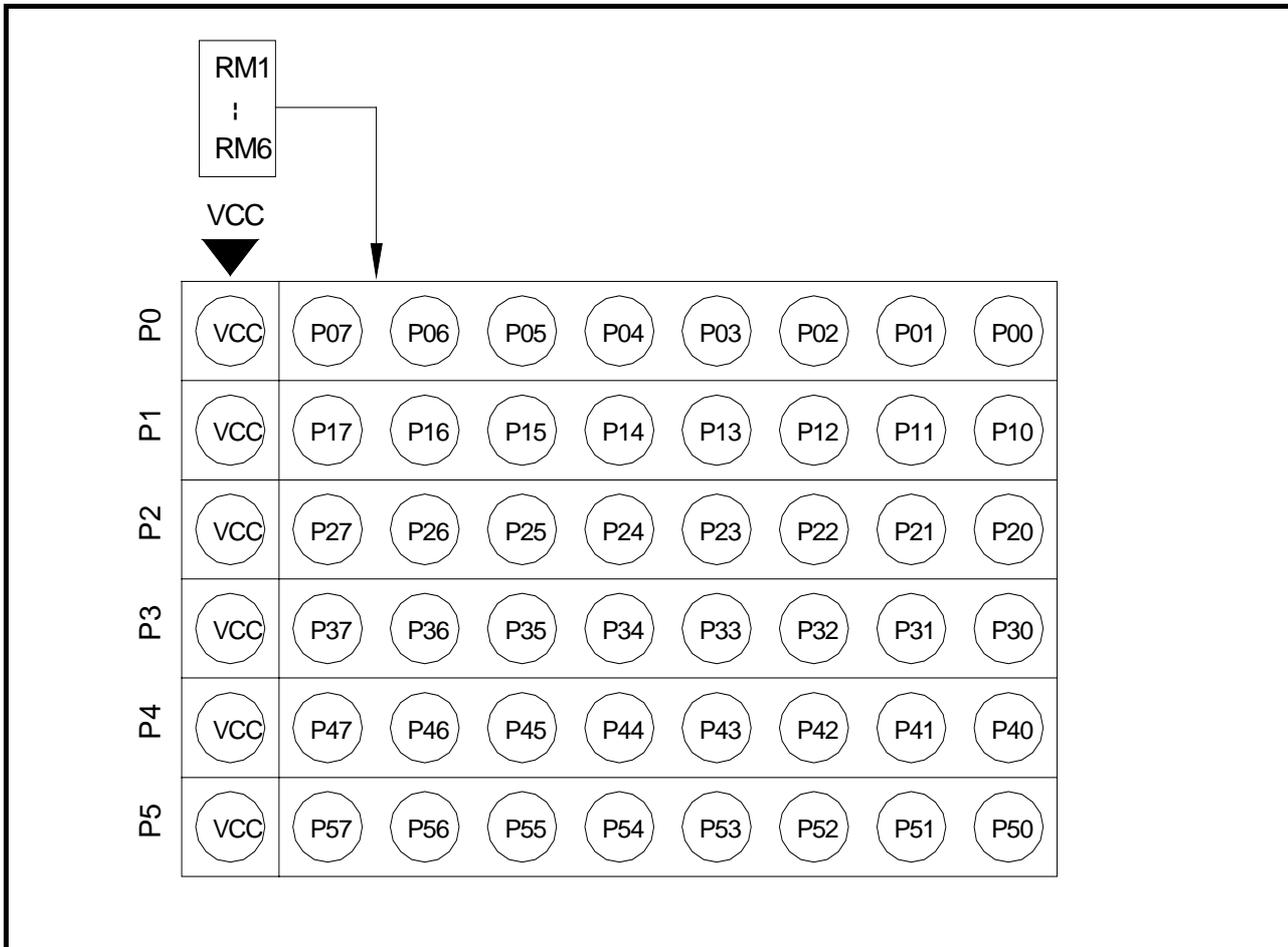
Figure 2.8 Position for mounting network resistors for pullup
