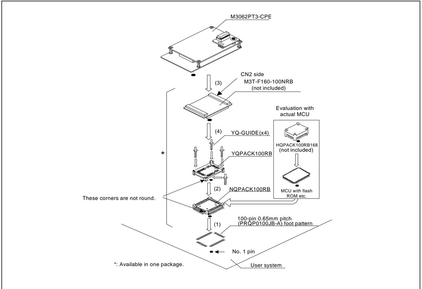
Figure 2.15 Connecting to a 100-pin 0.65mm pitch foot pattern (Part 1)
