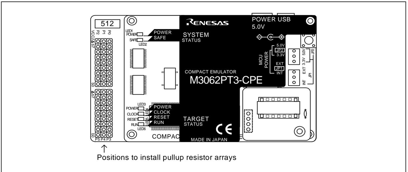
Figure 2.29 Positions of the pullup resistors
