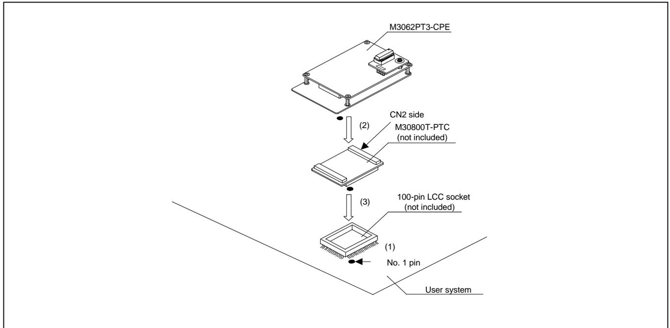
Figure 2.14 Connecting to a 100-pin LCC socket
