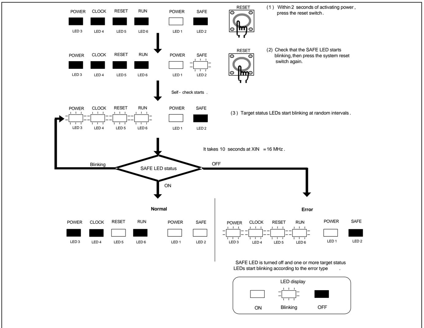
Figure 2.11 Self-check procedure
