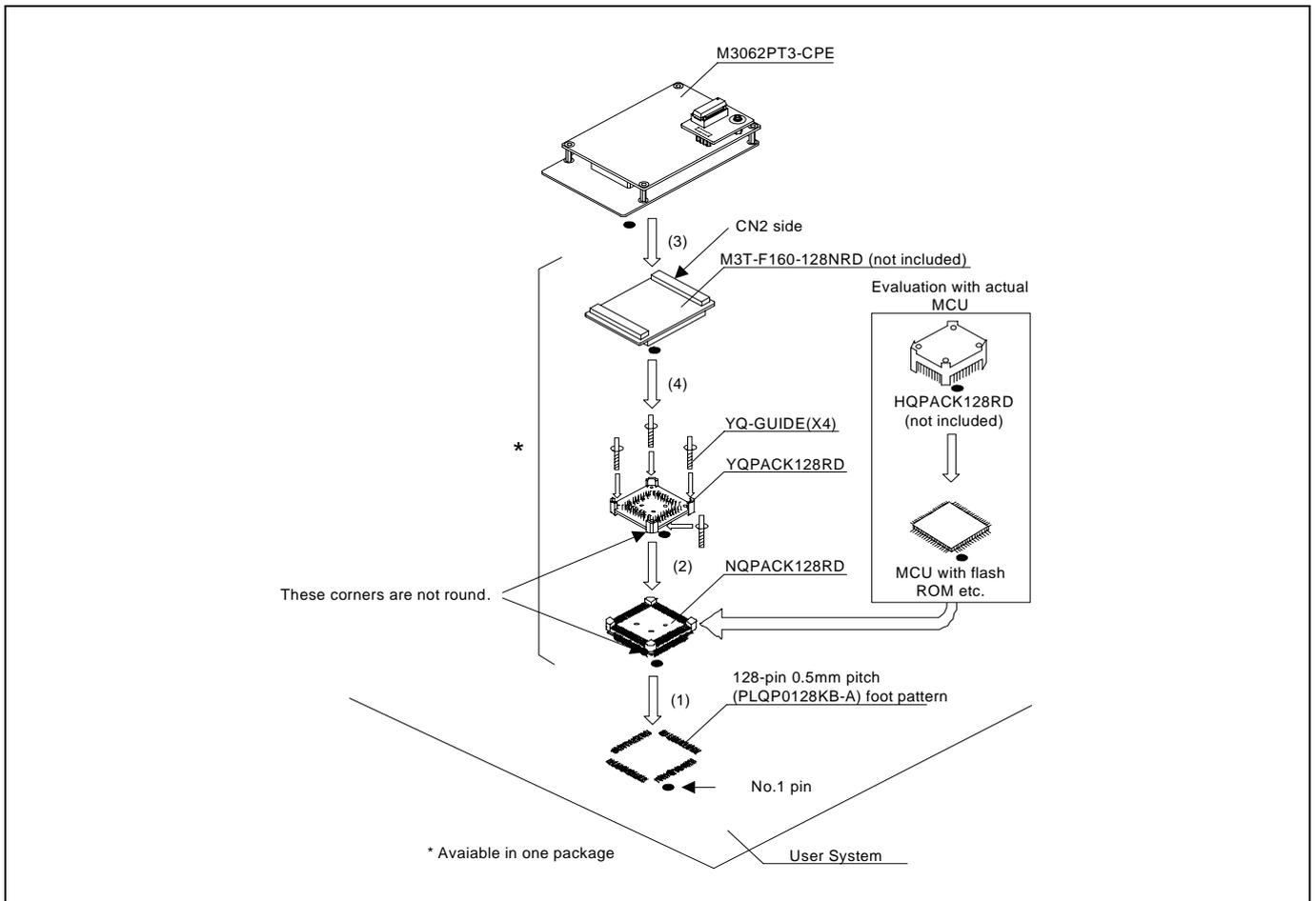
Figure 2.22 Connecting to a 128-pin 0.5mm pitch foot pattern
