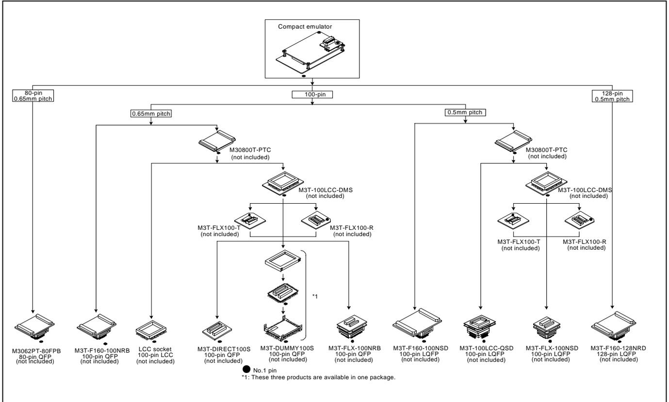
Figure 2.12 Connection of the M3062PT3-CPE and user system
