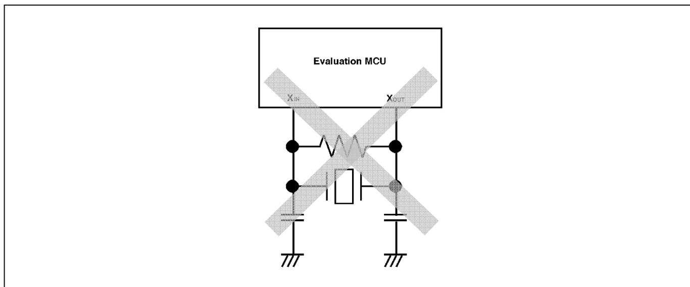
Figure 2.27 Circuit in which oscillation does not occur
