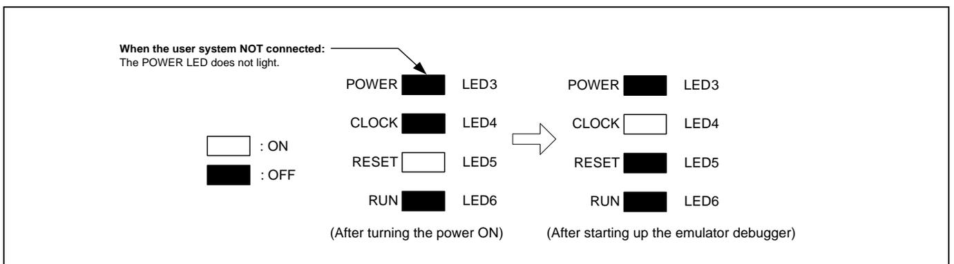
Figure 2.9 Target status LEDs display when the emulator starts up normally (when user system not connected)
