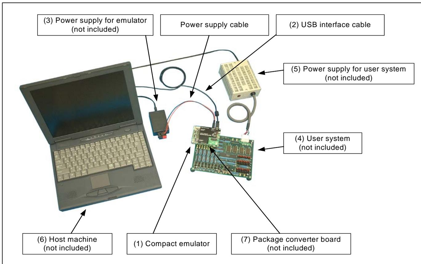
Figure 1.1 System configuration
