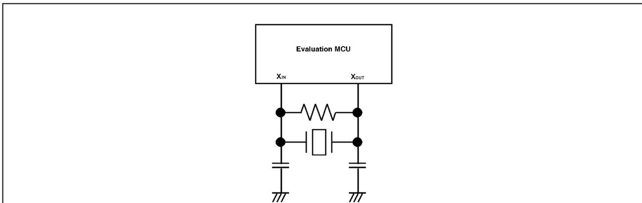
Figure 2.26 Circuit in which oscillation does not occur
