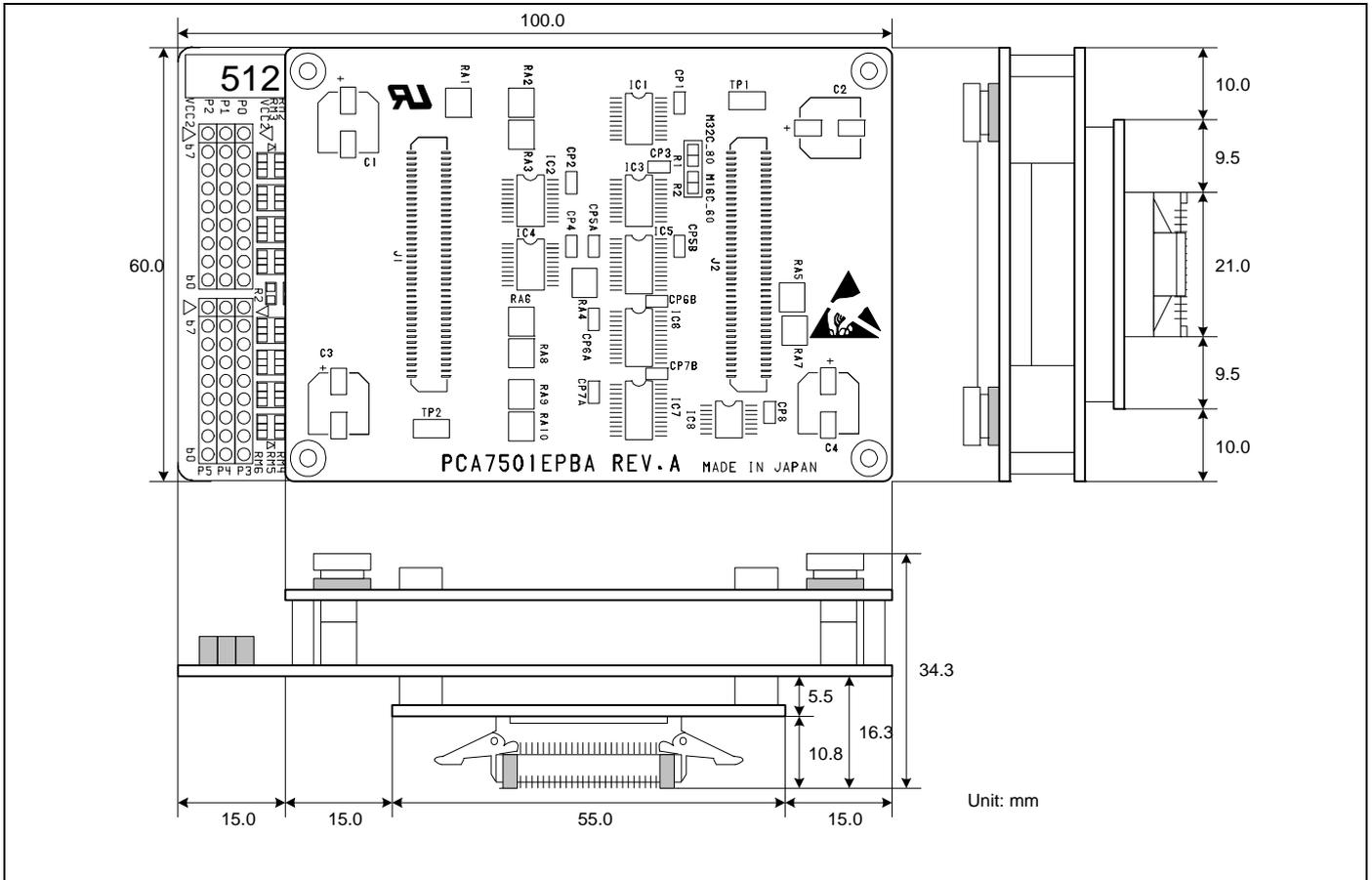
Figure 4.8 External dimensions of the emulation probe
