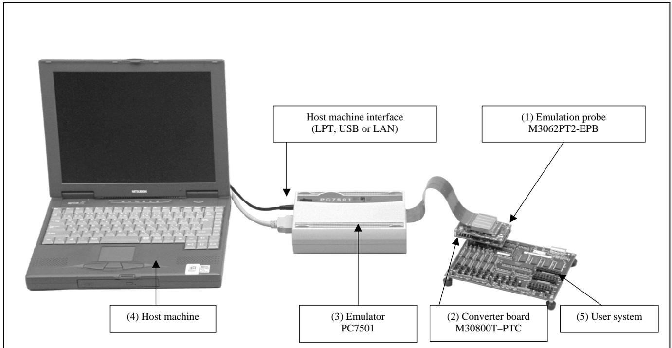
Figure 1.2 System configuration
