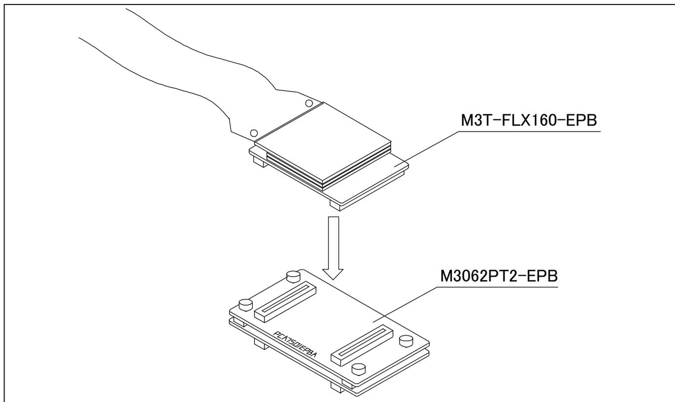
Figure 2.3 Connecting the PC7501 and emulation probe
