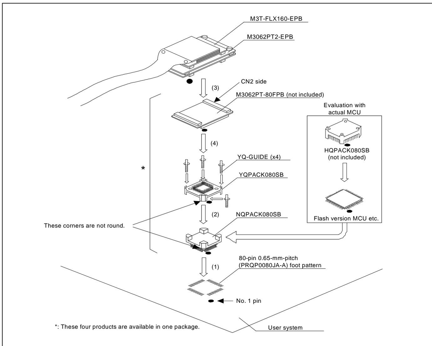
Figure 2.8 Connecting to an 80-pin 0.65-mm-pitch foot pattern
