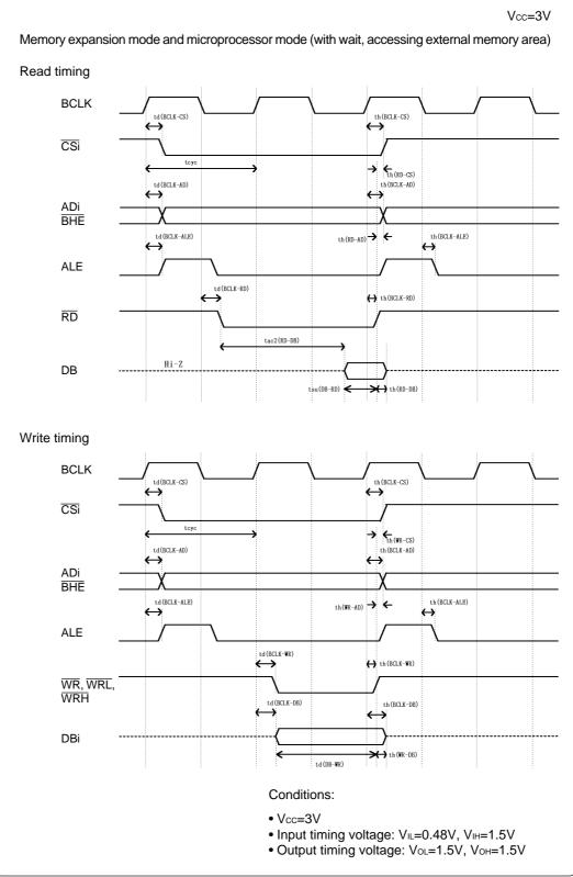
Figure 5.2 Memory expansion mode and microprocessor mode (with wait)
