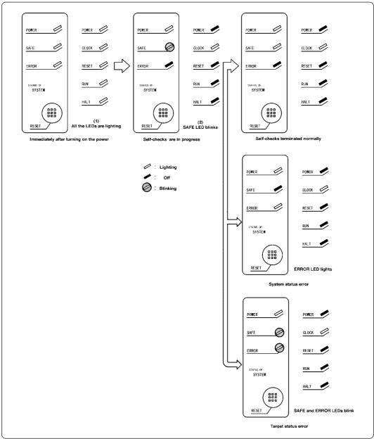
Figure 4.4 Self-check procedure
