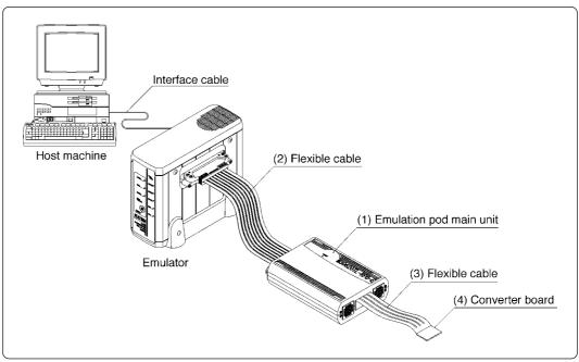
Figure 2.1 System configuration
