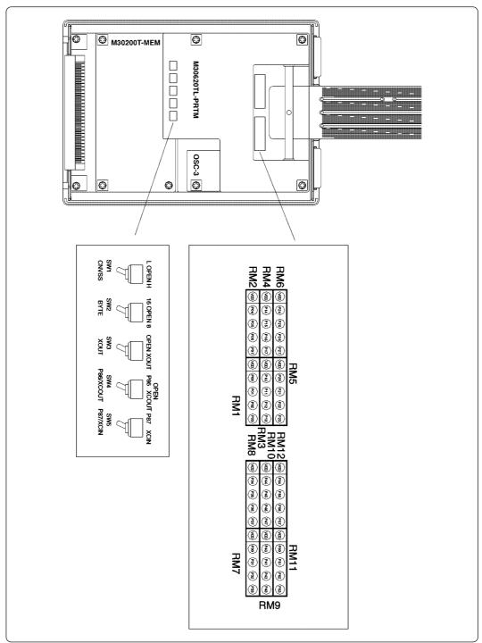
Figure 3.2 Positions of switches and their factory-settings
