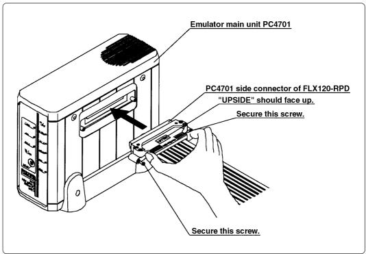
Figure 3.9 Connecting PC4701 and FLX120-RPD
