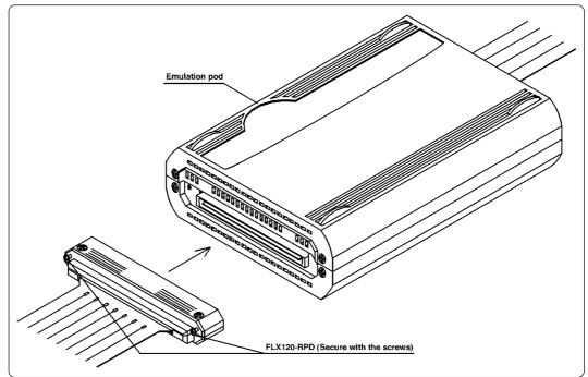
Figure 3.10 Connecting FLX120-RPD and emulation pod
