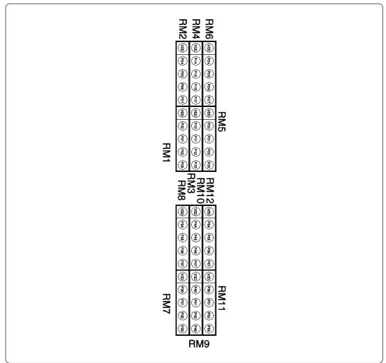
Figure 3.3 Positions for installing the pullup resistor
