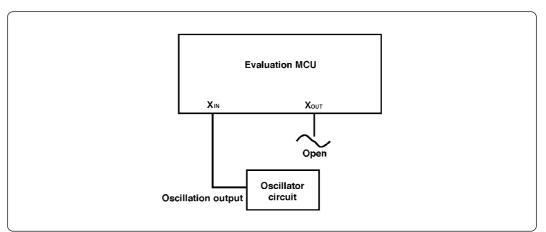
Figure 3.4 External oscillator circuit
