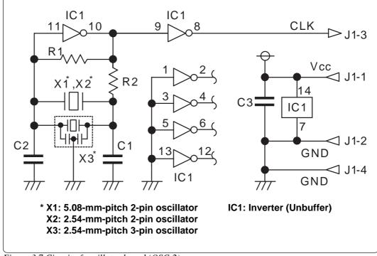
Figure 3.7 Circuit of oscillator board (OSC-2)
