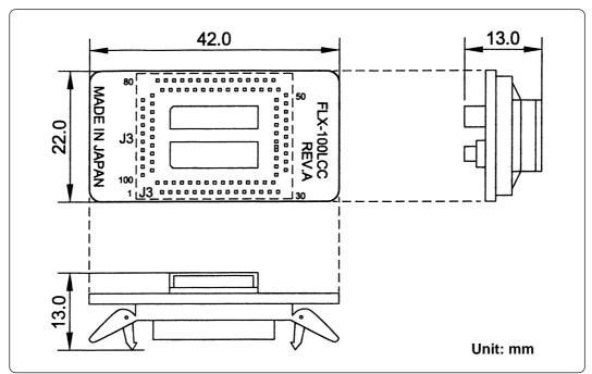
Figure 5.8 External dimensions of converter board (FLX-100LCC)
