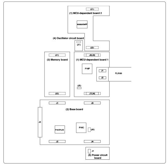
Figure 2.2 Internal view of emulation pod
