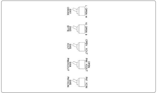
*Figure 4.3 Switch settings when running self-checks (factory-settings)*
