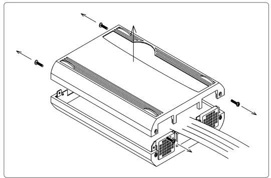
Figure 3.1 Removing the upper cover
