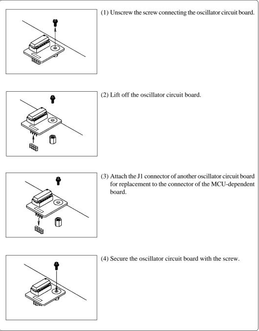
Figure 3.8 Replacing the oscillator circuit boards
