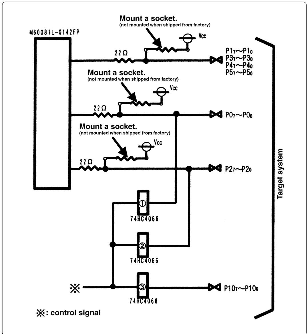
Figure 5.12 Connection diagram 2
