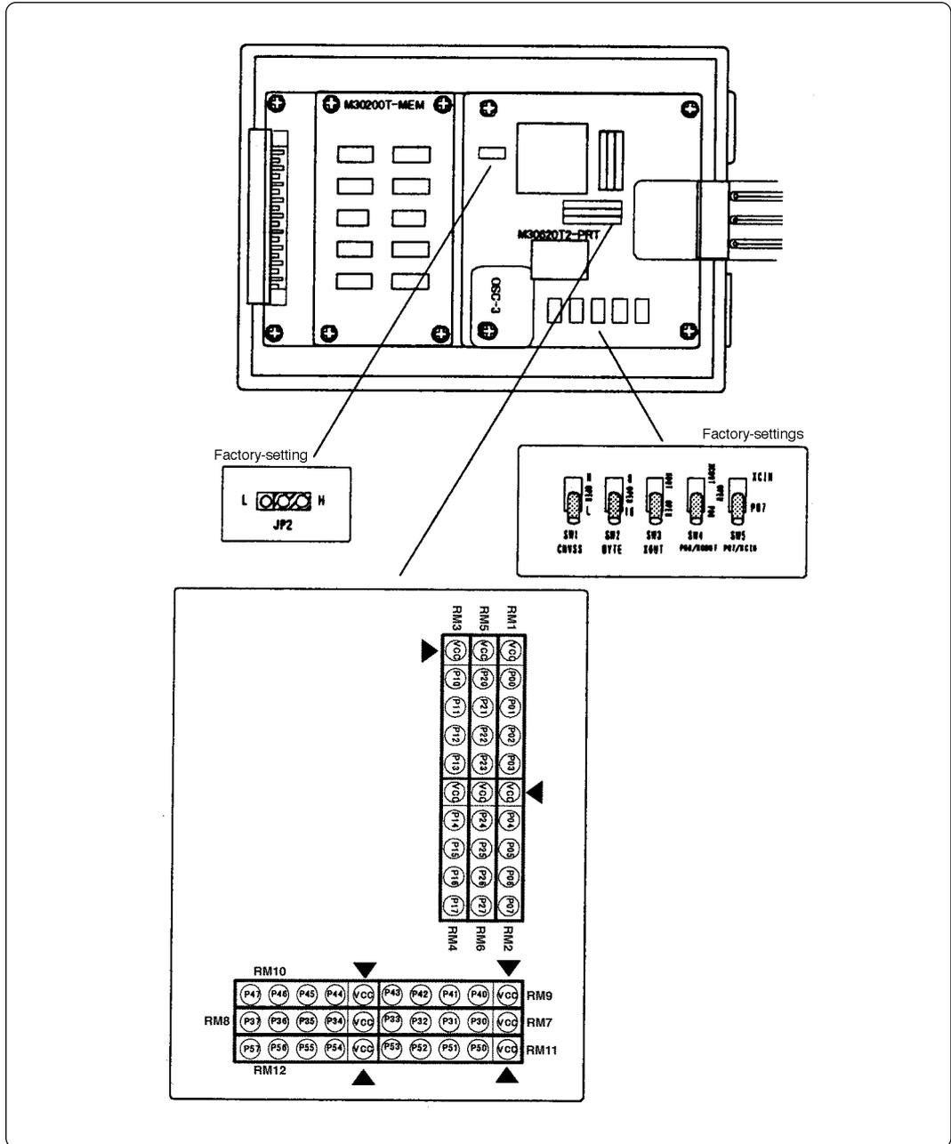
Figure 3.2 Positions of switches and their factory-settings
