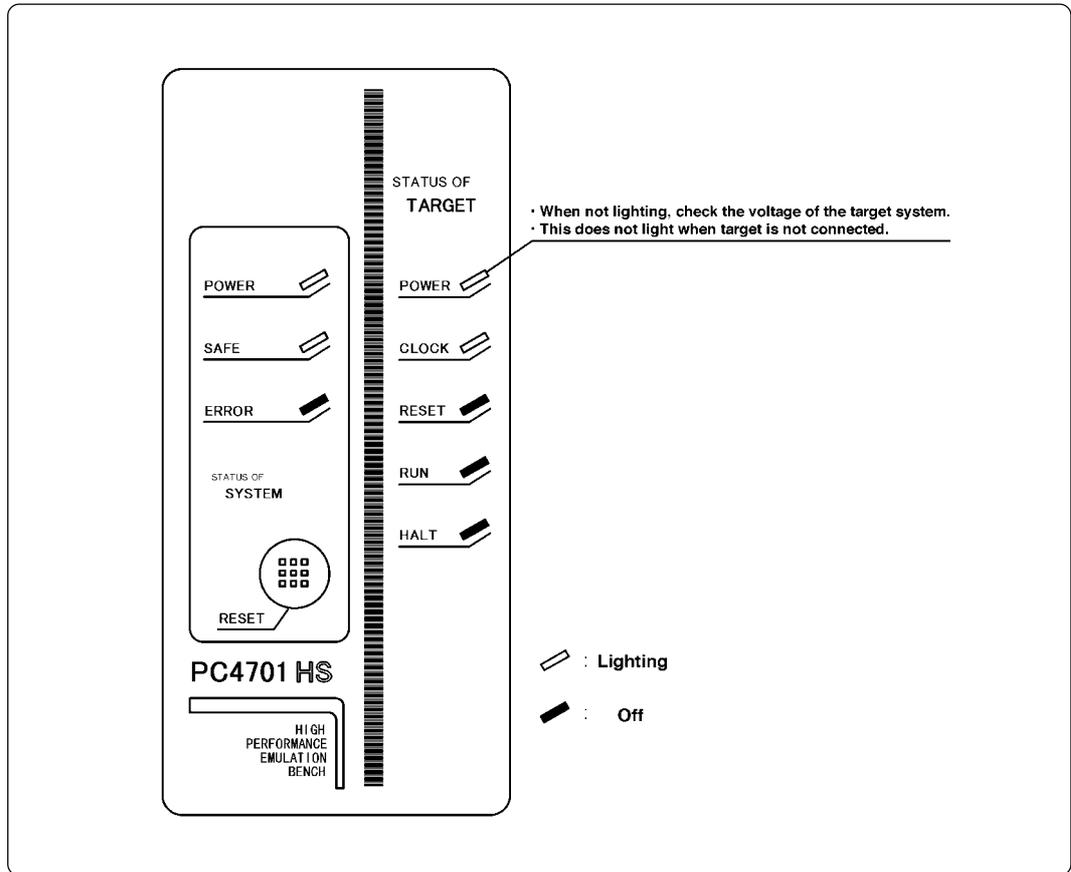
Figure 4.1 LED display when the power turned on
