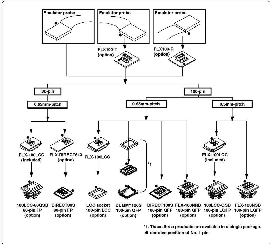
Figure 3.11 Connecting emulation pod and target systems
