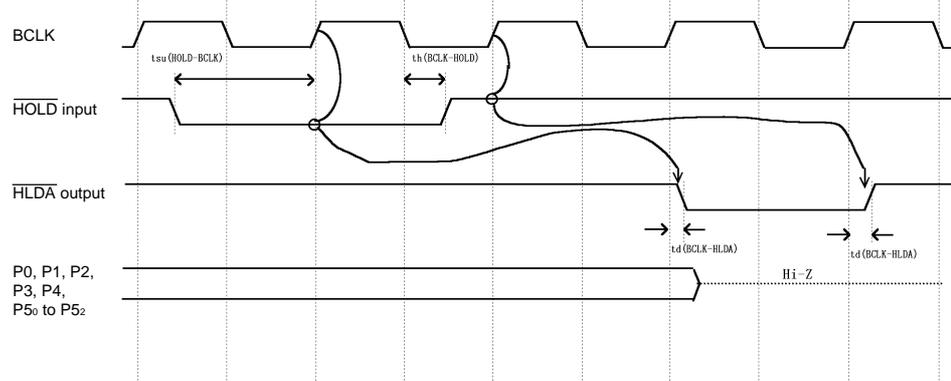
Note 1. P0<sub>0</sub> to P5<sub>2</sub> will be high-impedance status regardless of the input level of BYTE pin and ports P4<sub>0</sub> to P4<sub>3</sub> function selection bit (PM06) of the processor mode register 0.
