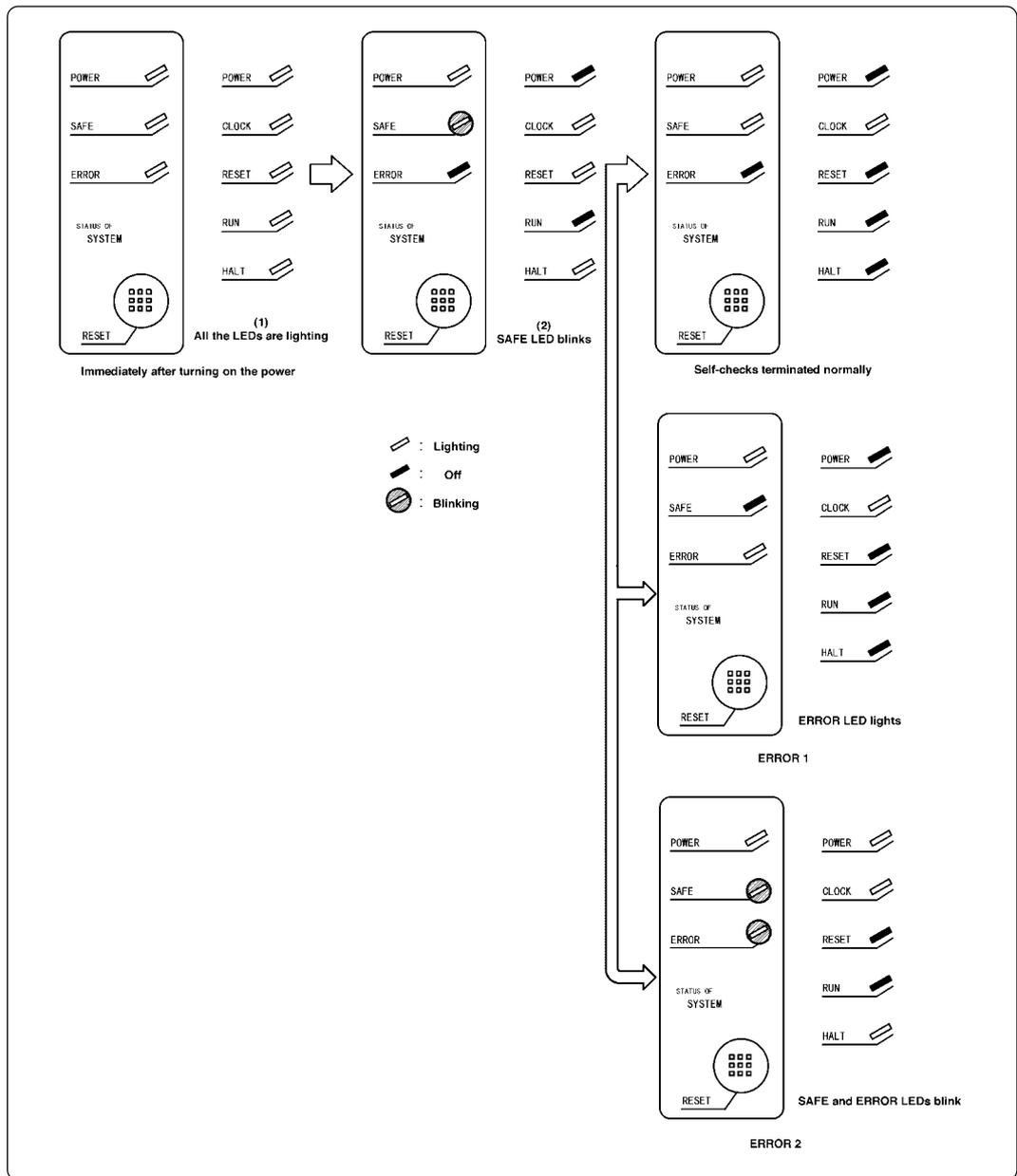
Figure 4.4 Self-check procedure
