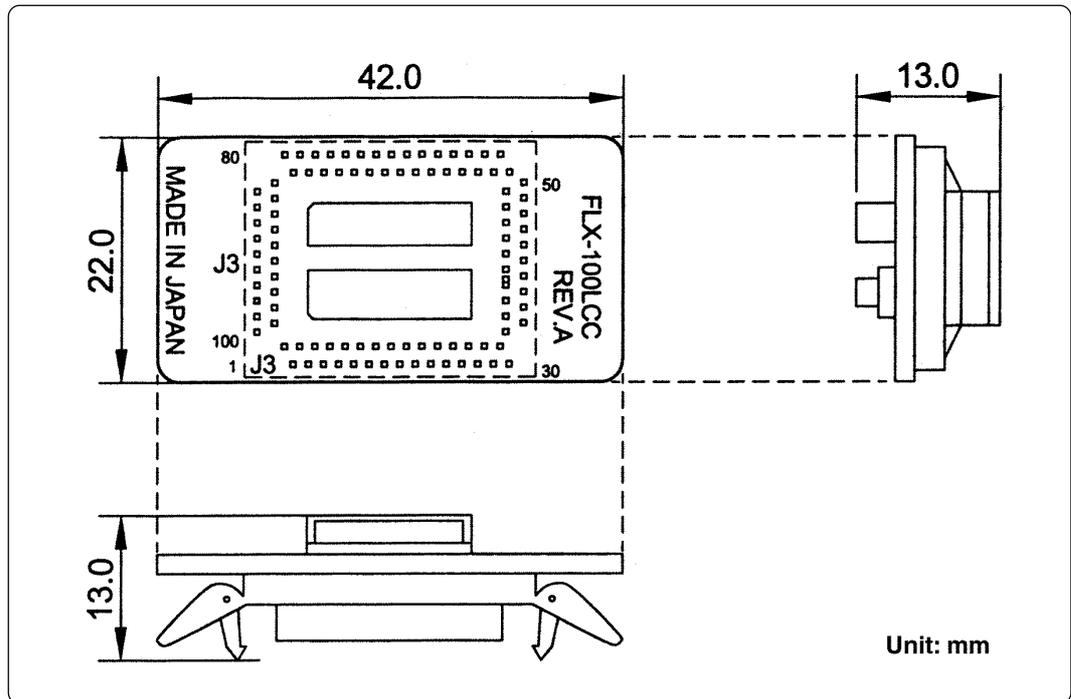
Figure 5.14 External dimensions of pitch converter board (FLX-100LCC)
