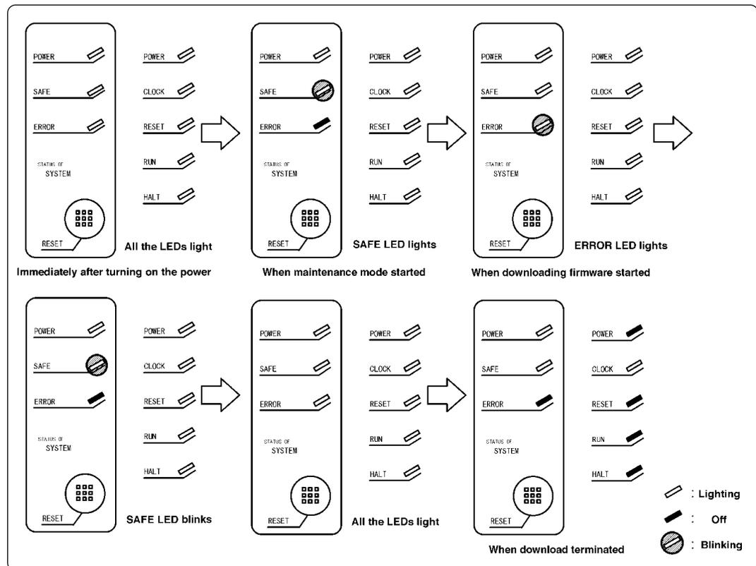
Figure 4.2 Downloading firmware in the maintenance mode
