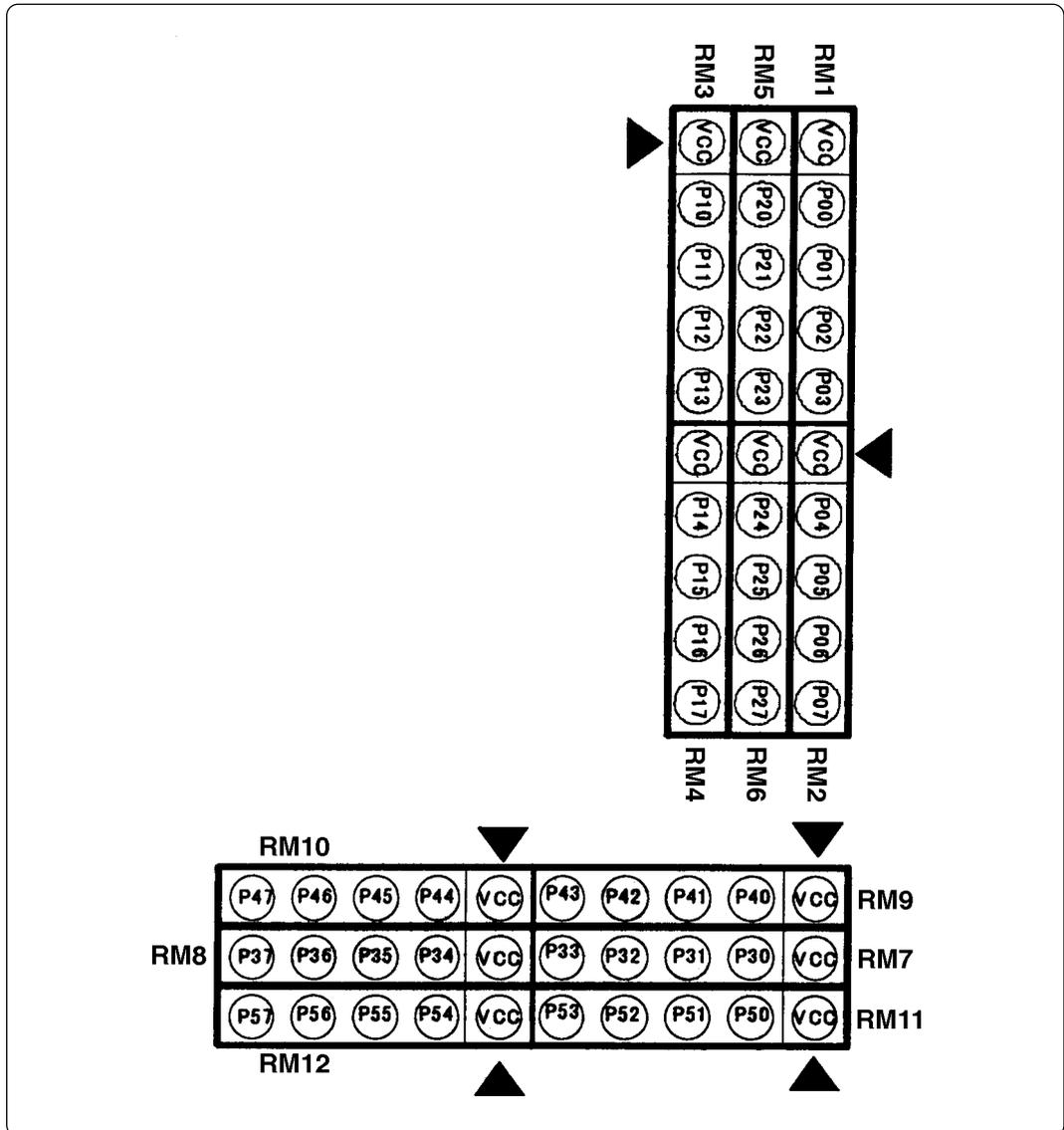
Figure 3.3 Positions for installing the pullup resistor
