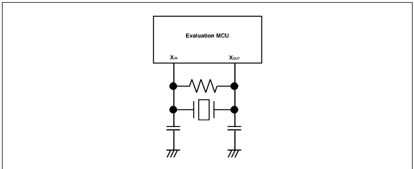
Figure 2.20 Circuit in which oscillation does not occur
