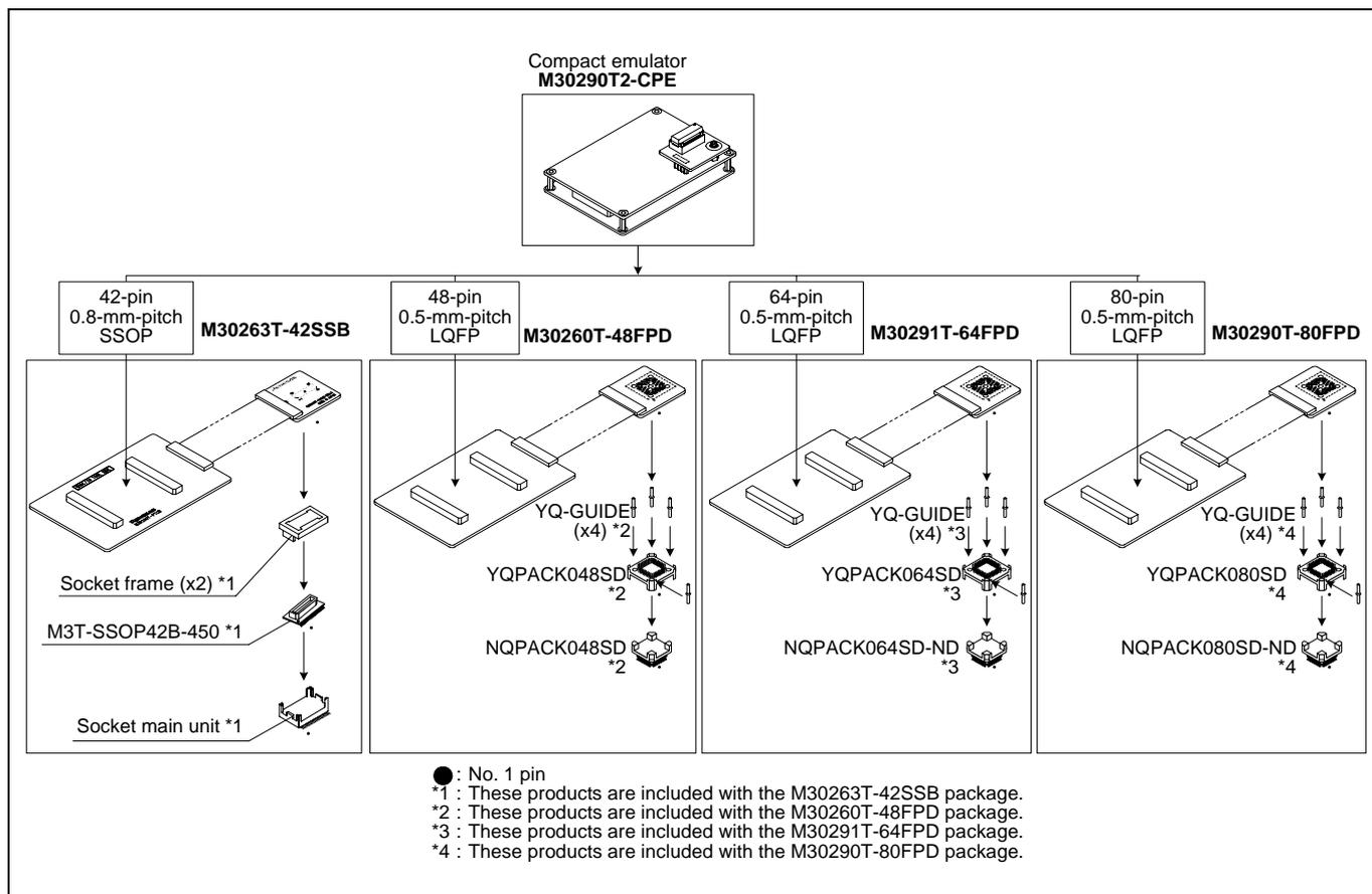
Figure 2.11 Connection of the M30290T2-CPE and user system
