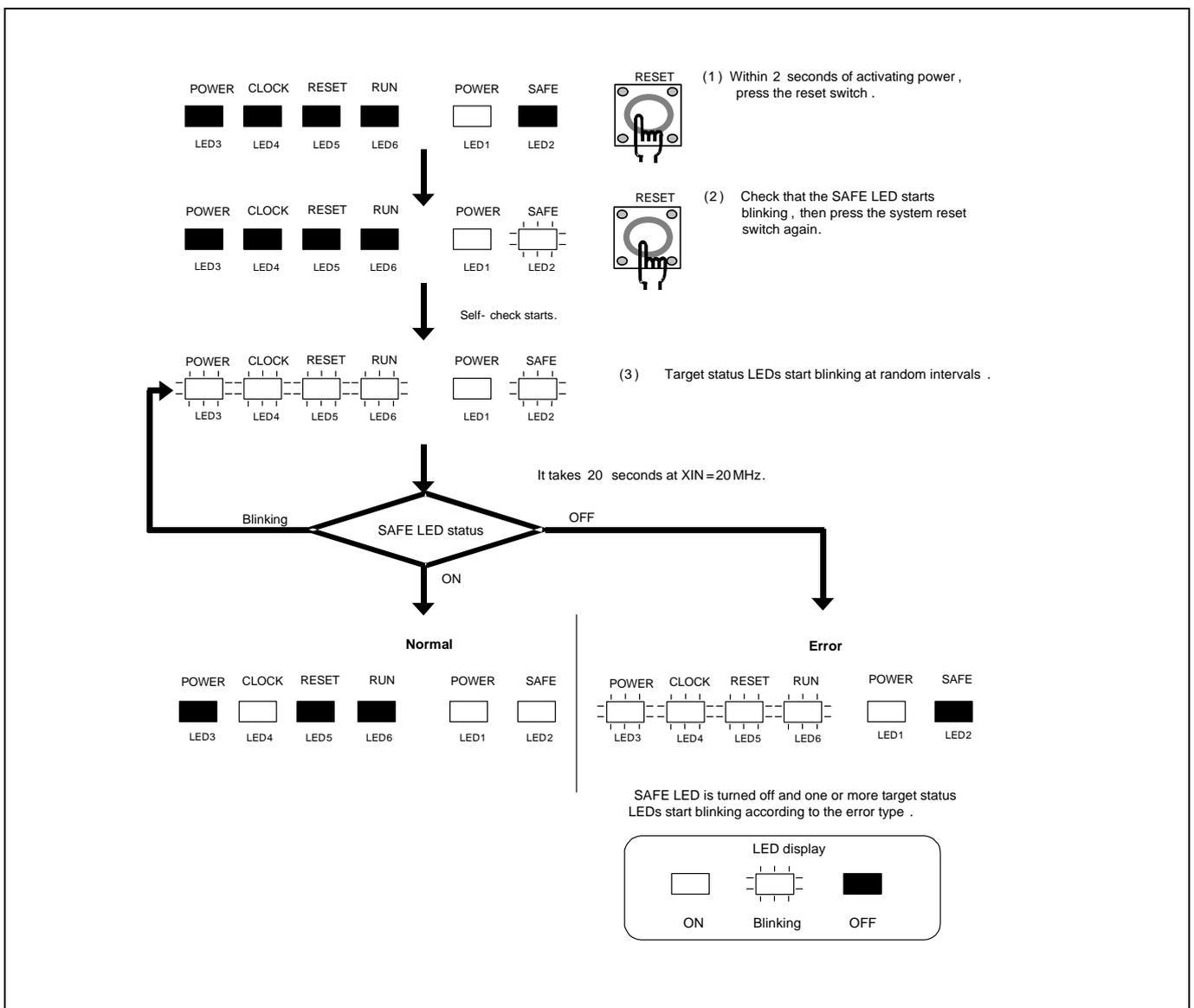
Figure 2.10 Self-check procedure
