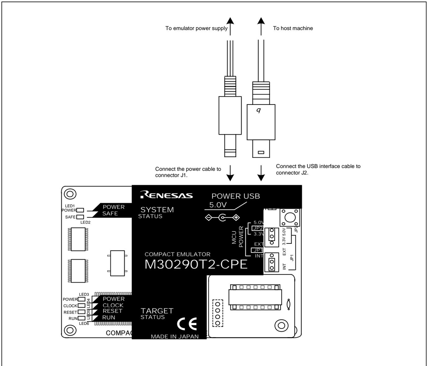
Figure 2.5 Connecting the emulator system
