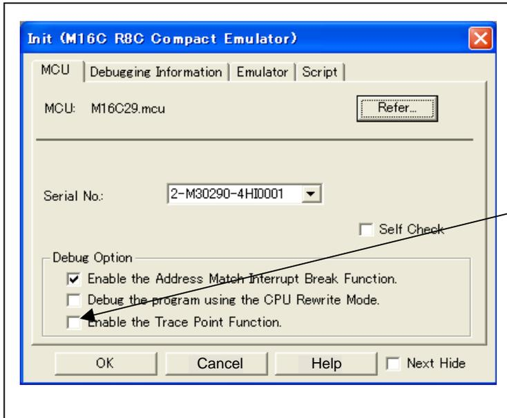
**Using or not using the trace point function**
