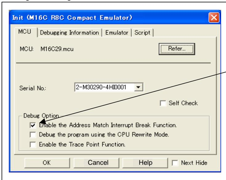
**Using or not using the address match break function**
