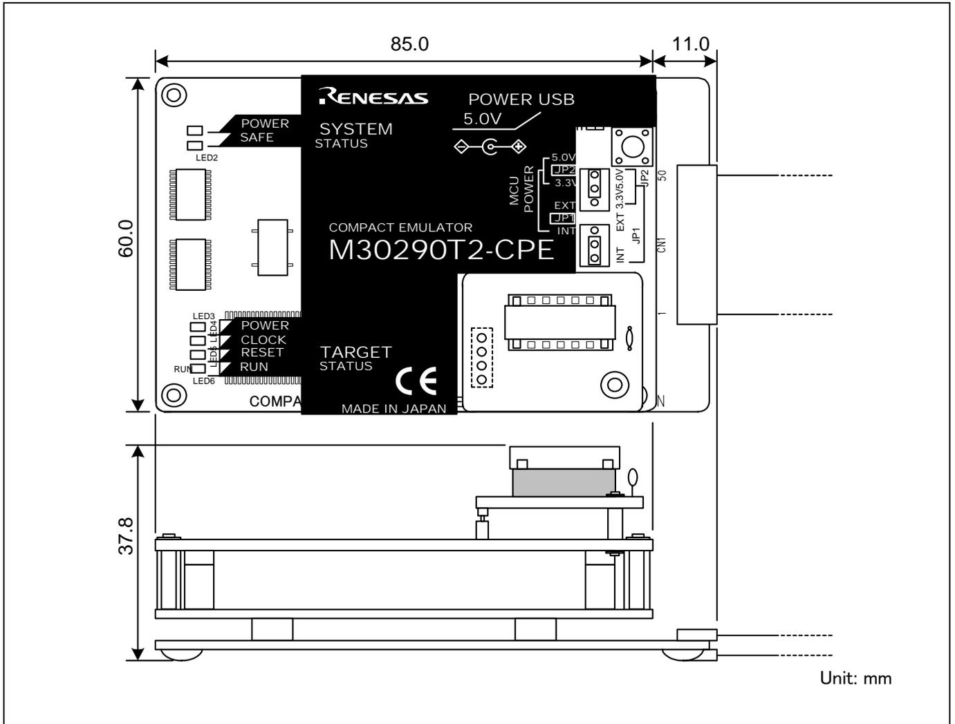
Figure 4.2 External dimensions of the compact emulator
