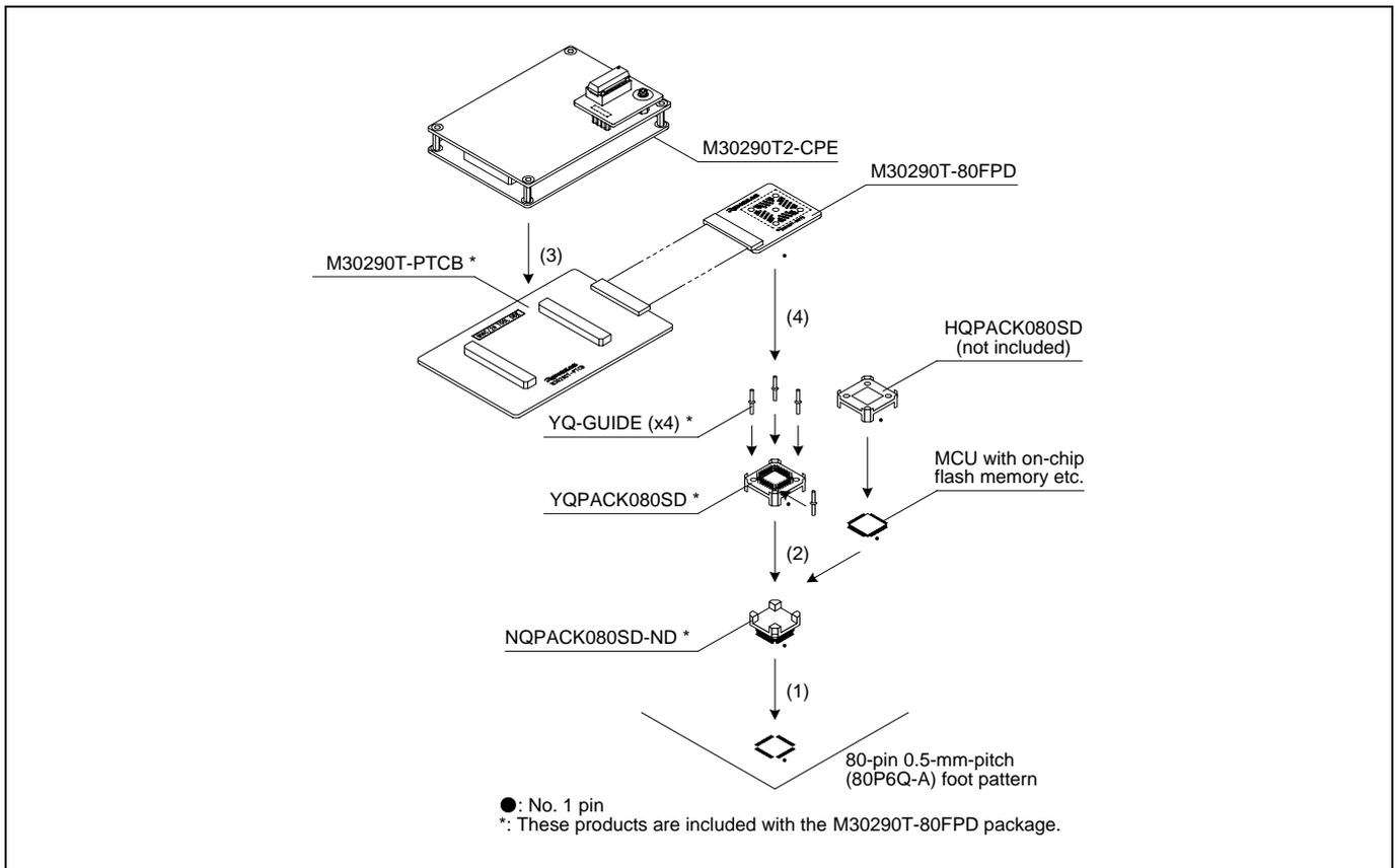
Figure 2.15 Connecting to an 80-pin 0.5-mm-pitch foot pattern
