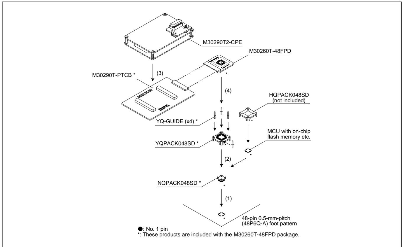
Figure 2.13 Connecting to a 48-pin 0.5-mm-pitch foot pattern
