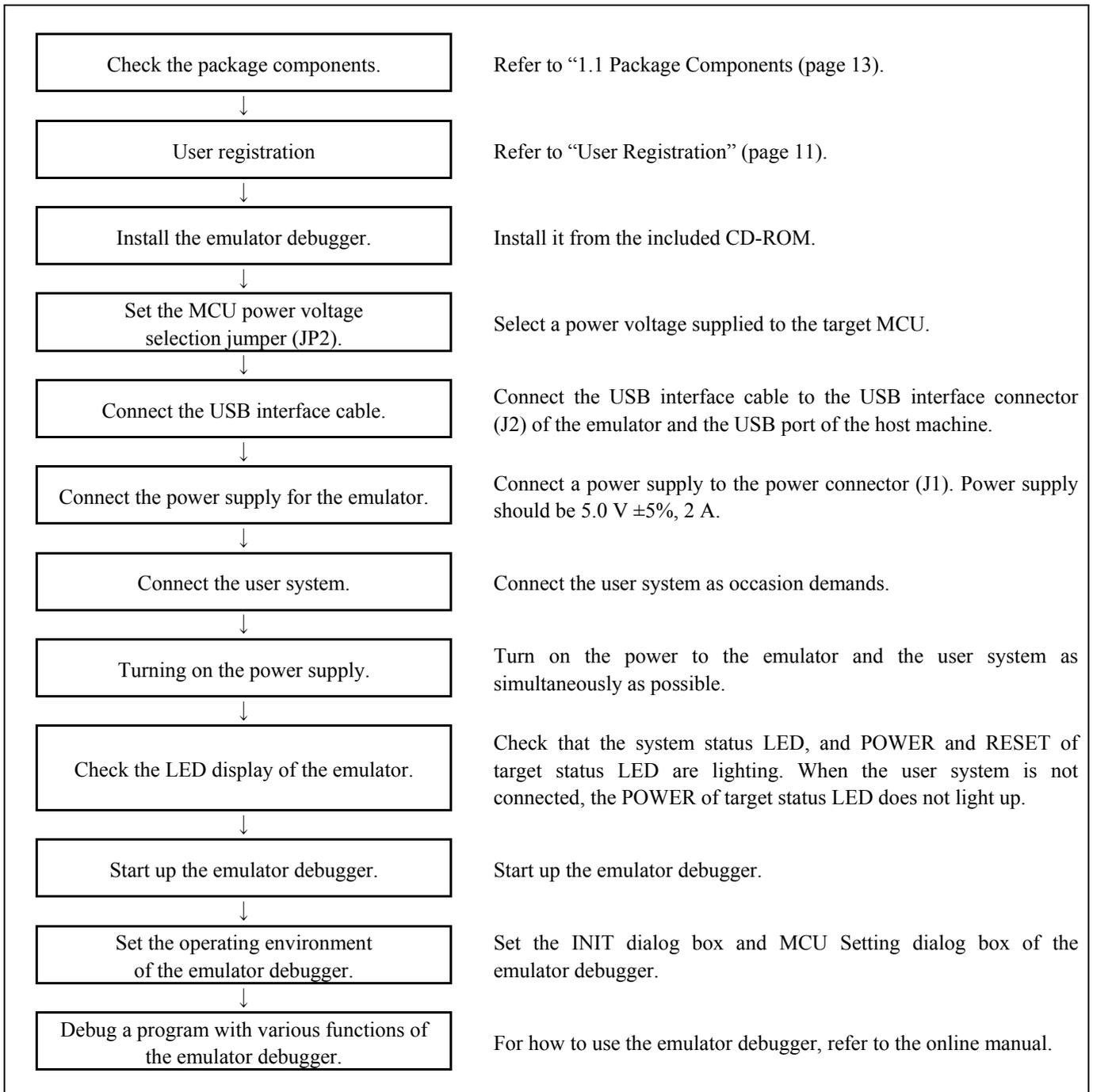
Figure 2.1 Flowchart of starting up the emulator
