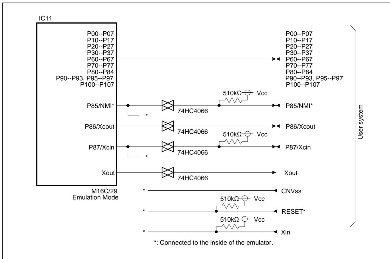
Figure 4.1 Connection diagram
