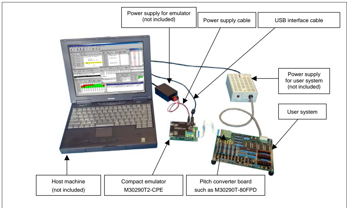
Figure 1.1 System configuration
