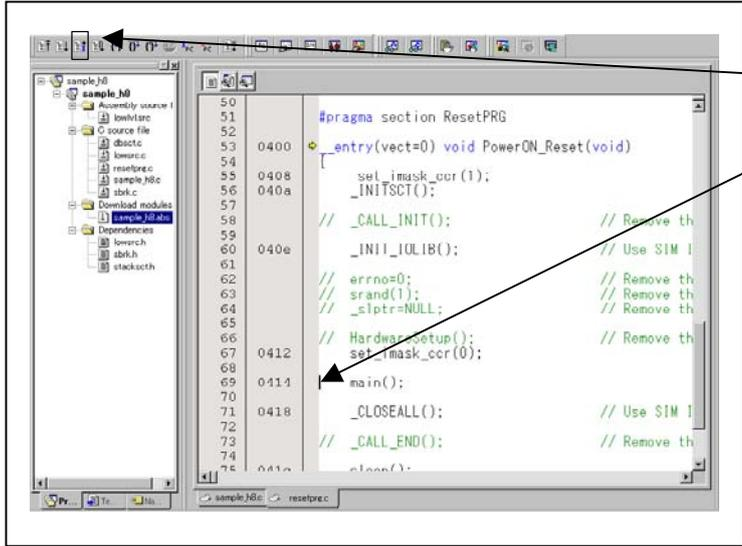
Setup procedure for running the program up to the cursor position
