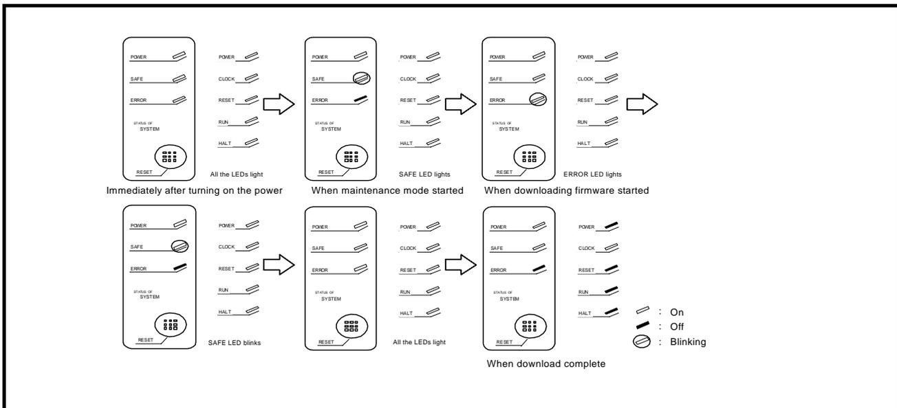
Figure 3.2 Downloading firmware in maintenance mode
