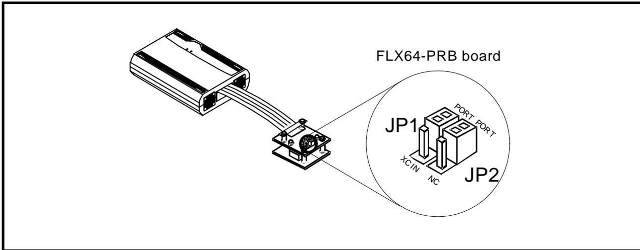
Figure 2.3 Positions of the switches and their factory-settings
