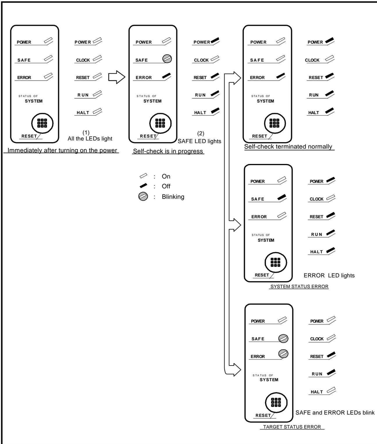
Figure 3.5 Self-check procedure
