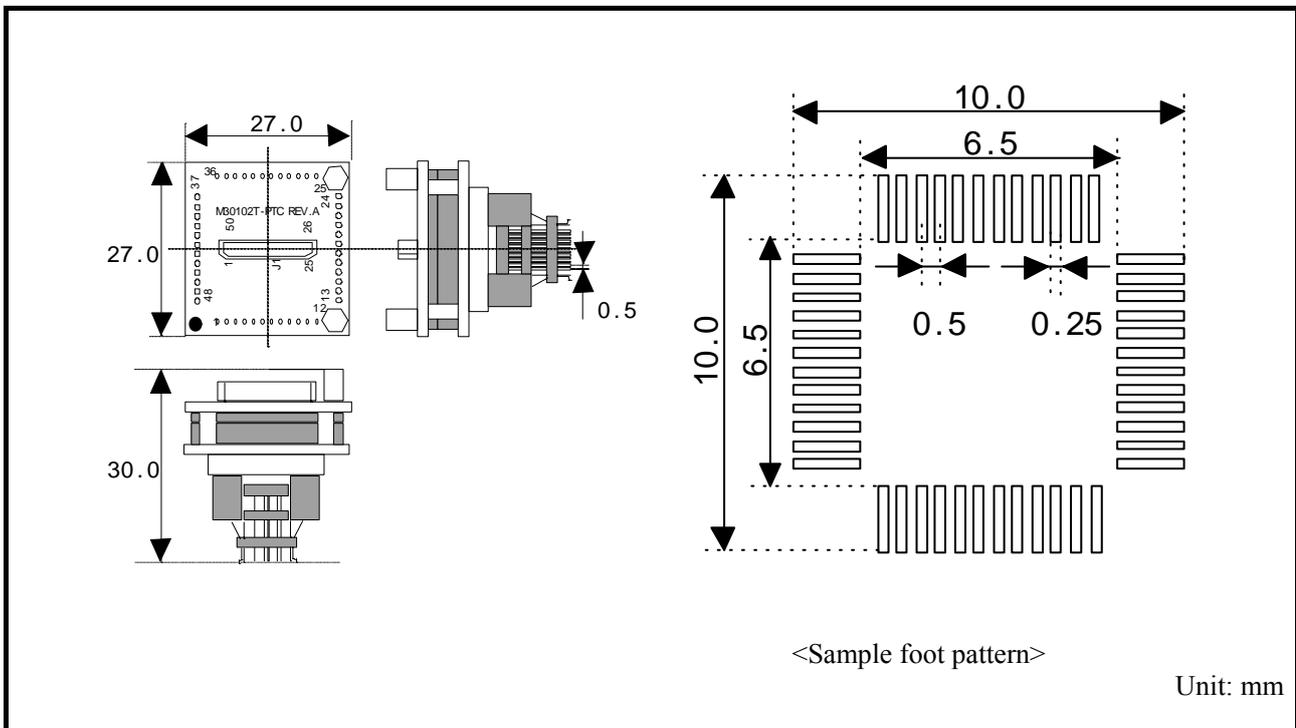
Figure 4.2 External dimensions of the converter board M30102T-PTC and a sample foot pattern
