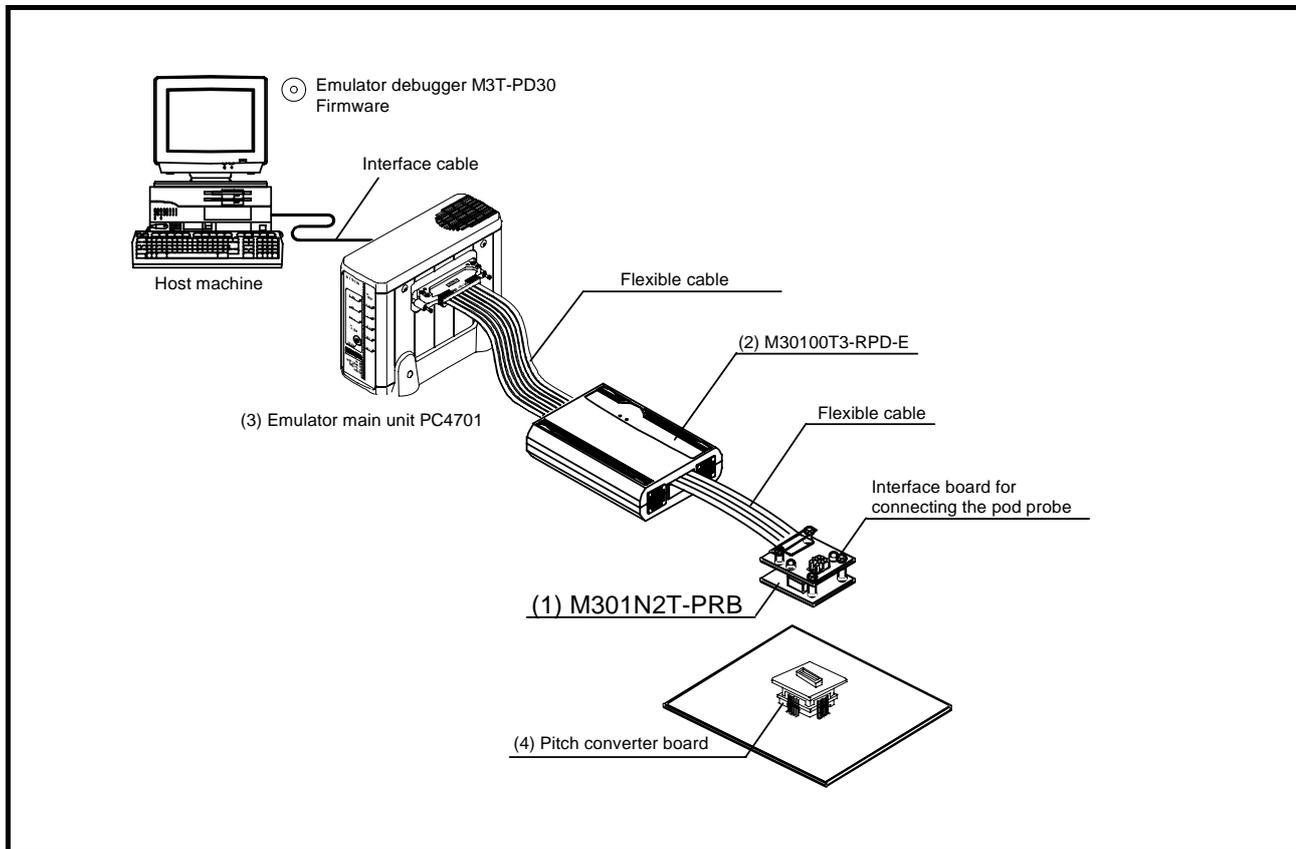
**Figure 1.1 System configuration**
