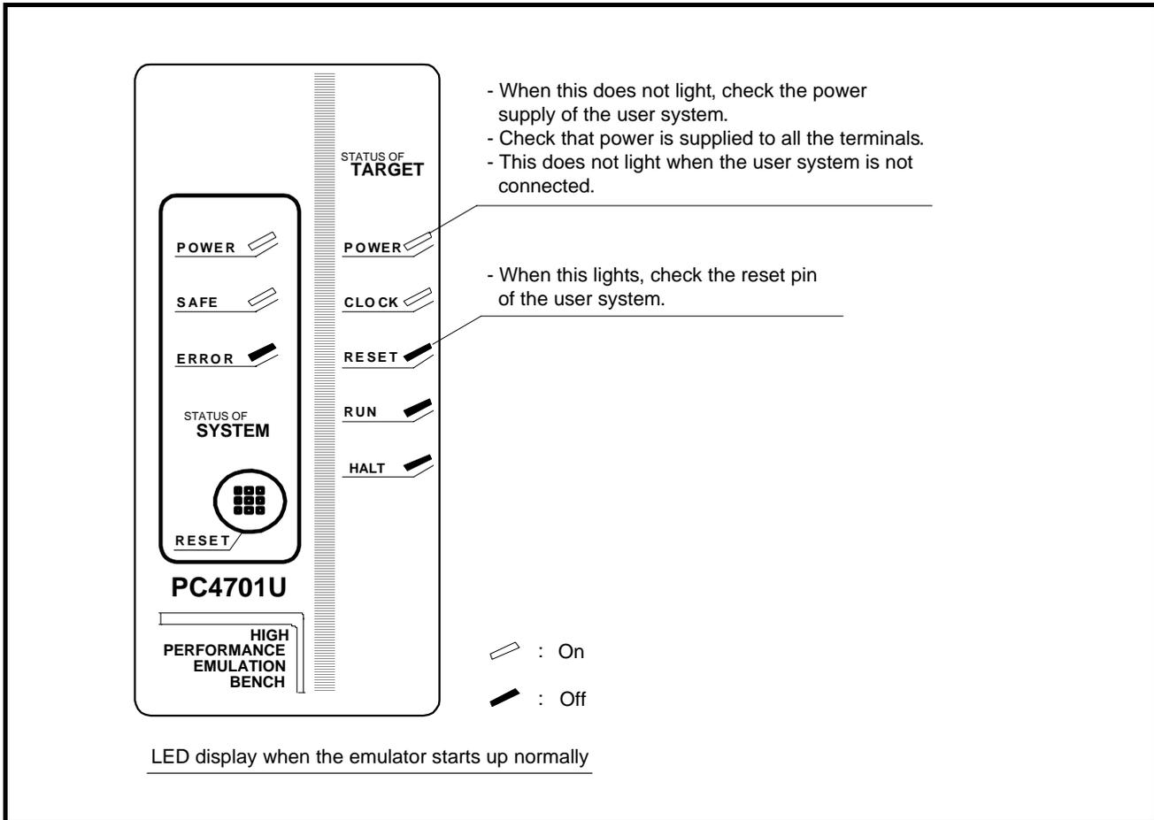
Figure 3.1 LED display when the power turned on
