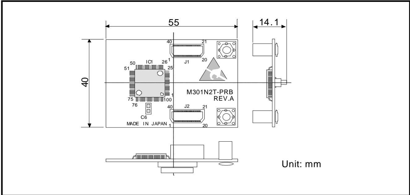
Figure 4.1 External dimensions of the M301N2T-PRB
