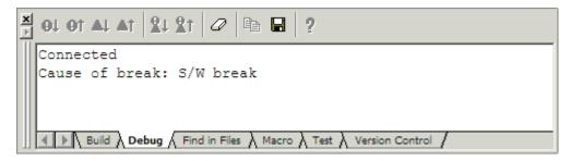
The user can also see the cause of the break that occurred last time in the [Status] window. Select [Status] from the [CPU] submenu of the [View] menu. After the [Status] window is displayed, open the [Platform] sheet, and check the Status of Cause of last break.
