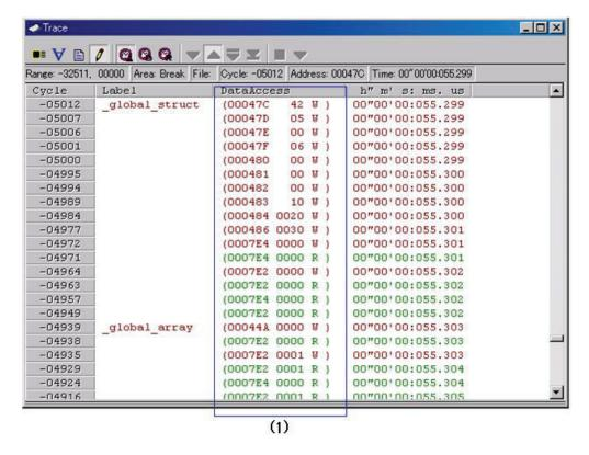
Data access display area: Shows data access information. If the information displayed here is "000400 1234 W," for example, it means that data "1234H" was written to the address 000400H in 2-byte width.
