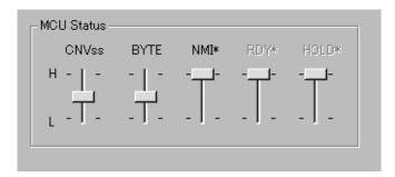
If the slider is at the middle position, it means that the value is indeterminate.
