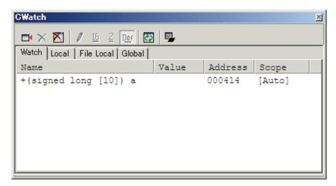
The user can click mark '+' at the left side of array a in the [C Watch] window to watch all the elements.
