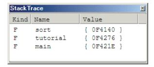
The upper figure shows that the position of the program counter is currently at the selected line of the sort() function, and that the sort() function is called from the tutorial() function.
