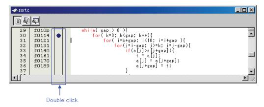
You can delete the break point by double-clicking again in the break point setting area ("Address Match Interrupt Break" column).
