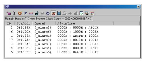
When the realtime OS is MRxx conformed to uITRON specifications V.3.0, the following data is displayed in the status bar.
