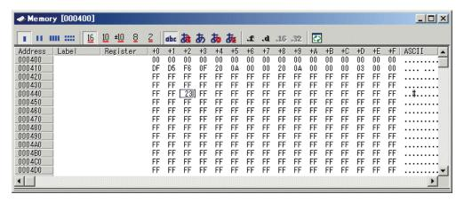
Placing the mouse cursor on a point in the display of data in the [Memory] window and double-clicking allows the values at that point to be changed.
