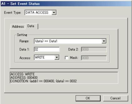
Example) Writing byte length data 32h to odd address 401h Contents of settings vary with each product and bus width. (8 bits bus width)
