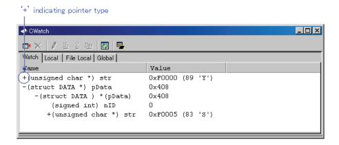
You can double-click on lines indicated by a '+' to see the members of that structure or union. The '+' changes to a '-' while the members are displayed. To return to the original display, double click the line, now indicated by the '-'.
