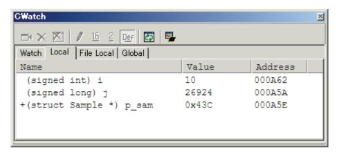
Double-click the mark '+' at the left side of pointer p\_sam in the [Locals] window to display the structure \*(p\_sam).
