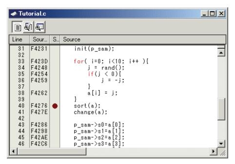
The red symbol will appear on the line containing the sort function call. This shows that a softwarebreak breakpoint has been set.
