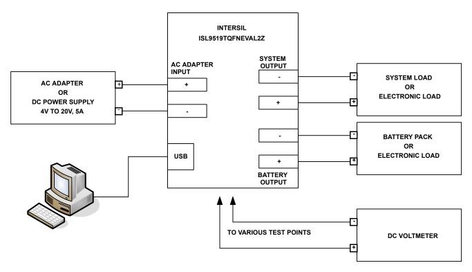
FIGURE 1. ISL9519TQFNEVAL2Z HARDWARE CONNECTION DIAGRAM
