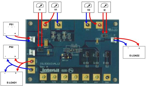
FIGURE 1. CONNECTION OF EQUIPMENT
