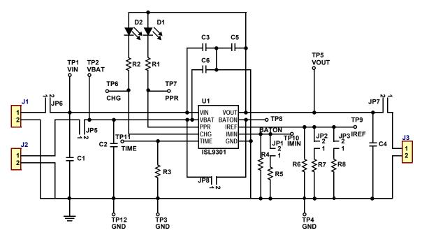
FIGURE 2. ISL9301EVAL1Z SCHEMATIC
