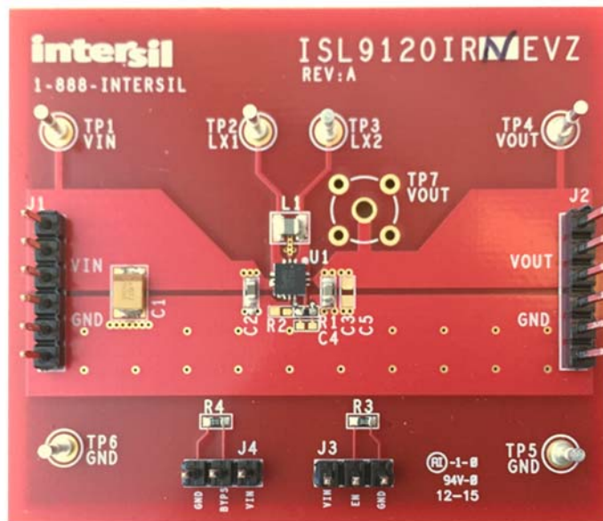
FIGURE 6. ISL9120IRN-EVZ EVALUATION BOARD
