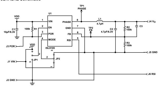
FIGURE 2. ISL9105EVAL1Z SCHEMATIC
