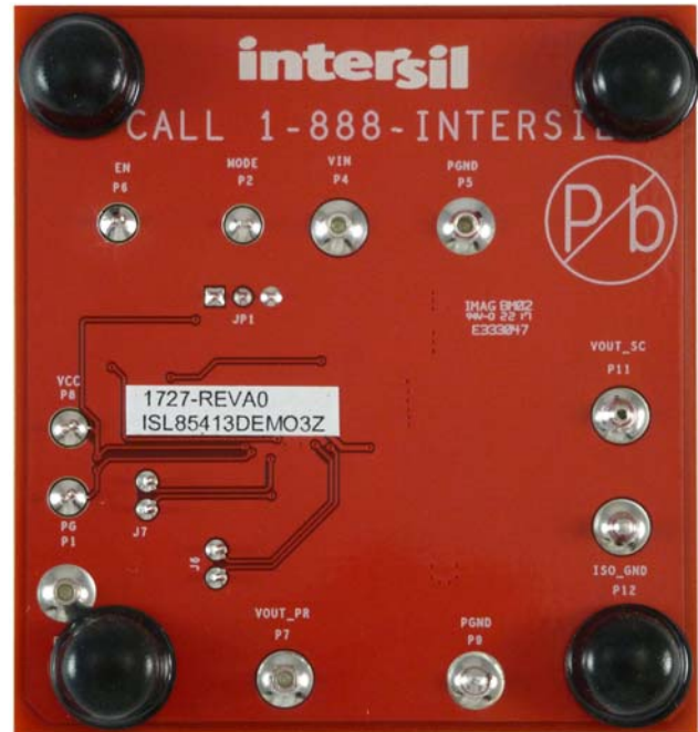
Figure 3. ISL85413DEMO3Z Evaluation Board Bottom View
