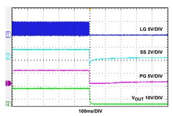
FIGURE 20. SHUT-DOWN WAVEFORMS,  $I_0 = 3A$
