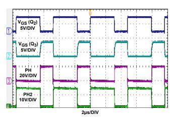
FIGURE 26. DRIVER SIGNAL OF  ${\rm Q_2,\,Q_3,\,PH}$  and PH2 waveforms;  ${\rm V_{IN}=24V,\,I_0=3A}$
