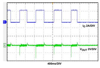
FIGURE 23. LOAD TRANSIENT,  $I_0 = 0A$  TO 3A
