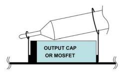
FIGURE 2. PROPER PROBE SETUP TO MEASURE OUTPUT RIPPLE
