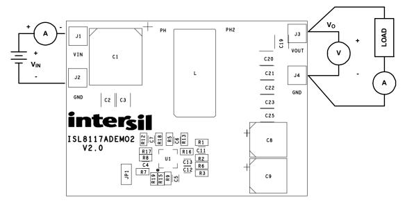
FIGURE 3. PROPER TEST SETUP
