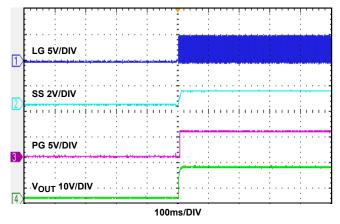
FIGURE 19. START-UP WAVEFORMS,  $I_0 = 3A$
