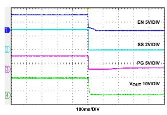
FIGURE 22. SHUT-DOWN WAVEFORMS,  $I_0 = 3A$
