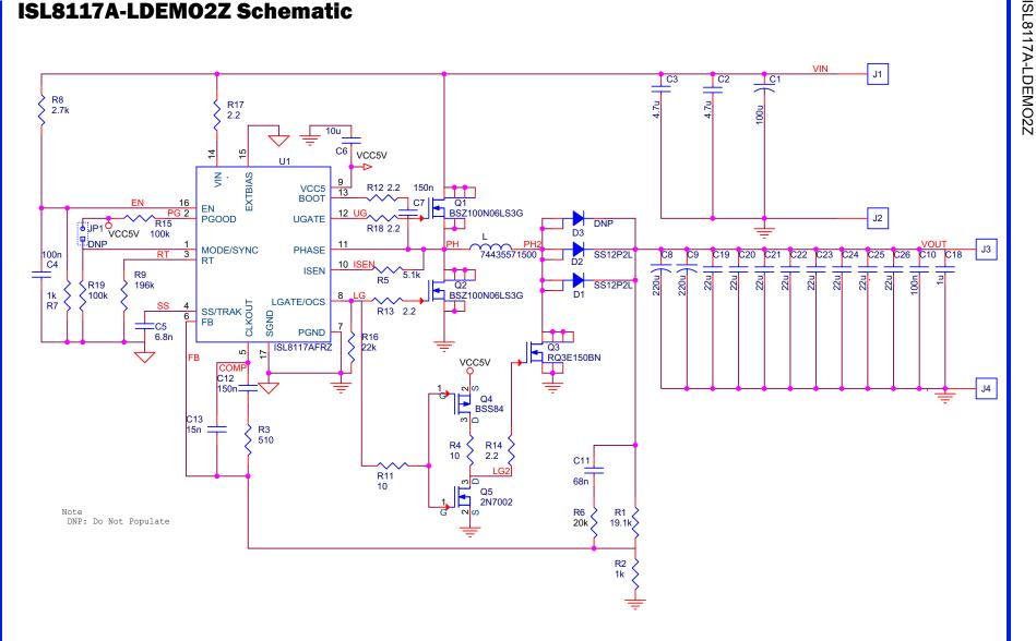
FIGURE 6. ISL8117A-LDEM02Z SCHEMATIC
