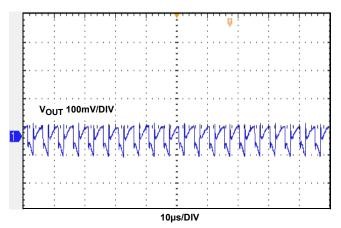
FIGURE 24. OUTPUT RIPPLE, I<sub>0</sub> = 3A
