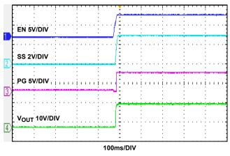
FIGURE 21. START-UP WAVEFORMS, I<sub>0</sub> = 3A
