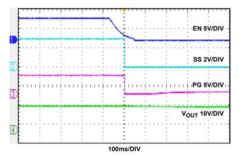
FIGURE 17. START-UP WAVEFORMS,  $I_0 = 0A$
