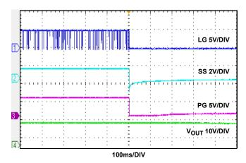
FIGURE 15. START-UP WAVEFORMS,  $I_0 = 0A$
