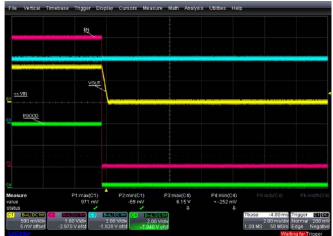
FIGURE 6. SHUTDOWN WAVEFORM: V_{IN} = 2.2V , V_{OUT} = 0.8V , EN HIGH TO LOW
