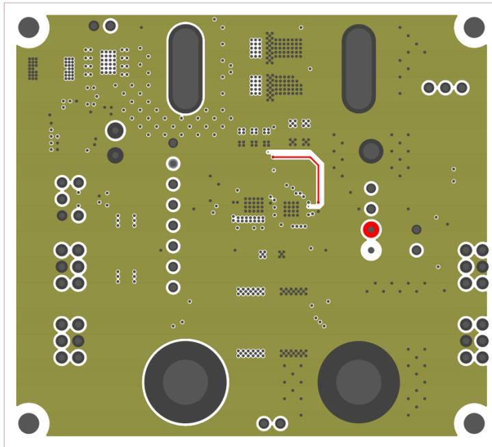
Figure 10. PCB - Inner Layer - Layer 2 (Top View)
