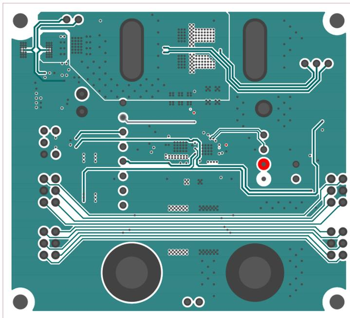
Figure 11. PCB - Inner Layer - Layer 3 (Top View)
