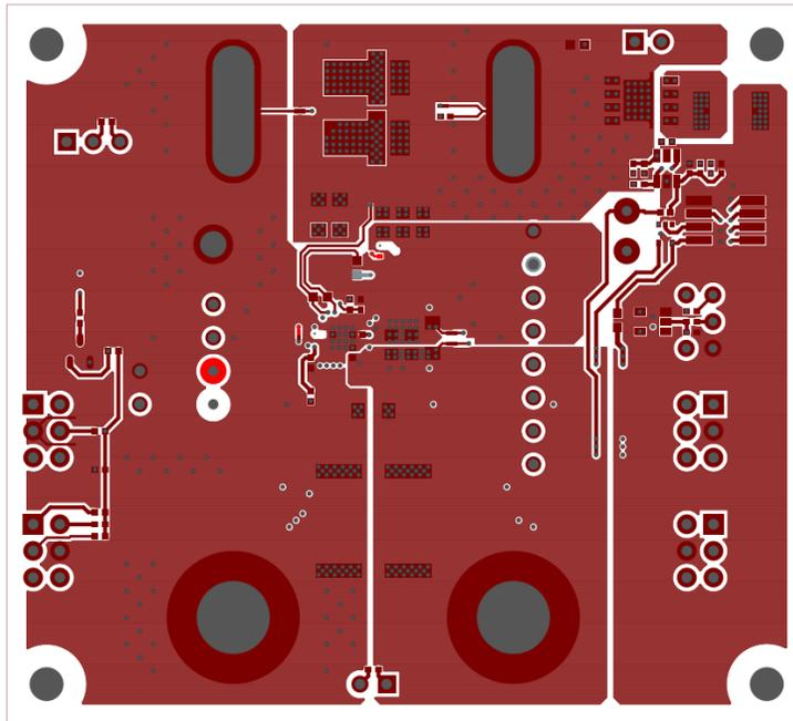
Figure 14. PCB - Bottom Layer (Top View)
