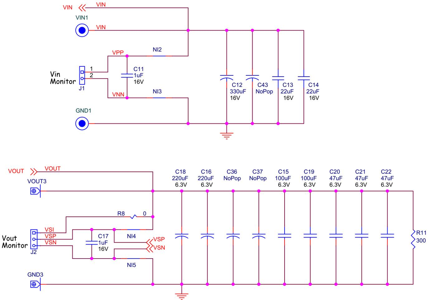
Figure 5. Schematic - Input and Output Filters
