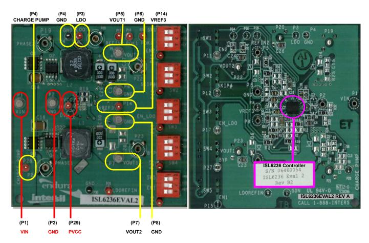
FIGURE 1. ISL6236EVAL2 REV B EVALUATION BOARD TOP AND BOTTOM VIEW
