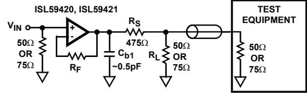
\* C<sub>b1</sub> is approximate PCB trace capacitance.
