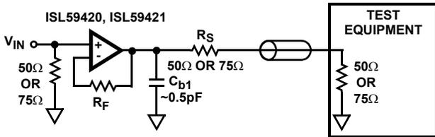
\* C<sub>b1</sub> is approximate PCB trace capacitance.
