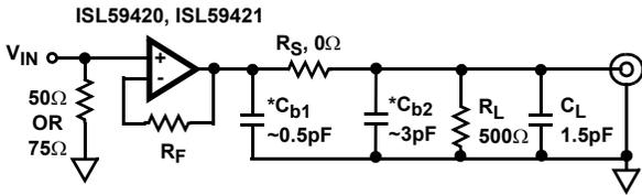
\* C<sub>b1</sub>, C<sub>b2</sub> are approximate PCB trace capacitances.
